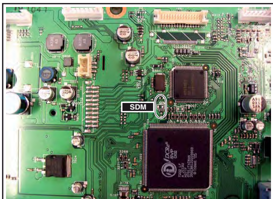
Figura 5-2 Service jumper (componentes SSB)
