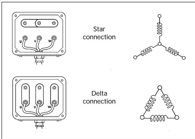
**On disconnected motors:** Measure U - U<sub>1</sub>, V - V<sub>1</sub>, W - W<sub>1</sub>. Compare readings with the **highest** of the inductance readings and check if it is within tolerances. Equal readings, or small differences within tolerance limits, indicate that both stator and rotor are in good condition. If the motor condition is very suspect, turn the rotor approx. 90° and repeat the measurement.
