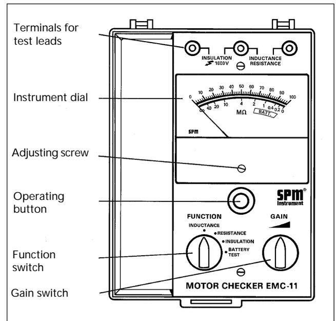
Large differences in inductance only, are probably caused by an inter-turn short circuit in a stator winding. As the damage spreads, it will also affect resistance readings. A rotor fault will affect the inductance of the stator windings as the rotor position is changed.
