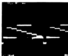
IC303 Pin 10 PB MODE 1H DELAY OUTPUT SIGNAL
