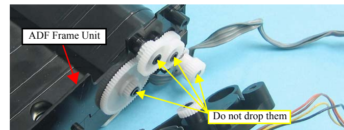
Figure 4-144. Handling the ADF Motor Unit
