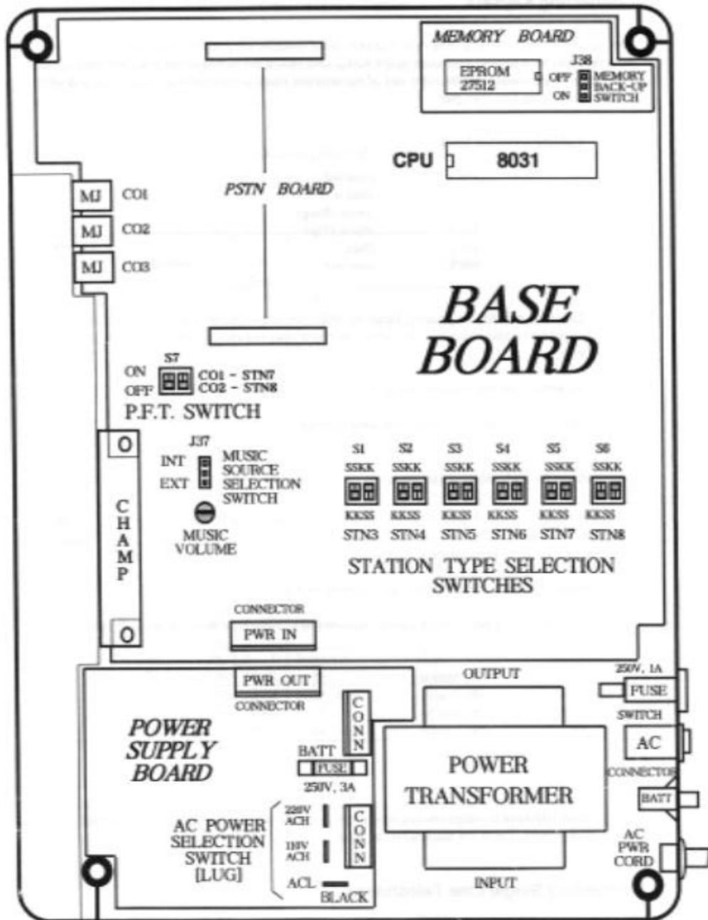
Figure 4 - Base Board Switch Locations
