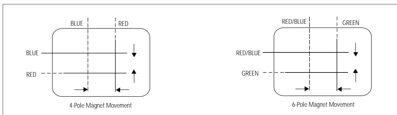
Fig. 3-3 Center Convergence Adjustment
