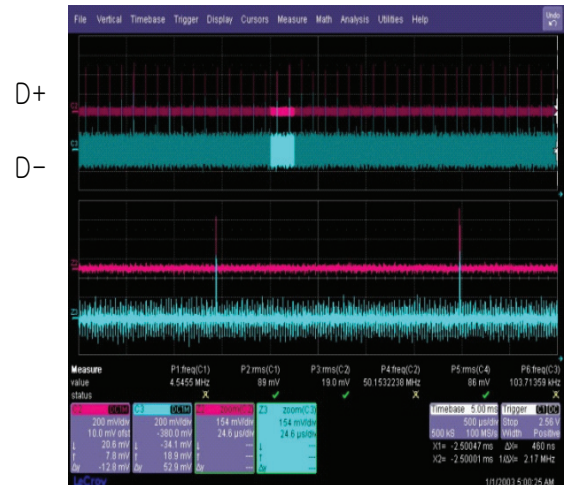
< Waveform of USB D \pm signal > USB D+ / D- (CN502 Pin1, 2 & 9, 10)
