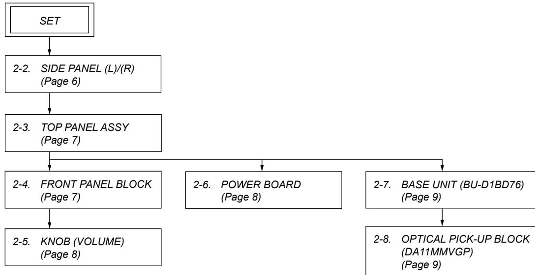
**Note:** Follow the disassembly procedure in the numerical order given.
