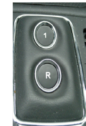
Push buttons replace the T-lever for driving direction selection
