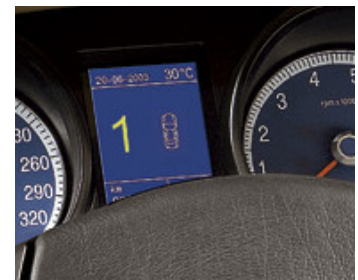
Gear and driving mode visualisation on central display
