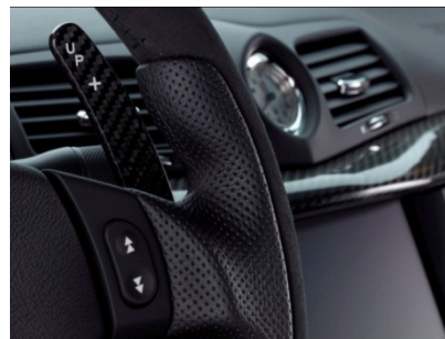
Longer gearshift paddles permit easy shifting during cornering
