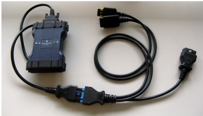
VCI with 4-way adapter cable for older vehicles
