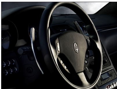
Longer gearshift paddles permit easy shifting during cornering
