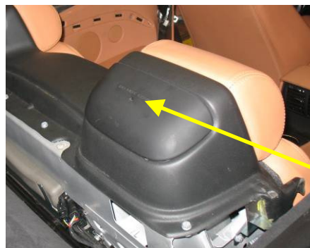
The tungsten pin concealed underneath the plastic breaks the rear window during roll bar activation.
