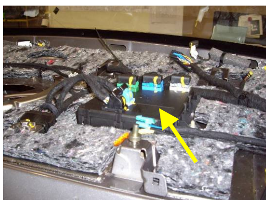
The NVB is located underneath the rear parcel shelf
