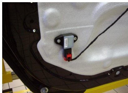
Lateral pressure sensor for advanced impact warning
