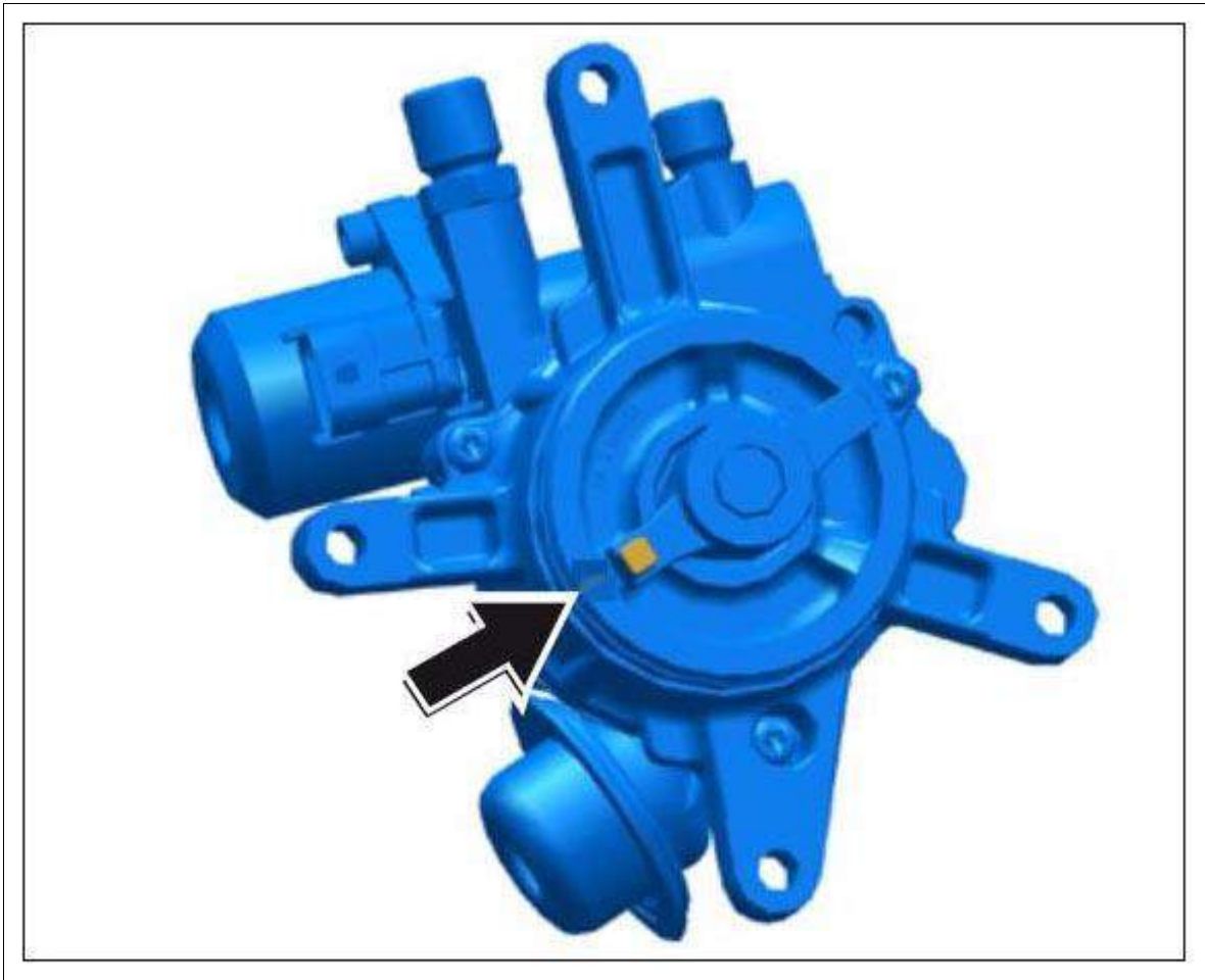
Fig 1: Locating Mark Rotor Position
