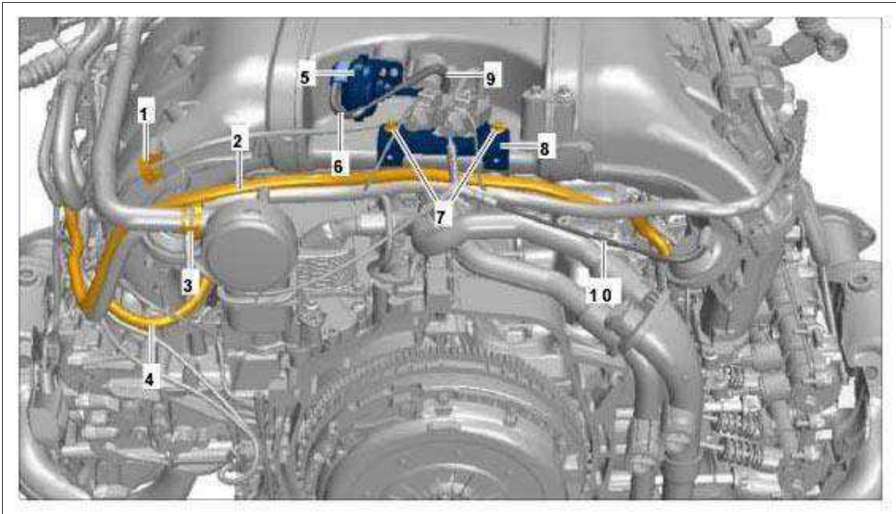
Fig 1: Overview Of Line And Cable Routing On Front Intake-Air Distributor
