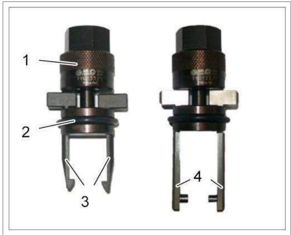
Fig 5: Identifying Fuel Injector Holder (Puller Arms)
