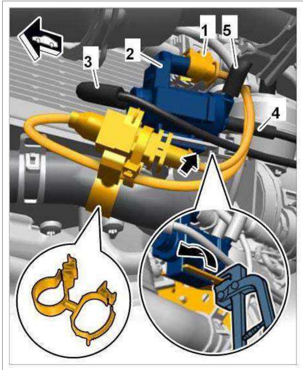
Fig 9: Locating Change-Over Valve For Shut-Off Valve For Gear Wheel Set Heat Exchanger
