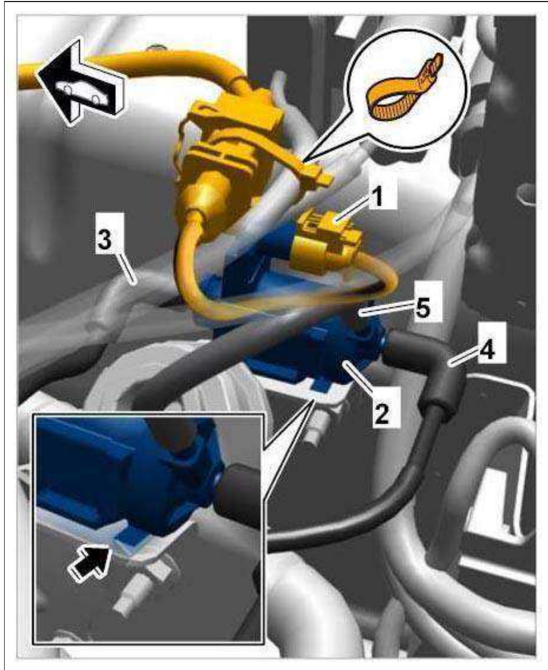
Fig 5: Locating Change-Over Valve For Heat Exchanger
