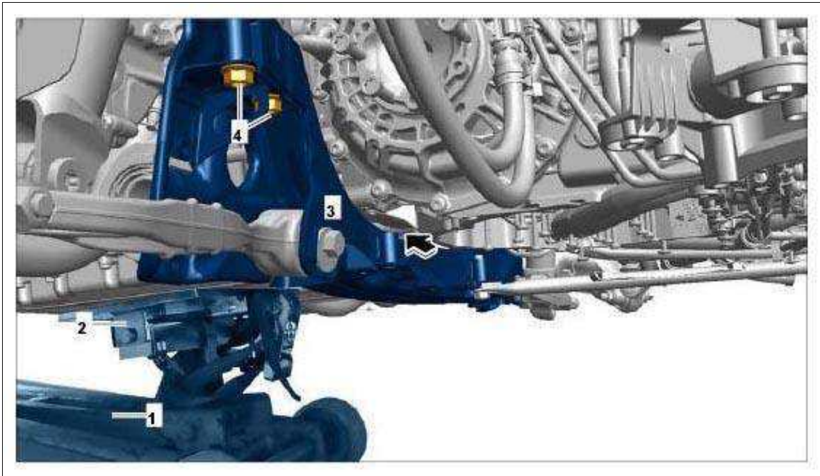
Fig 4: Supporting Engine Using Jack
