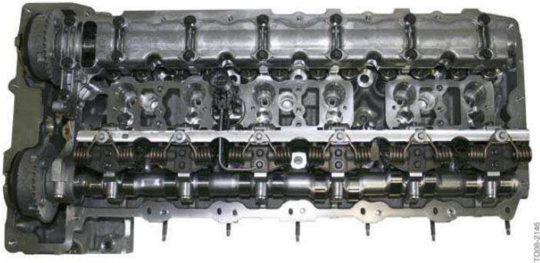
Fig. 19: Identifying Cylinder Head - N55 Courtesy of BMW OF NORTH AMERICA, INC.
