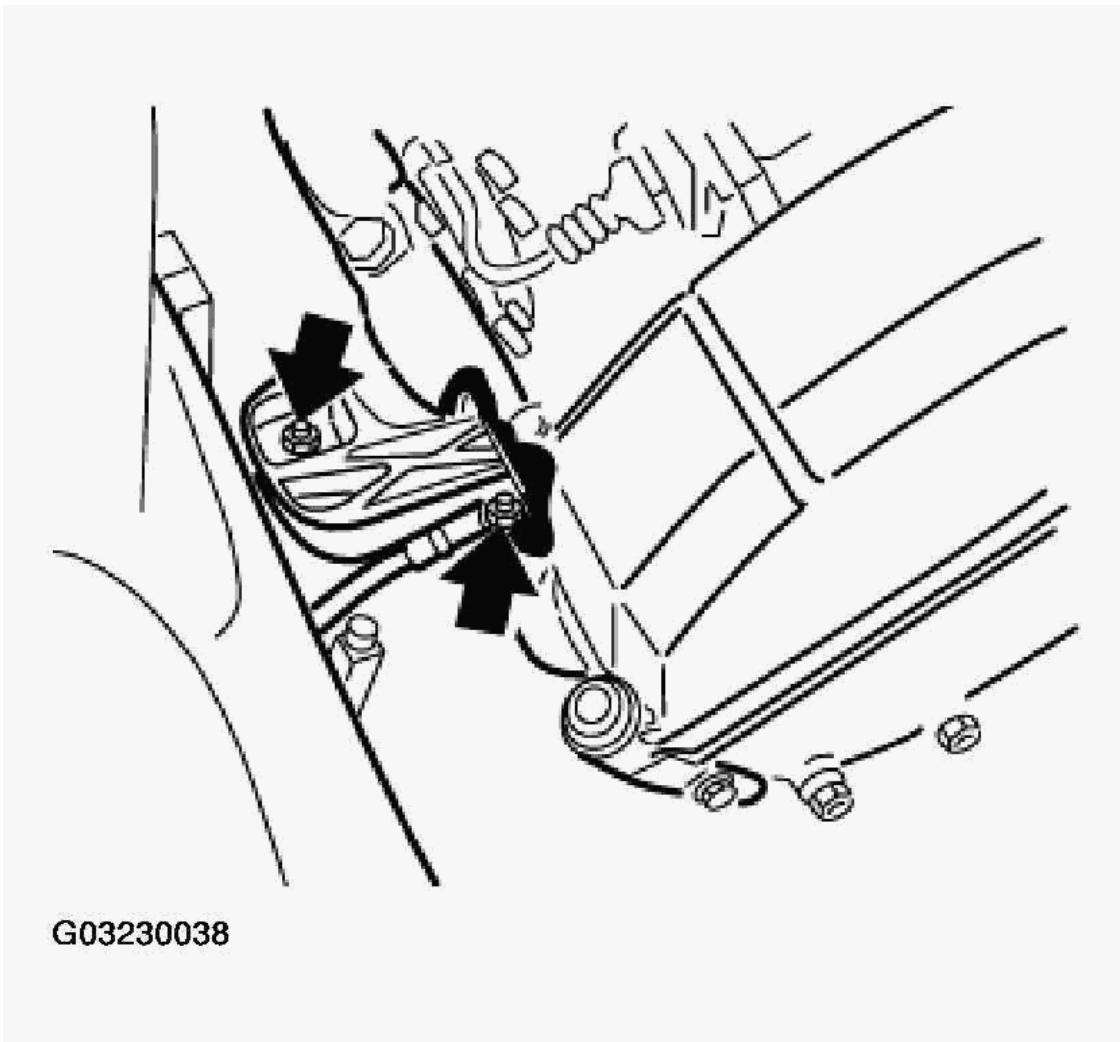
Fig. 12: Locating Right Engine Mount And Ground Wire Courtesy of BMW OF NORTH AMERICA, INC.
