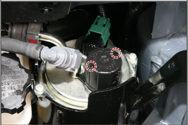
Holes on priming pump cap
