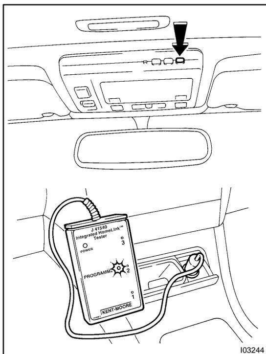
(b) Press the switch which an inspection code has been registered for and check that LED (green) of the home link tester lights up.
