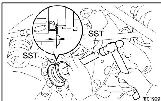
6. INSTALL SIDE GEAR SHAFT OIL SEAL
