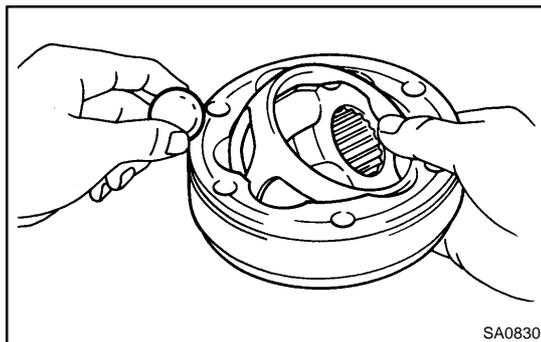
(b) Tilt the cage and inner race to the side and insert the balls one by one.
