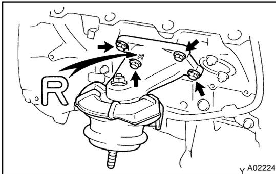
**27. INSTALL RH ENGINE MOUNTING BRACKET**
