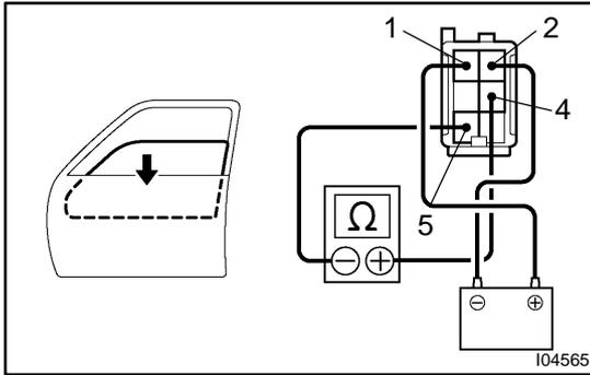
**19. Driver's Door (Window Down):****INSPECT JAM PROTECTION LIMIT SWITCH**
