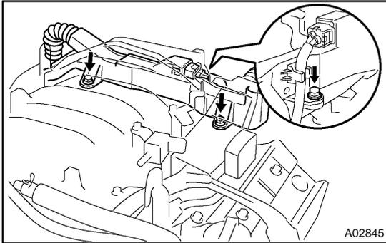
(2) Remove the 3 bolts, and disconnect the engine wire protector from the rear water bypass joint and RH cylinder head.
