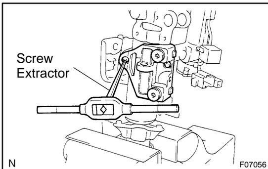
**13. REMOVE COLUMN UPPER BRACKET AND COLUMN UPPER CLAMP**
