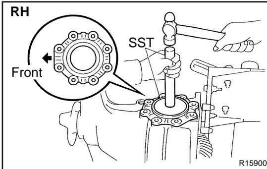
**12. INSTALL DIFFERENTIAL CARRIER RETAINERS**
