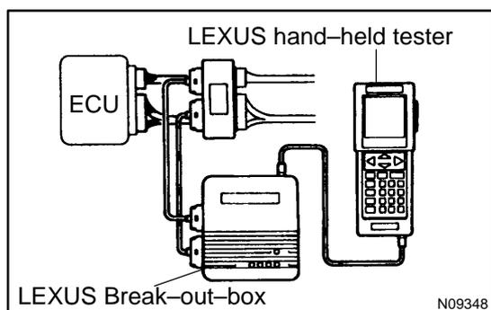
**8. ECU TERMINAL VALUES MEASUREMENT BY USING LEXUS BREAK-OUT-BOX AND LEXUS HAND-HELD TESTER**
