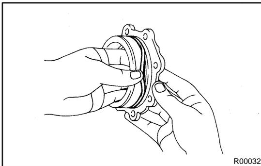
**27. INSTALL O-RING FROM DIFFERENTIAL CARRIER RETAINERS**
