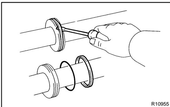
**3. IF NECESSARY, REPLACE TEFLON RING AND O-RING**
