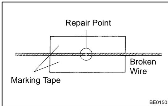
**7. IF NECESSARY, REPAIR DEFOGGER WIRE**
