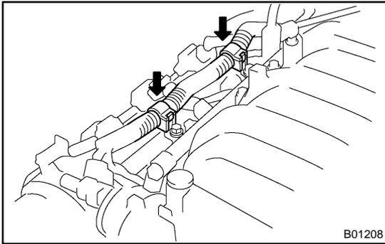
(w) Disconnect the engine wire from the RH delivery pipe, rear water bypass joint, intake manifold and cylinder head.
