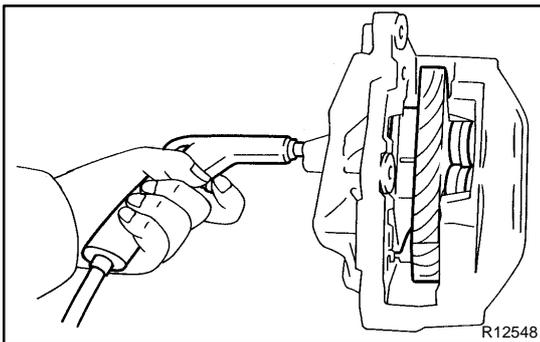
(b) Place the plate between the pistons and insert a pad on one side.
