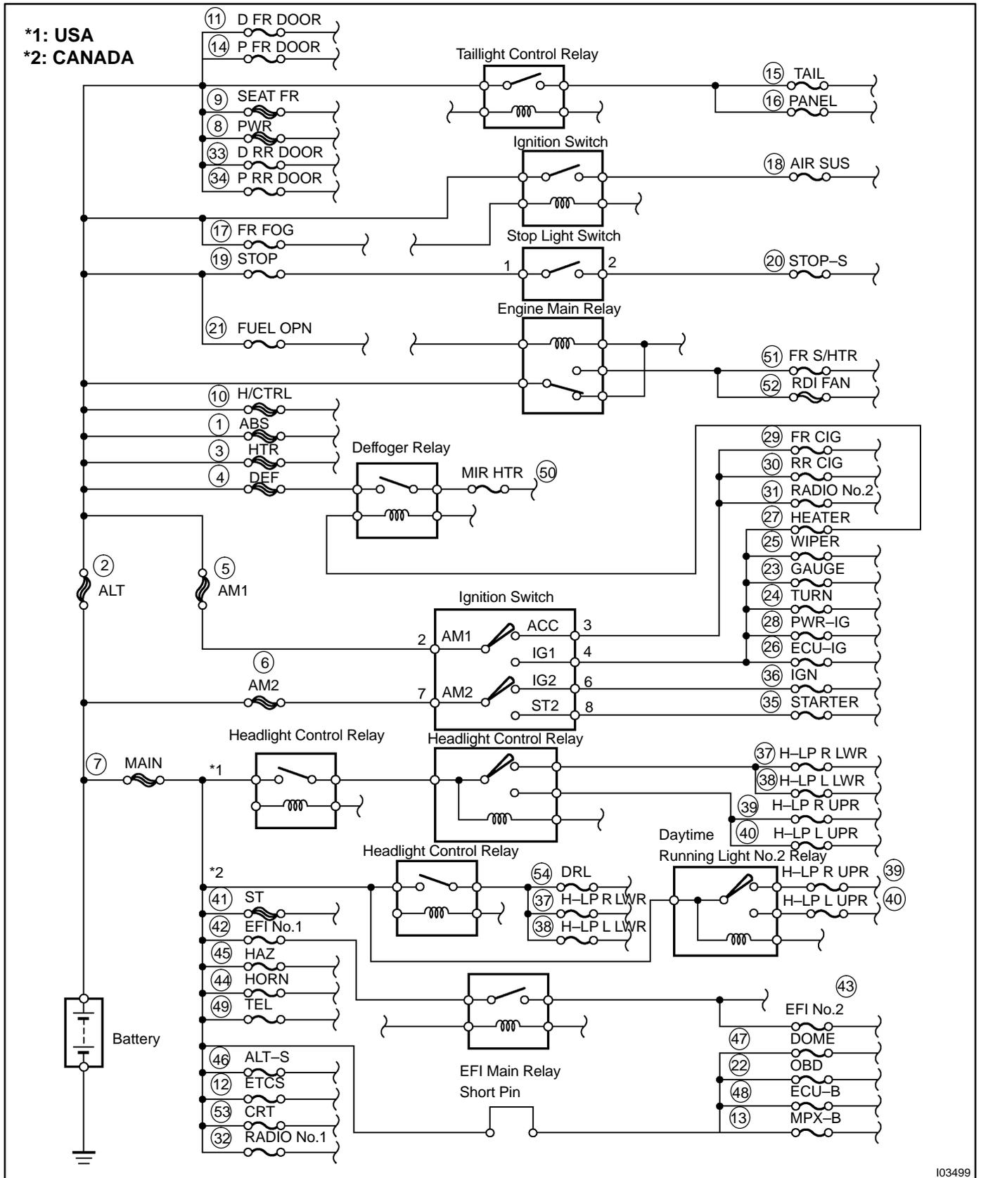
The power source supplies power to each of the vehicle's electrical devices. It is composed of the battery, fuses and relays, which are located centrally at engine room junction block, engine room No.1 relay block, fusible link block and engine room No.2 relay block in the engine compartment, and instrument panel junction block in the cabin near the driver's feet.
