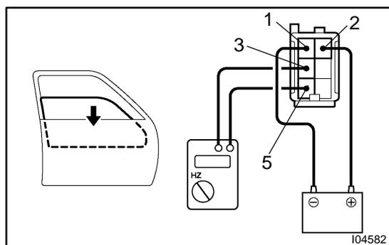
(d) Reverse the polarity and check that pulse is generated. If operation is not as specified, replace the motor.
