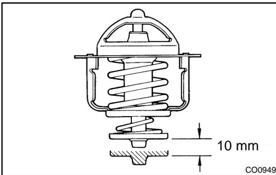
(c) Check the valve lift.
