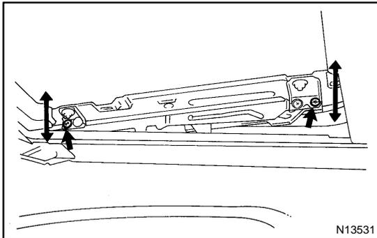
**2. ADJUST SLIDING ROOF GLASS LEVEL DIFFERENCE**
