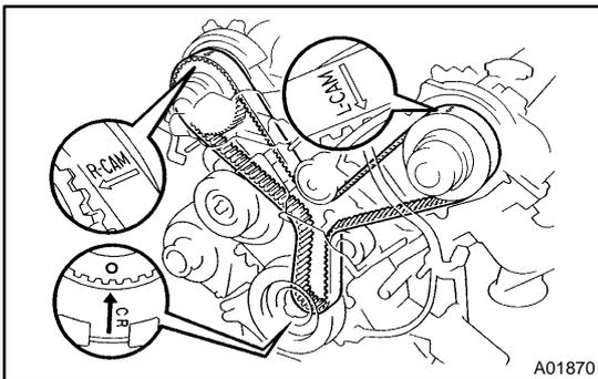
**16. IF RE-USING TIMING BELT, CHECK INSTALLATION MARKS ON TIMING BELT**
