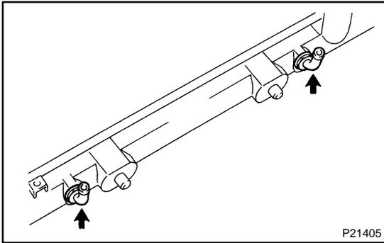
**7. REMOVE OIL COOLER FROM LOWER TANK**
