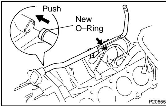
**26. INSTALL WATER BYPASS PIPE**
