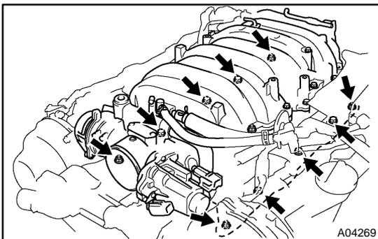
(x) Remove the 6 bolts, 4 nuts, intake manifold assembly and 2 gaskets.
