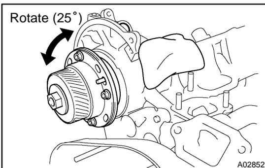
**(b) Rotate the VVT-i pulley from left to right 2 to 3 times within**
