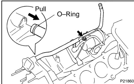
6. **REMOVE WATER BYPASS PIPE**
