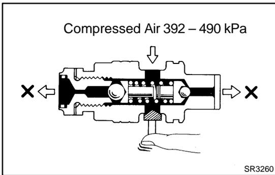
(b) Check the flow control valve for leakage. Close one of the holes and apply compressed air of 392 - 490 kPa (4 - 5 kgf/cm<sup>2</sup>, 57 - 71 psi) into the opposite side hole, and confirm that air does not come out from the end holes.
