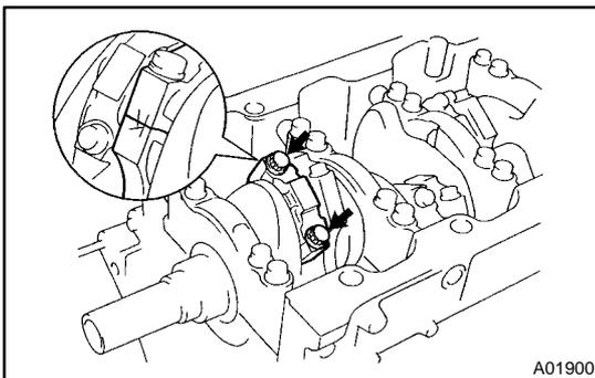
**20. REMOVE CONNECTING ROD CAPS AND CHECK OIL CLEARANCE**
