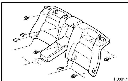
(c) Remove the 7 bolts, then raise the seatback assembly upward to remove the seatback assembly.
