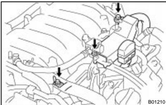
(3) Remove the 3 bolts, and disconnect the engine wire protector and wire clamp bracket from the intake manifold.
