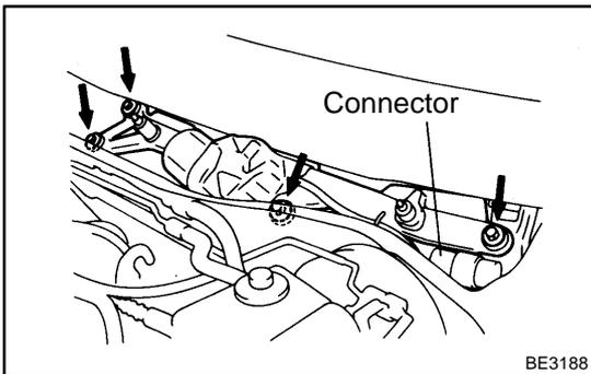
3. REMOVE WIPER MOTOR AND LINK ASSEMBLY
