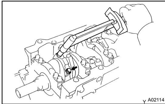
(g) Install the connecting rod cap with the 2 bolts.
