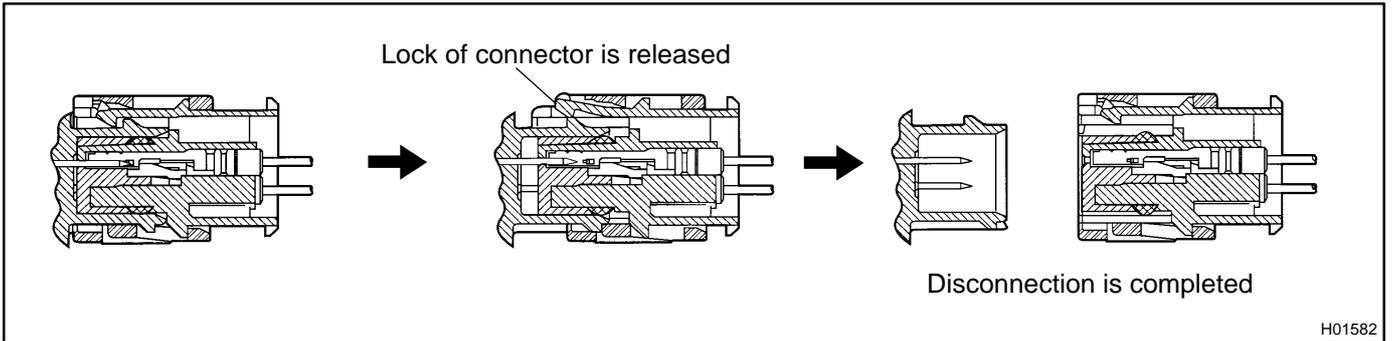
**11. CONNECTION OF SIDE AIRBAG SENSOR CONNECTOR**
