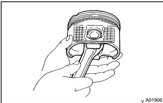
**24. CHECK FIT BETWEEN PISTON AND PISTON PIN**
