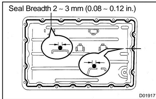
(b) Remove any packing material and be careful not to drop oil on the contacting surfaces of the transmission case and oil pan.
