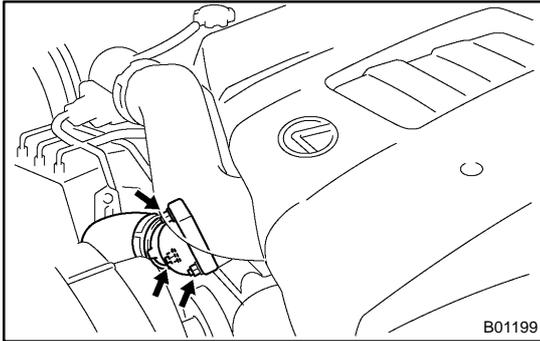
3. **DISCONNECT WATER INLET FROM WATER INLET HOUSING**
