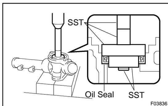
(c) Coat a new oil seal lip with power steering fluid.
