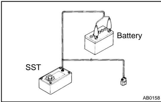
**1. AIRBAG DEPLOYMENT WHEN SCRAPPING VE-
