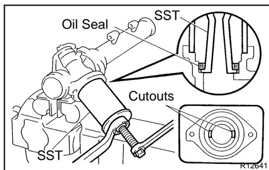
(b) Using SST, remove the oil seal from the rack housing.
