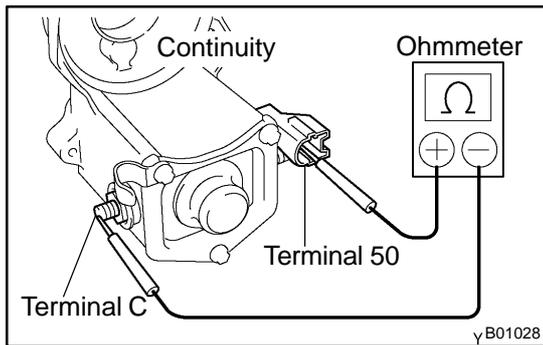
**16. DO PULL-IN COIL OPEN CIRCUIT TEST**
