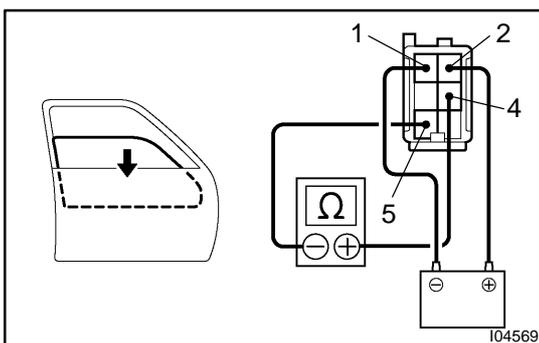
**21. Front Passenger's Door (Window Down):****INSPECT JAM PROTECTION LIMIT SWITCH**
