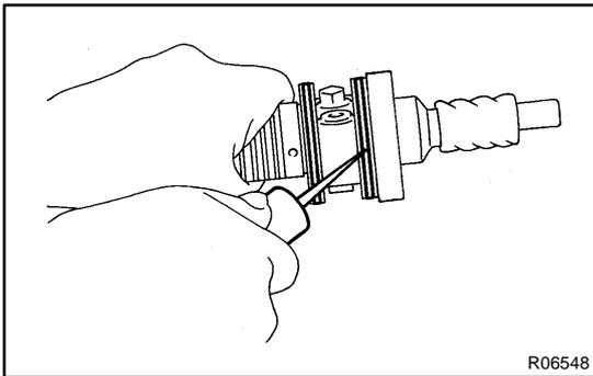
**5. IF NECESSARY, REPLACE TEFLON RINGS AND O-RINGS**
