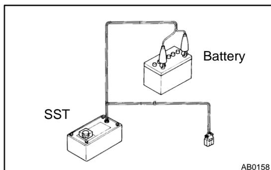
(1) Connect the SST to the battery.
