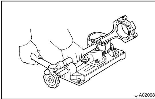
(c) Using a plastic-faced hammer and brass bar, lightly tap out the piston pin and pin and remove the connecting rod.
