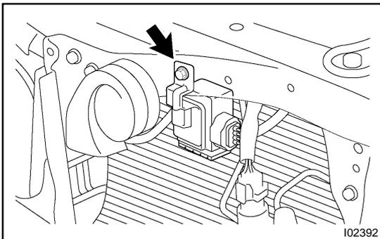
**6. REMOVE SMOG VENTILATION SENSOR**
