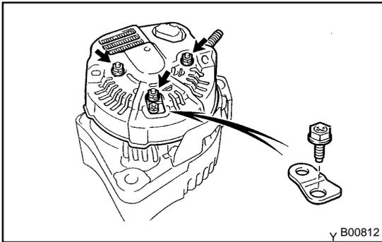
(b) Remove the 3 nuts, bolt, plate terminal and rear end cover.
