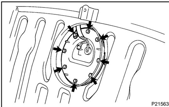
6. REMOVE FUEL PUMP, BRACKET AND SET PLATE ASSEMBLY
