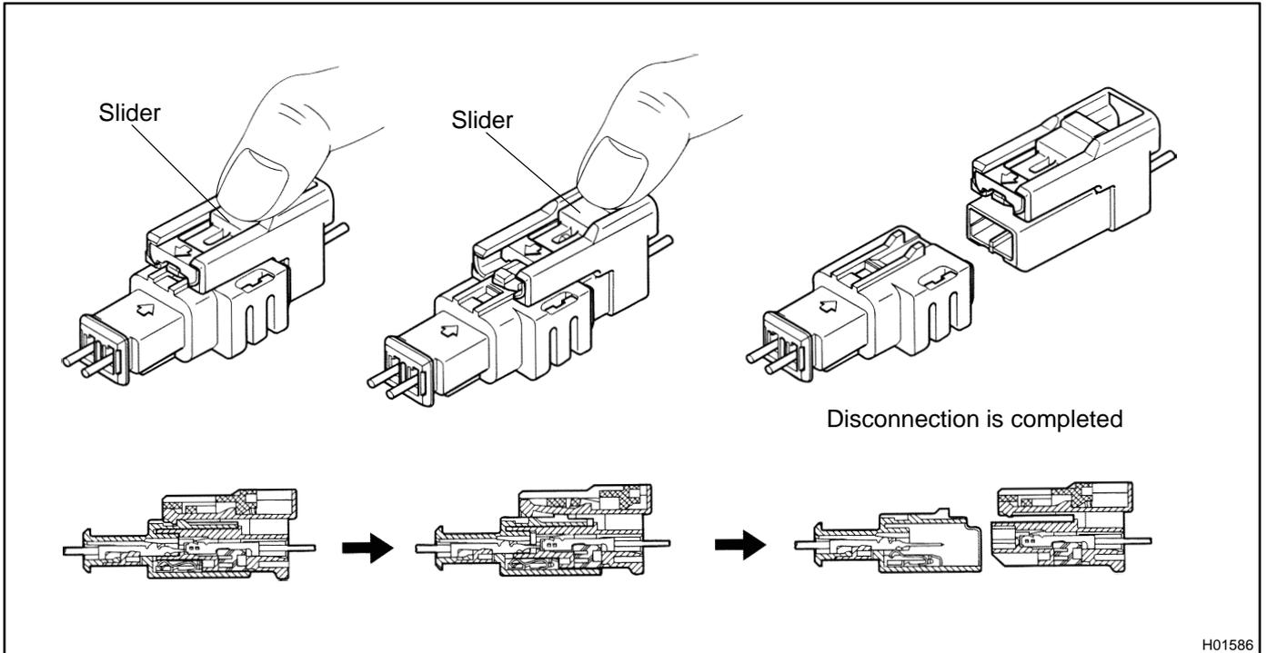
**15. CONNECTION OF CONNECTORS FOR STEERING WHEEL PAD (with AIRBAG) AND FRONT PASSENGER AIRBAG ASSEMBLY**
