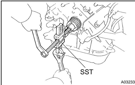
**31. REMOVE CRANKSHAFT TIMING PULLEY**
