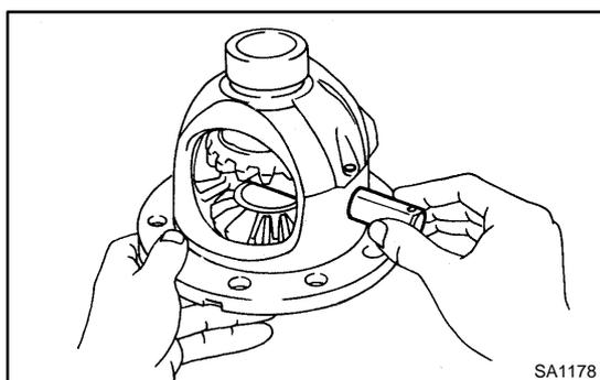
(b) Install the 2 side gears, pinion gears, pinion gear thrust washers and pinion shaft in the differential case.
