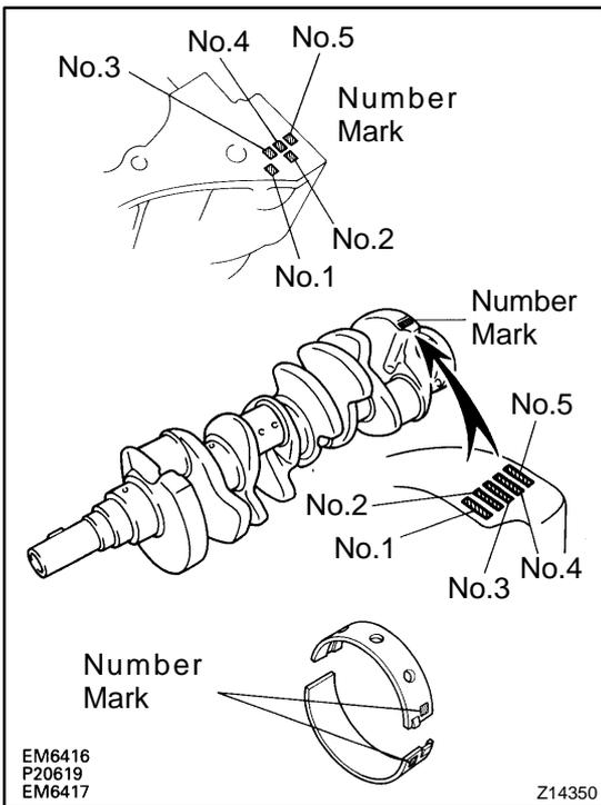
If the oil clearance is greater than maximum, replace the bearings. If necessary, replace the crankshaft.
