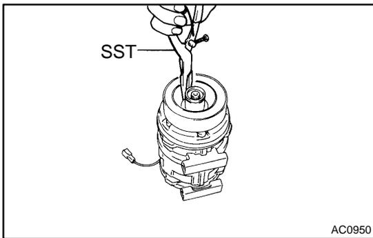
(b) Using SST, remove the snap ring.
