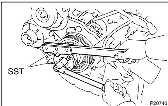
**17. LOOSEN CRANKSHAFT PULLEY BOLT**
