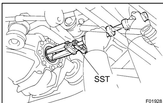
5. REMOVE SIDE GEAR SHAFT OIL SEAL
