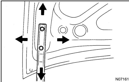
(b) For forward/rearward and left/right adjustment, loosen the bolts.
