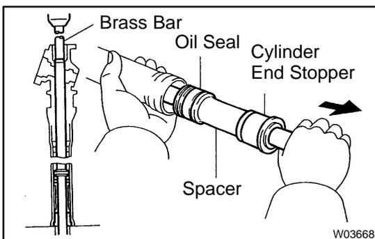
**15. REMOVE CYLINDER END STOPPER, SPACER, OIL SEAL AND STEERING RACK**
