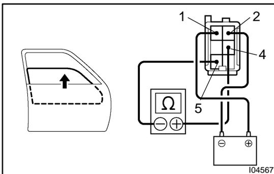
**20. Front Passenger's Door (Window Up):****INSPECT JAM PROTECTION LIMIT SWITCH**
