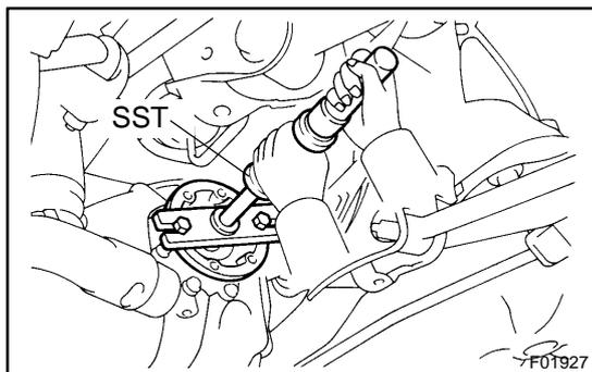
4. REMOVE SIDE GEAR SHAFT
