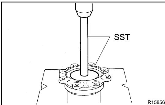
**28. INSTALL OIL SEALS FROM DIFFERENTIAL CARRIER RETAINERS**
