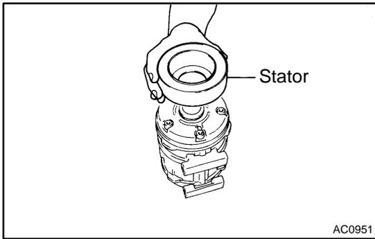
(c) Remove the stator.
