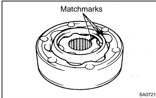
(a) Align the matchmarks placed before removal.
