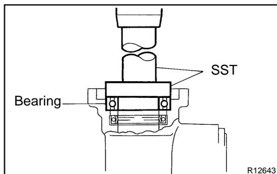
(e) Using SST, press in a new bearing.
