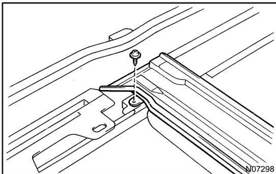
3. REMOVE ROOF DRIP CHANNEL
