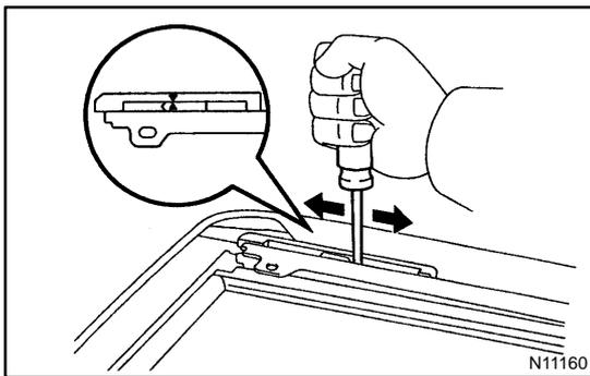
(b) When the front or rear alignment is not correct, remove the glass and adjust the drive rail.
