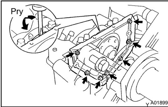
**18. REMOVE REAR OIL SEAL RETAINER**
