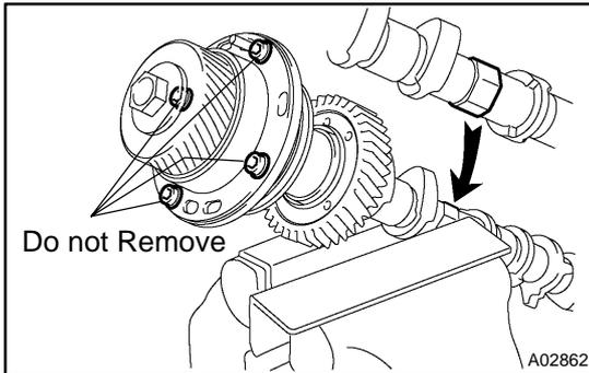
**23. REMOVE CAM SHAFT TIMING TUBES**
