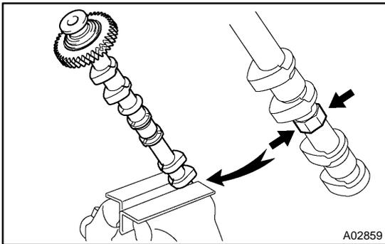
**22. DISASSEMBLE EXHAUST CAMSHAFTS**
