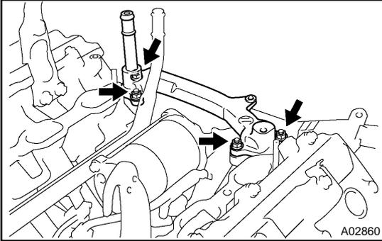
**13. REMOVE REAR WATER BYPASS JOINT**
