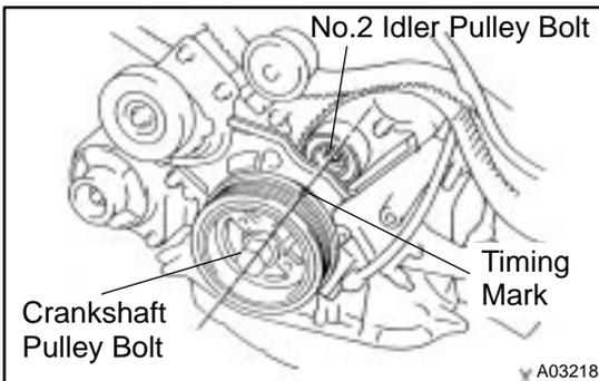
**(a) Check the crankshaft pulley position.**
