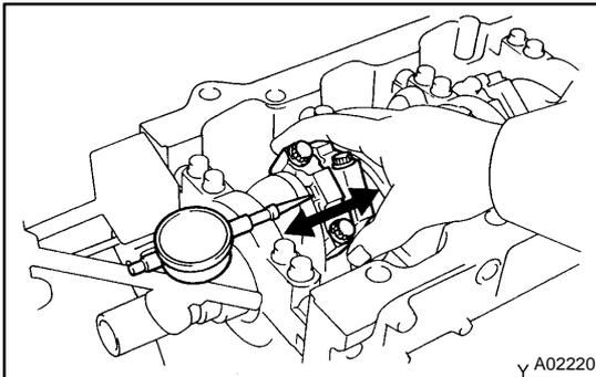
**19. CHECK CONNECTING ROD THRUST CLEARANCE**
