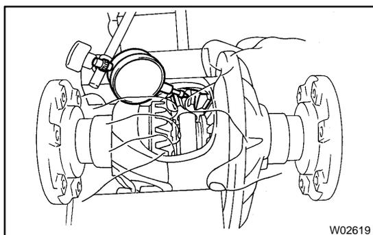
(d) Using a dial indicator, measure the pinion gear backlash with holding one side gear toward the case.
