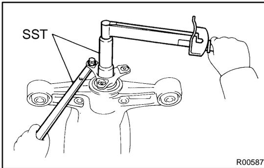
If the preload is greater than the specification, replace the spacer.
