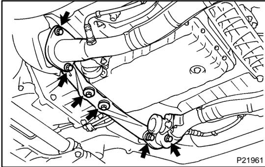
5. DISCONNECT FRONT EXHAUST PIPE FROM TWC
