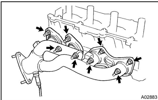
**26. REMOVE RH EXHAUST MANIFOLD FROM CYLINDER HEAD**
