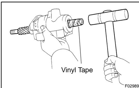
**13. REMOVE CONTROL VALVE ASSEMBLY**
