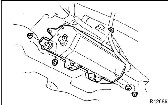
5. REMOVE FRONT PASSENGER AIRBAG ASSEMBLY
