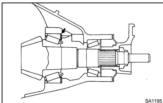
If tooth contact pattern is not correct, replace the adjusting washer installed on the front of the drive pinion rear bearing to adjust it.
