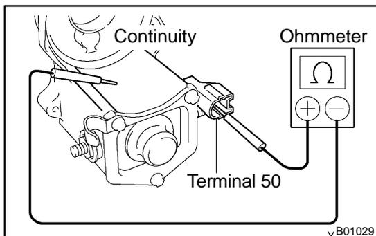
**17. DO HOLD-IN COIL OPEN CIRCUIT TEST**
