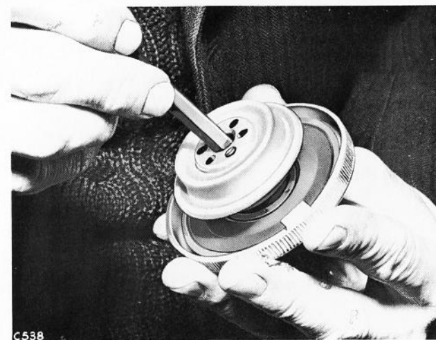
Fig.15 Checking Radiator Pressure release and Overflow Valve
