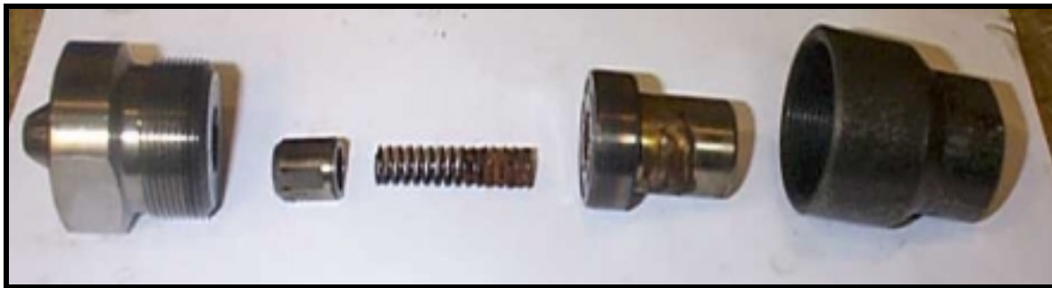
Fig. 79 FLOW-LIMITER VALVE DISASSEMBLED
