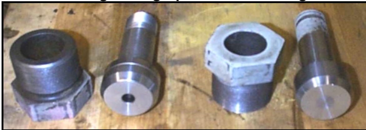
Fig. 54 High-pressure Rail Plug
