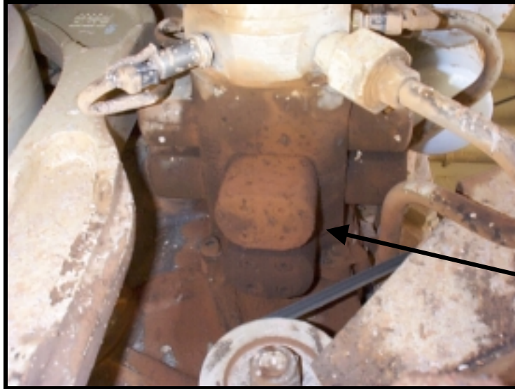
Fig. 21 High-pressure Fuel Pump Leak at Weep hole.
