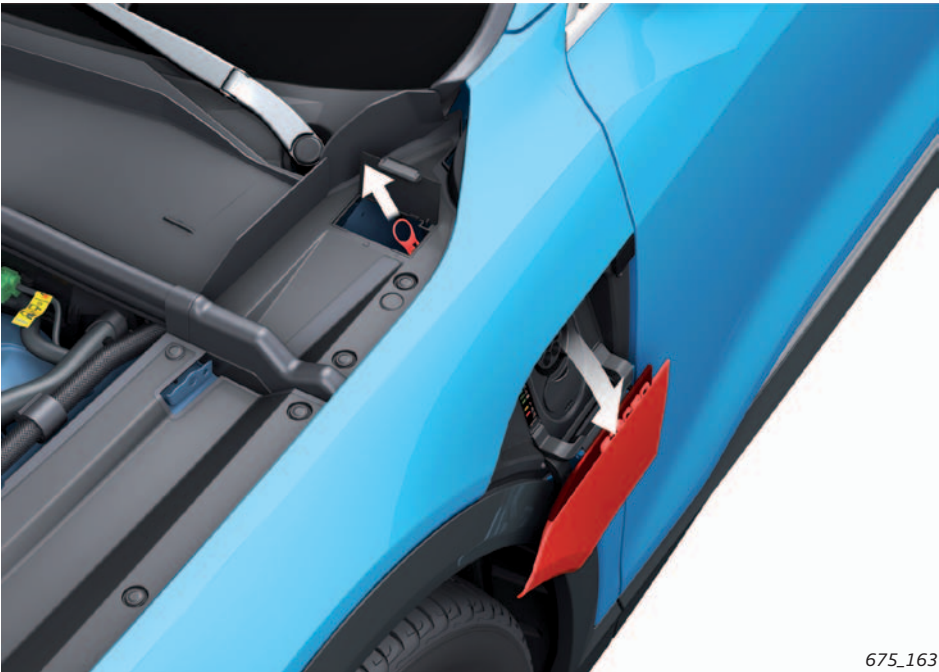
Charging flap manual release
