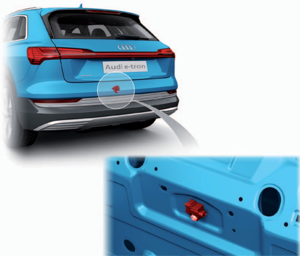
Crash sensor for rear-end collision G572
