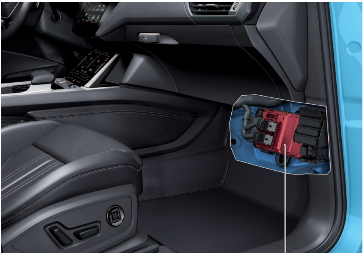
Onboard supply control unit J519
