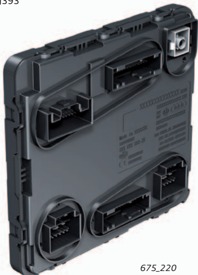
Convenience system central control unit J393
