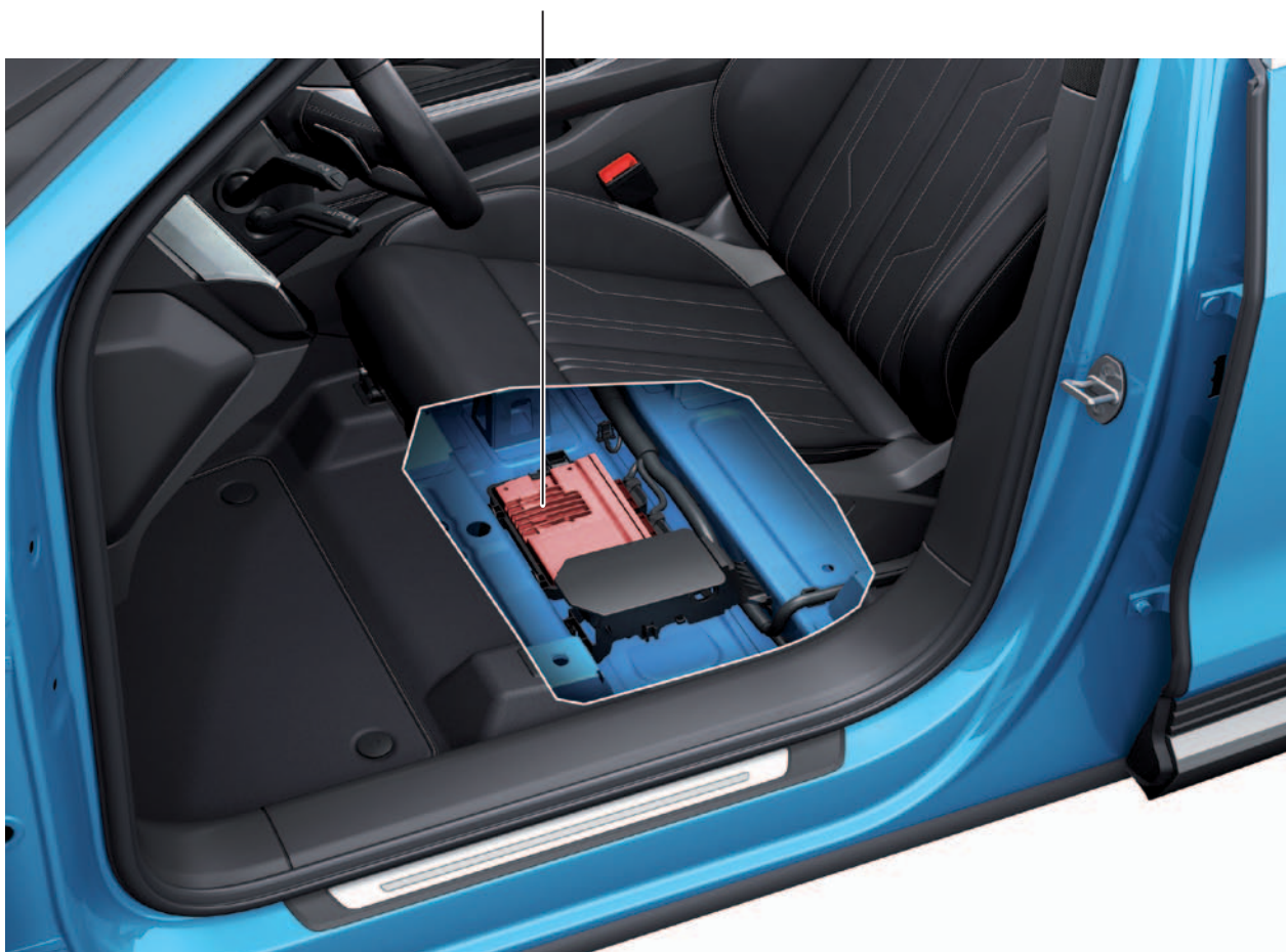
Data bus diagnostic interface J533
