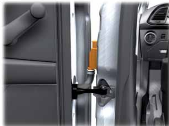
Rear door coupling stations (connectors)
