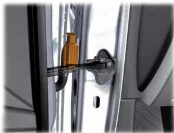
Front door coupling stations (connectors)
