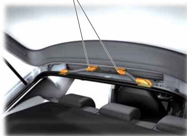
Tailgate coupling stations (connectors)
