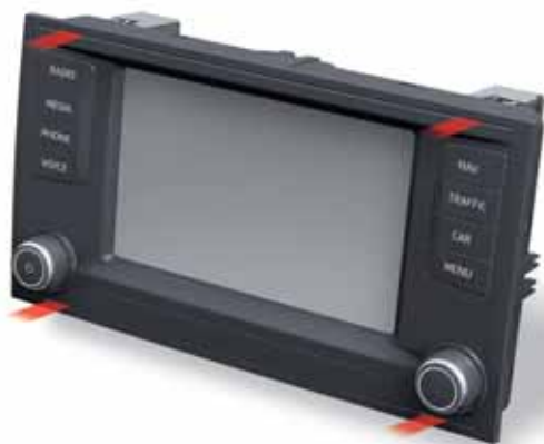
Slots to set the T10057 removal tools
