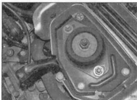
9.22 Remove the transmission mounting – AL4 transmission
