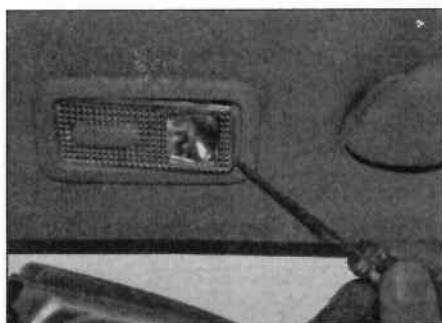
6.2a Unclip the interior side light unit ...
