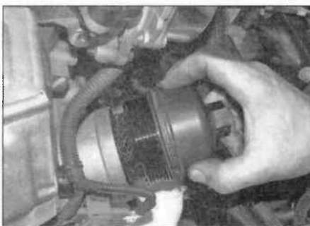
3.8b ... and unscrew the filter plastic cover
