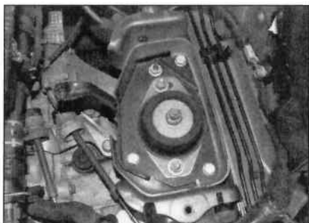
7.21 Remove the transmission mounting – MCM and BVM6 transmissions
