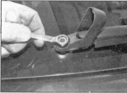
13.7 Lift up the trim cover and undo the wiper arm spindle nut
