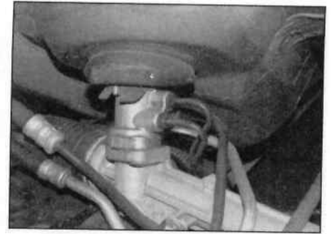
19.8 Undo the fluid pipes unions
