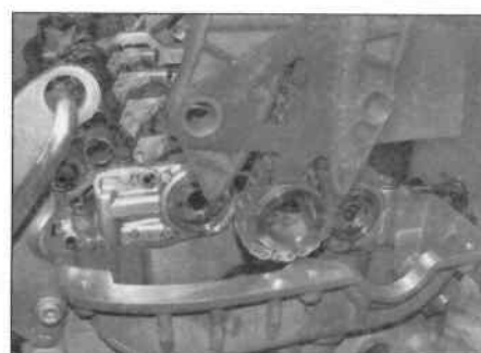
6.17b ... complete with crankshaft sprocket
