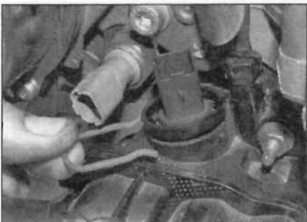
7.6a Prise out the sensor securing clip ...
