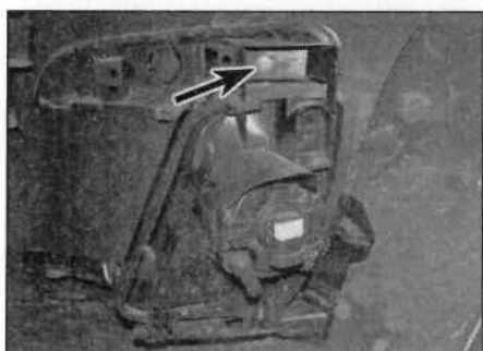
7.38a Undo the upper mounting screw (arrowed) ...
