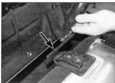
23.7 Unclip the hinge pin (arrowed)
