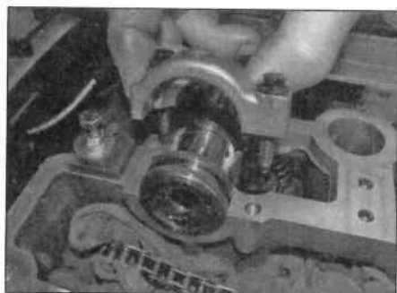
7.14a Remove the camshaft bearing caps ...
