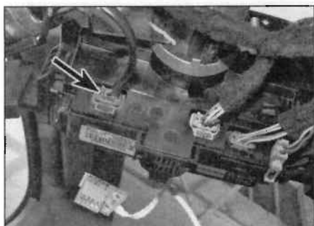
18.3 Disconnect the transponder wiring connector (arrowed)
