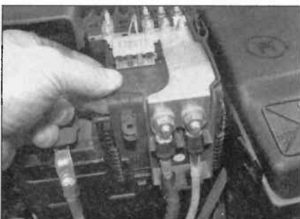
4.6c ... then slide the fused link assembly upwards
