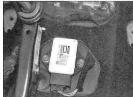
22.21 Gyrometer/accelerometer sensor
