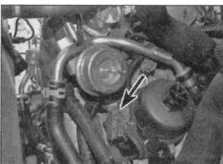
21.15 Disconnect the wiring plug connector (arrowed)
