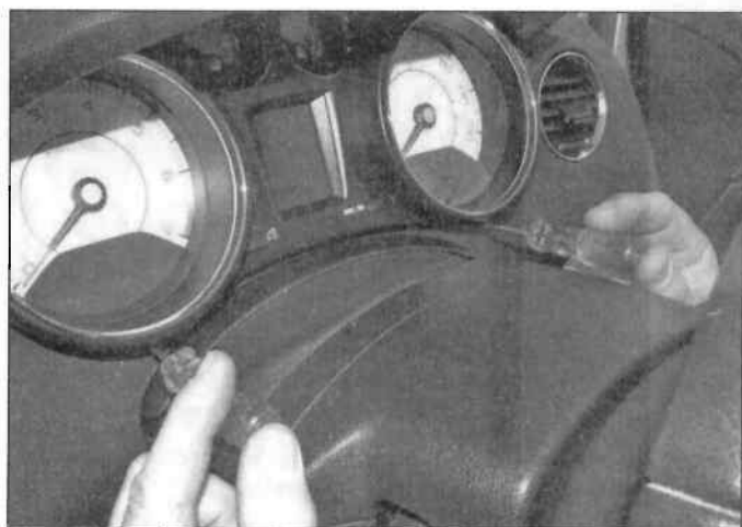
9.3a Insert two thin screwdrivers/pins ...
