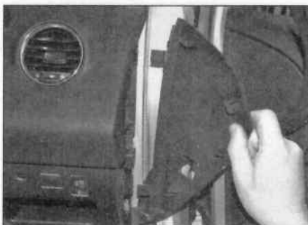
4.24 Unclip the trim from the side of the fascia
