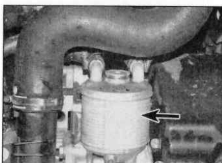
7.3 Fluid cooler (arrowed) – AT6 transmission
