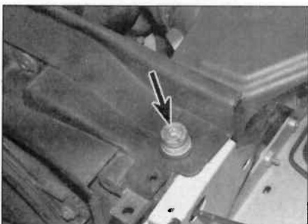
20.6 Undo the front panel outer retaining bolts (one side arrowed)
