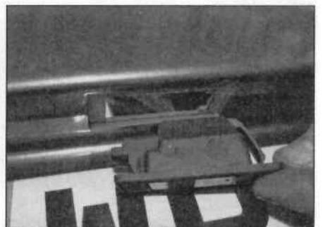
7.30b ... and remove the light unit from the bumper
