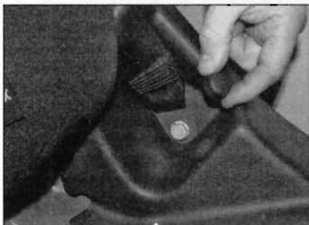
24.10 Undo the seat belt lower anchor bolt
