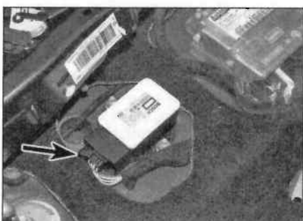
19.33 Release the clip (arrowed) and disconnect the sensor wiring plug
