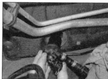
3.6 Turn the master cylinder 45° clockwise, and remove it from the bulkhead
