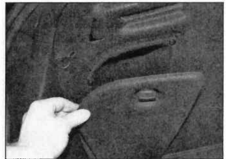
7.12a Remove the compartment cover ...
