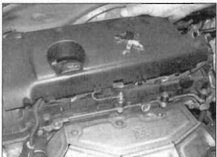
4.3 Remove the cylinder head cover
