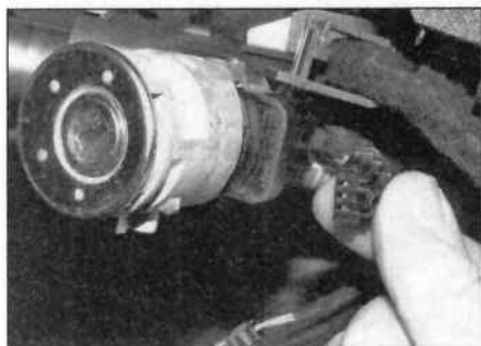
18.5 Disconnect the switch wiring connector (arrowed)
