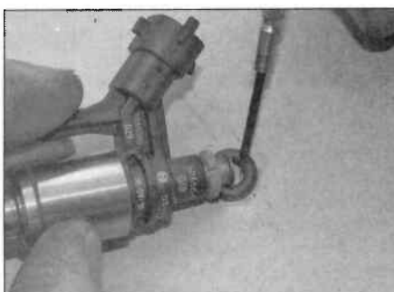
15.20b Remove the upper seal from the injector ...
