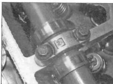
7.14b ... noting the markings for refitting
