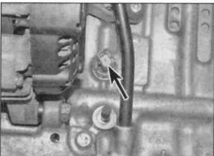
15.3 The oil pressure switch is located on the front face of the cylinder block (arrowed)
