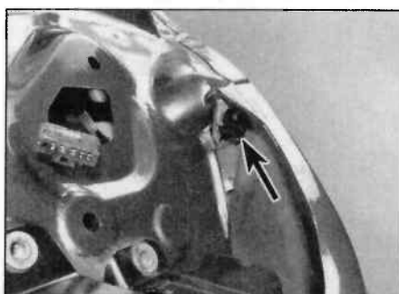
7.3 Turn the clip (arrowed) a quarter of a turn
