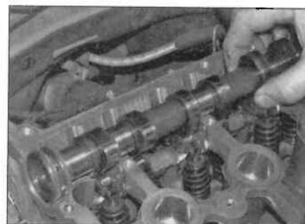
7.15 Remove the camshaft ...
