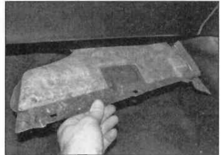
10.60 Remove the trim from inside the footwell
