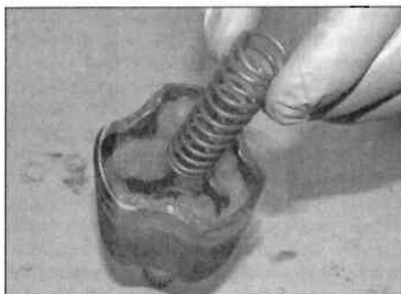
3.27b ... and insert the spring (where fitted)
