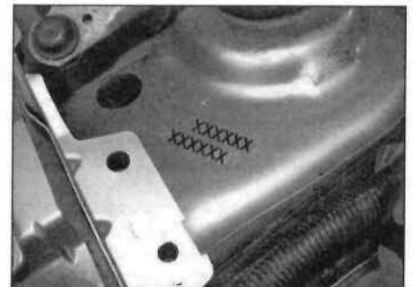
The vehicle identification number (VIN) is stamped on the right-hand inner wing panel
