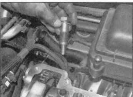
7.10 Remove the timing chain tensioner
