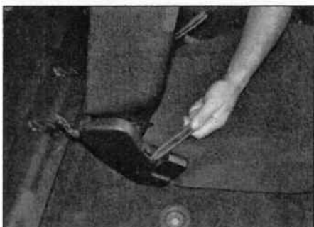
23.13a Pull the strap to tilt the seat back forwards ...
