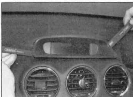
27.17 Unclip the display unit ...
