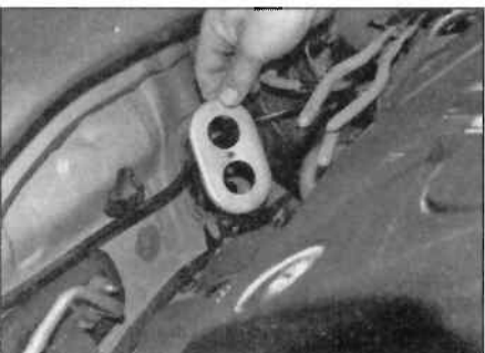
10.44a Remove the heater pipe retaining plate ...
