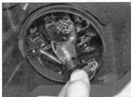
5.16a Rotate the bulbholder clockwise ...
