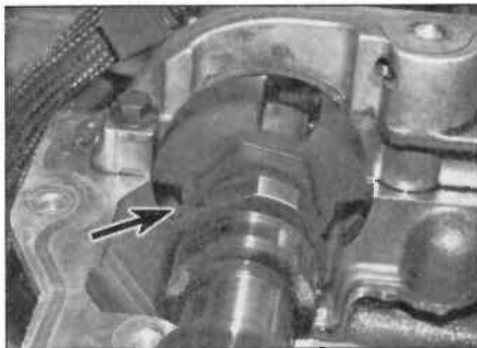
7.29c ... noting that the inlet camshaft will be about 30° out
