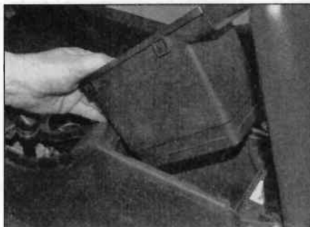
26.10a Lift out the storage compartment ...
