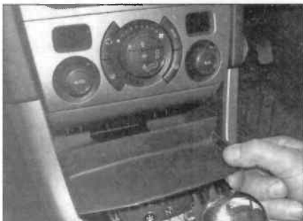
10.1 Remove the rubber tray
