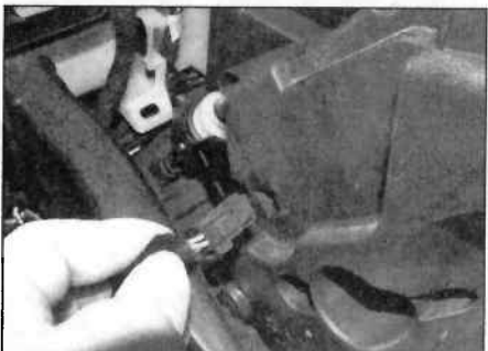
4.7a Disconnect the wiring connectors for the parking lock ...
