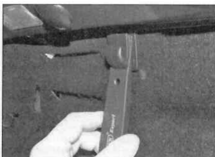
25.31a Carefully unclip the luggage hook ...
