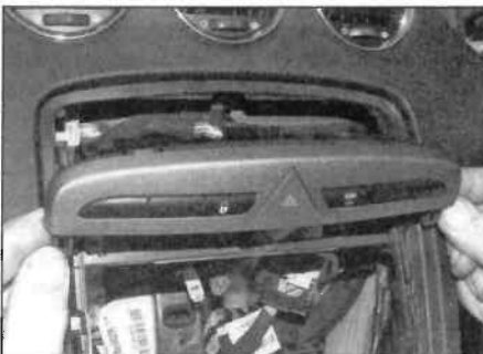
4.17 Unclip the switch panel from the facia ...
