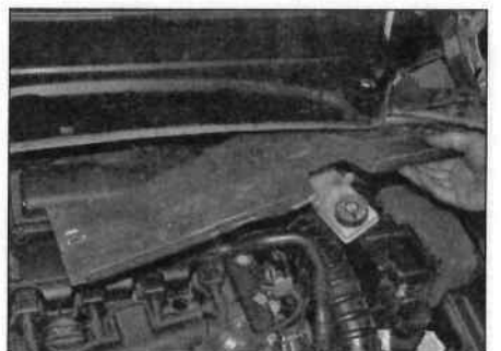
22.8b ... and withdraw the insulation material
