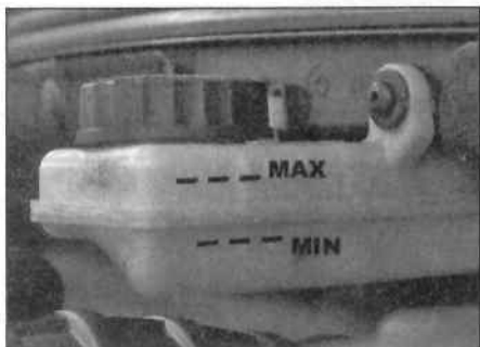
14.3 Brake/clutch fluid level markings
