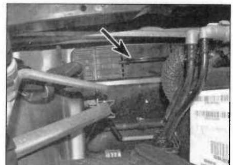
10.3a Pull the filter cover (arrowed) ...
