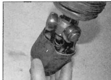
3.28 Refit the tripod joint into the outer joint
