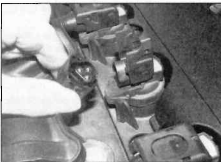
3.4b ... disconnect the wiring connector ...
