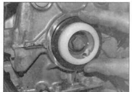
11.5 Locate the oil seal and fitting sleeve over the end of the crankshaft
