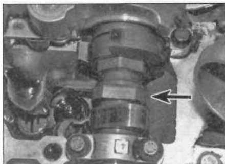
7.29b Make sure the flats are positioned correctly ...
