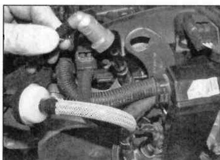
20.3a Release the clip and disconnect the vacuum pipe – petrol engines
