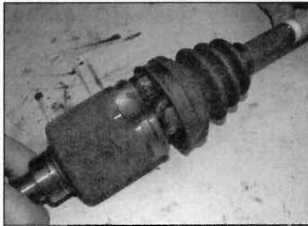
3.18a Slide the joint apart ...
