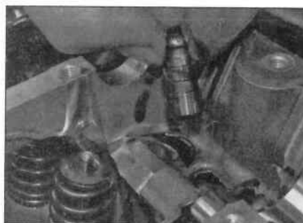
7.18 ... and then the hydraulic tappets
