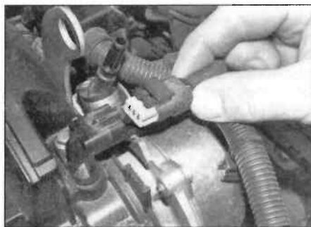
8.6 Disconnect the camshaft sensor wiring connectors
