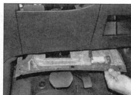
17.5a Remove the trim panel from under the fascia
