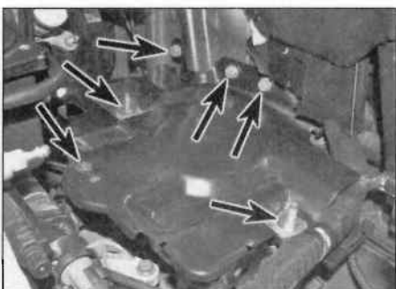
4.15a Undo the battery tray fasteners (arrowed) ...
