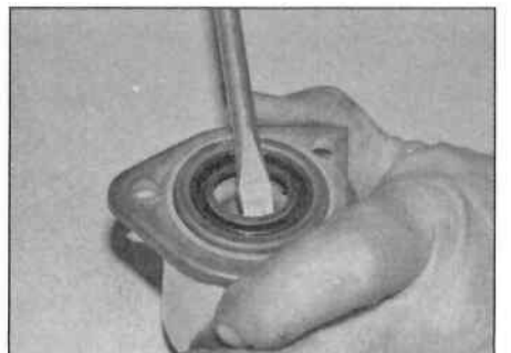
4.8 Remove the input shaft seal from the guide sleeve – BE4/5 transmission
