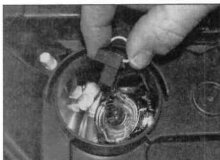
5.5 Disconnect the headlight bulb wiring plug
