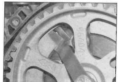
12.18b ... must be 1.2 mm measured with a feeler gauge
