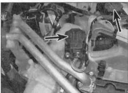
10.69a Two air control motors (arrowed) on the left-hand side of the heater unit
