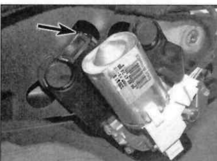
15.5a ... release the securing clip (arrowed) ...
