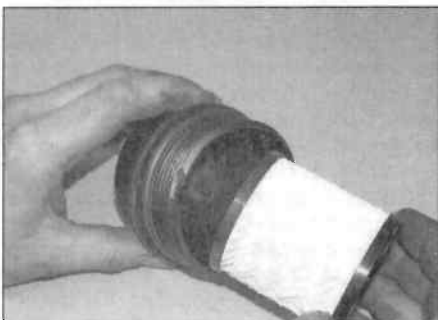
3.11b ... insert the new filter into the cap ...
