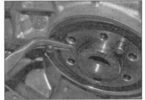
11.10b ... then use a self-tapping screw and pliers to extract the oil seal
