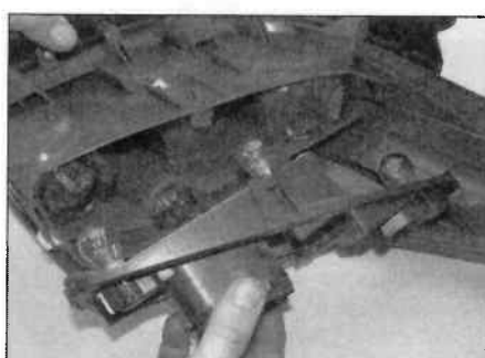
5.32b Release the retaining clips and pull the bulbholder from the light unit – Estate (SW)
