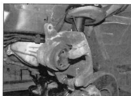
4.4 ... then pivot the caliper upwards and away from the brake pads, and tie it to the suspension strut
