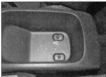
26.9b ... and undo the two retaining screws
