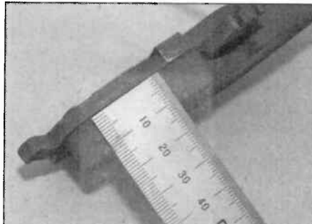
11.7 Check the thickness of the brake pad friction material
