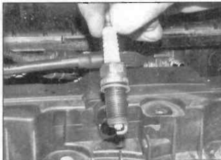
15.4 Examine the spark plugs to check the condition of the engine – see text
