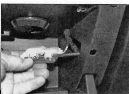
6.11 Unclip the light unit from the inside the glovebox
