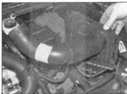
15.4a Remove the front part of the air ducting ...
