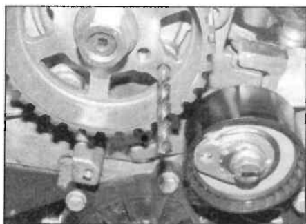
8.17 Insert a suitable drill bit through the sprocket into the hole in the backplate
