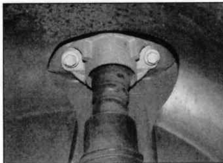
12.3 Undo the two shock absorber upper mounting bolts
