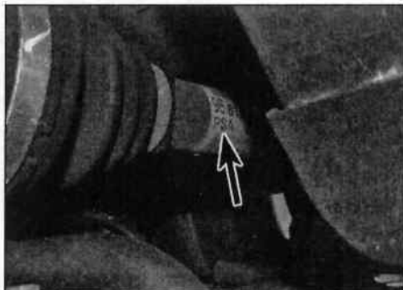
3.0 Make of driveshaft (PSA) written on label (arrowed)
