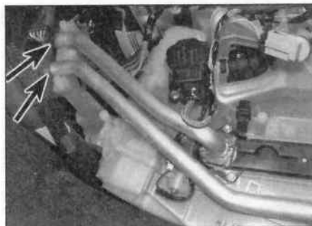
10.25 Make sure the pipes (arrowed) are located correctly in the bulkhead
