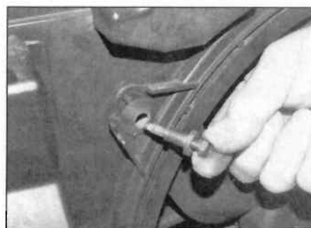
6.3b ... noting the collars fitted to the bolts for refitting
