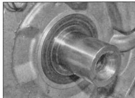
14.5b ... and press the seal into place
