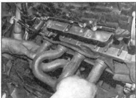
17.10 Remove the exhaust manifold
