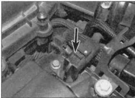
15.40 Camshaft position sensor (arrowed)
