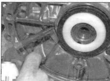
11.13 Apply a small amount of sealer at the casing joints
