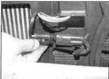
6.5a Disconnect the wiring connector ...
