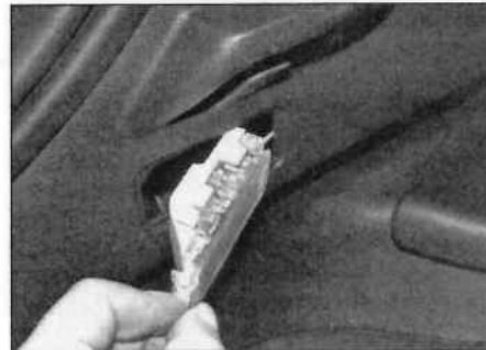
25.37 Unclip the luggage compartment light unit
