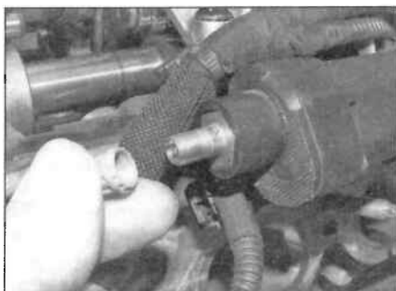
7.2a Pressure relief valve – VTi engine
