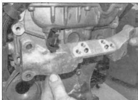
8.14 Remove the engine mounting bracket
