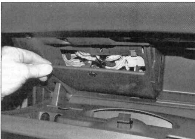
3.3a Rotate the fastener 90° and pull down the cover ...
