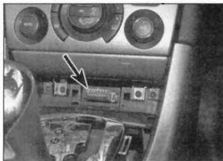
2.2 Vehicle diagnostic plug connector (arrowed)
