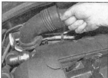
14.2 Remove the inlet hose
