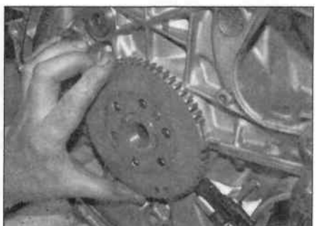
12.4 Remove the TDC timing plate from the crankshaft
