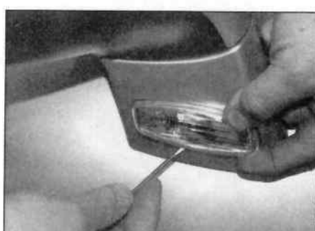
5.28 Unclip the light unit ...
