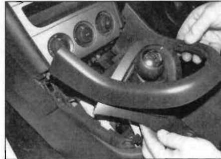
26.5 Unclip the upper trim panel from the fascia
