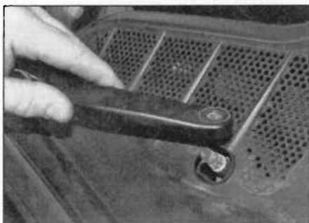
13.3a Remove the wiper arm ...
