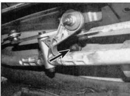
14.9 Locating dowel on bulkhead (arrowed) for wiper linkage
