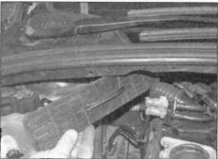
10.3b ... and withdraw it from the bulkhead
