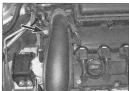
4.5a Undo the rear mounting bolt (arrowed) ...
