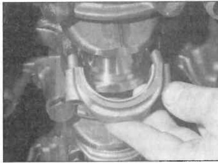
9.5 Remove the big-end bearing shell and cap
