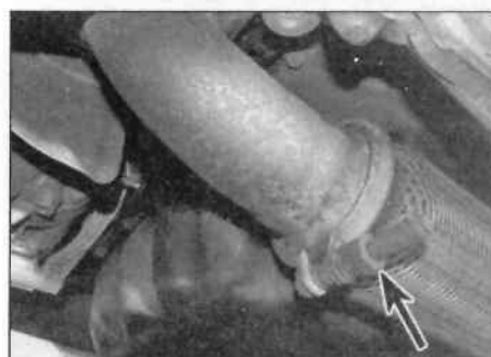
21.13 Front pipe/catalytic converter-to-flexible pipe retaining clamp
