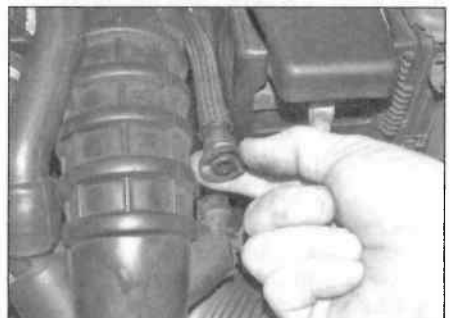
3.8 Disconnect the vacuum hose
