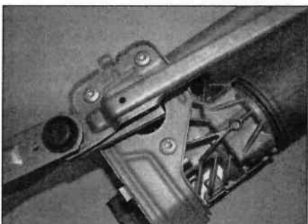
14.8b ... then undo the three retaining screws to remove the motor
