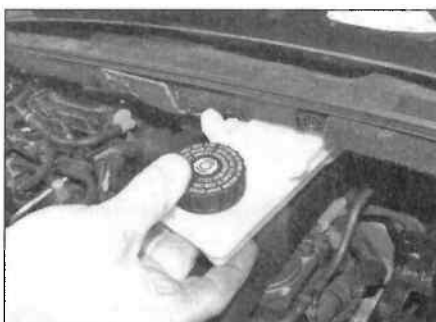
15.6 Remove the brake/clutch fluid reservoir to one side
