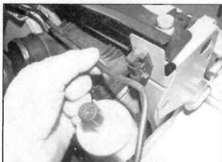
20.4 Unclip the coolant overflow pipe from the retaining clip
