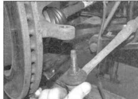
2.7 Disconnect the track rod end
