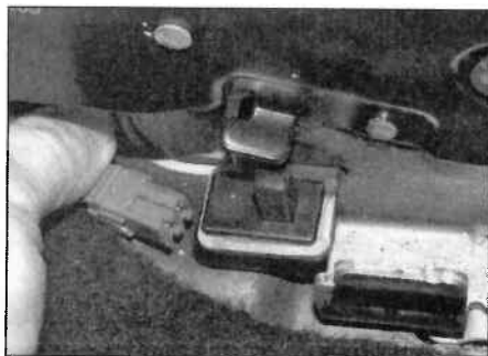
15.4 Disconnect the wiring connector from the switch
