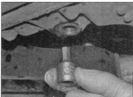
2.3b ... and then remove the inner drain plug/level tube (8 mm Allen key)
