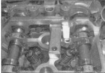
3.1 ... to lock the camshafts in position
