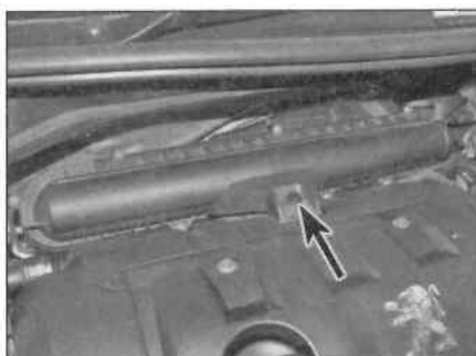
3.1 Undo the retaining bolt (arrowed)
