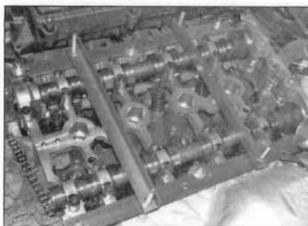
7.1b ... to clamp camshafts in position
