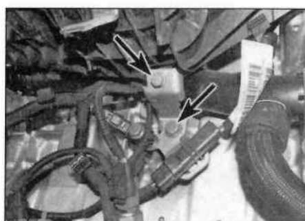
16.9 Undo the bracket mounting bolts (arrowed)
