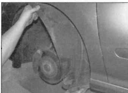
17.3 Remove the inner wheel arch liner
