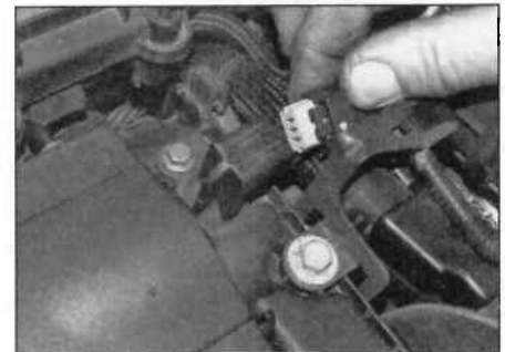
C Check the camshaft sensor wiring connectors are securely connected (turbo petrol model shown).
