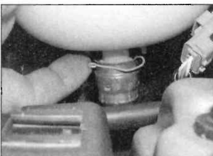
2.12 Where click-fit connectors are used, prise out the circlip then disconnect the hose
