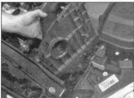
3.8b ... and remove the air intake ducting ...
