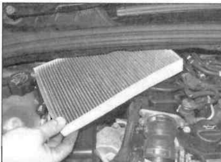
10.4 Slide the pollen filter out from the bulkhead
