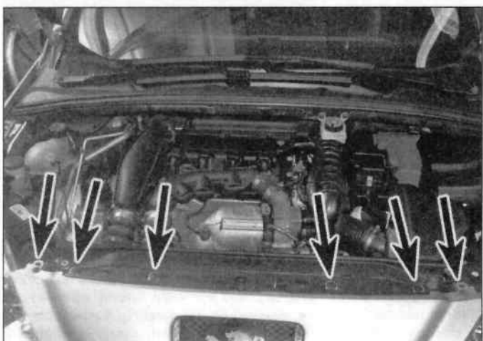
6.5c ... two outer screws and four inner retaining clips (arrowed)
