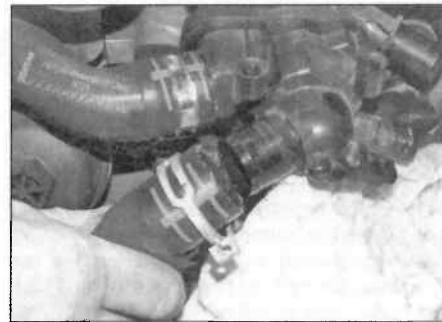
8.8 Disconnect the coolant hoses
