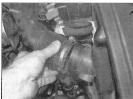
3.13 Disconnect the front of the air inlet ducting
