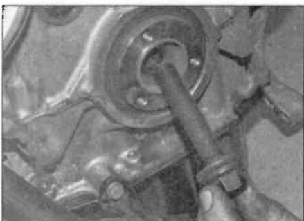
6.14a Remove the crankshaft hub retaining bolt ...
