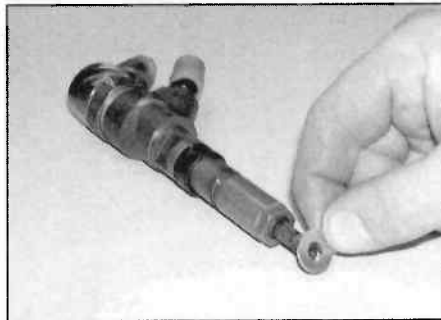
11.13b ... and place a new copper washer on the injector nozzle
