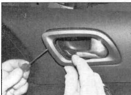
12.5 Carefully unclip the handle surround trim
