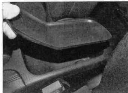
26.9a Pull up the storage tray from the rear of the console ...
