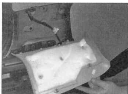
25.16b ... and remove the upper trim panel
