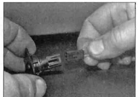
10.78 ... and disconnect the wiring connector
