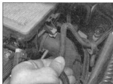
3.14a Unclip the vacuum pipe ...
