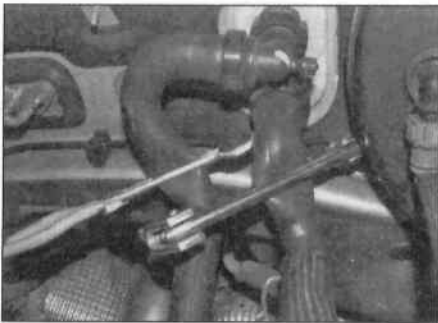
10.13 Using hose clamps to prevent the loss of fluid
