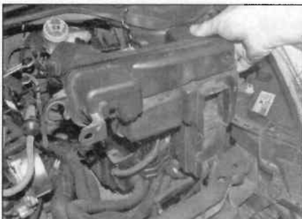
3.7c ... and remove the resonator box
