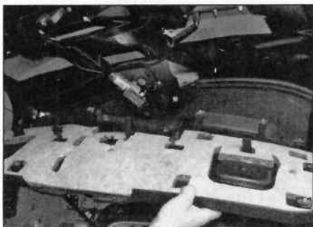
25.72 Unclip the lower trim panel from the tailgate
