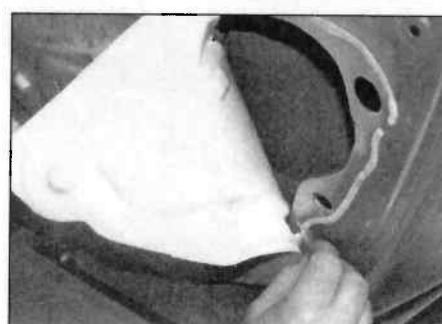
12.24 Using a knife to remove the sealing sheet
