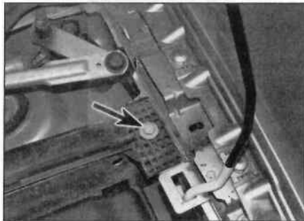
22.7a Undo the retaining bolt (arrowed) ...
