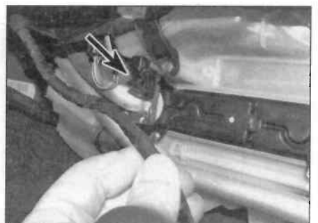
10.18 Release the wiring loom from the retaining clip (arrowed)
