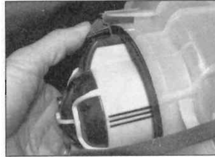
10.33a Release the locking clip ...
