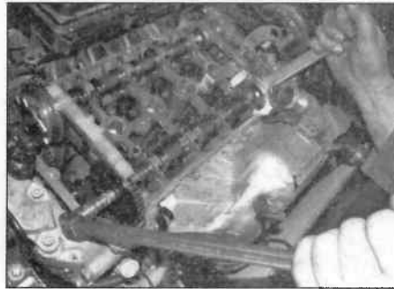
6.8b ... and slacken the camshaft sprocket/dephaser unit retaining bolts
