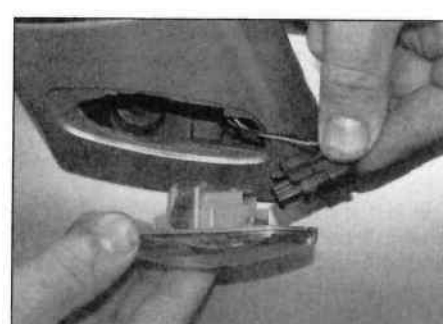
5.29 ... and disconnect the wiring connector
