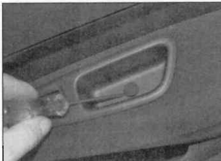
12.11a Unclip the plastic cover ...
