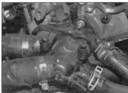
5.7 Note the position of the hoses before removal
