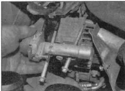
7.9b ... and remove the automatic tensioner
