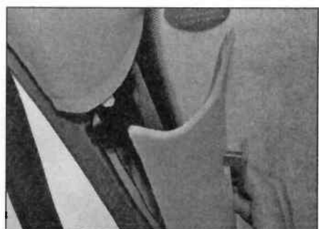
25.4 ... and unclip the pillar trim panel
