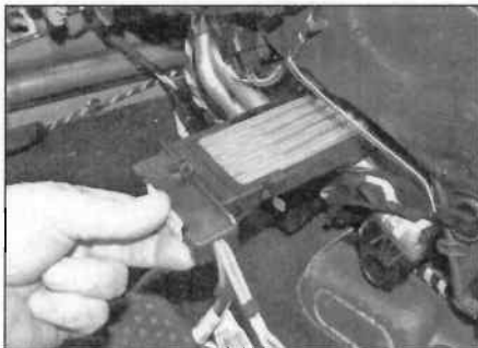
10.66 Additional heater fitted on some models
