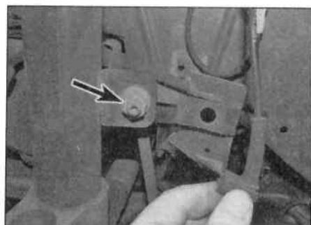
4.2 Undo the anti-roll bar link upper nut (arrowed)
