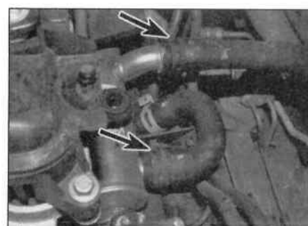
2.29 Release the coolant hose retaining clips (arrowed)
