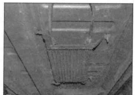
8.1 Fuel cooler fitted under floor panel
