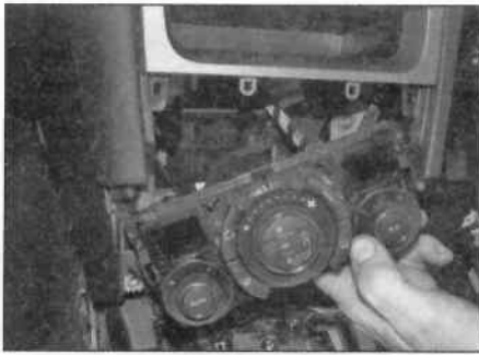
10.4b ... and remove the heater control panel
