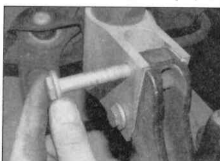
4.3 Remove the strut-to-hub carrier bolts – noting their fitted position
