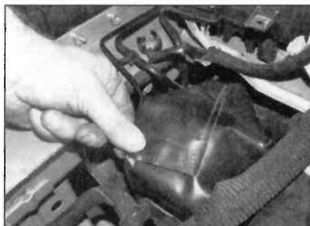
19.6 Remove the plastic weather cover from the unit
