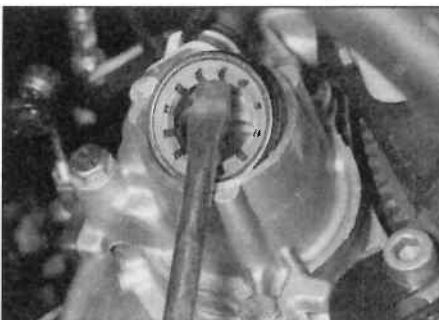
4.2 Use a large flat-bladed screwdriver to prise out the driveshaft oil seals
