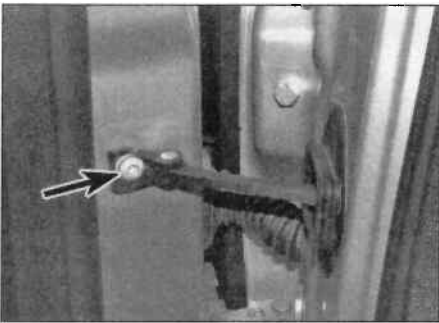
11.3 Undo the door check strap bolt (arrowed)
