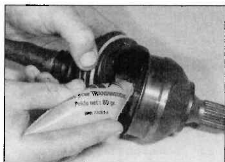
3.11f Pack the joint with grease, working it into the ball tracks while twisting the joint, then locate the gaiter outer lip in its groove on the outer member
