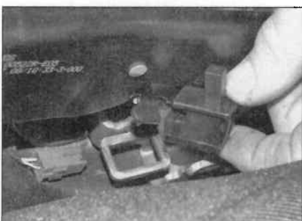
4.31 ... and unclip the switch from the handbrake bracket
