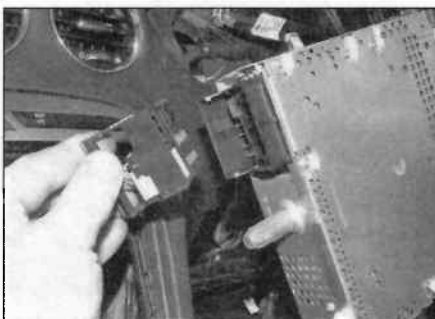
17.3 Disconnect the wiring plug connectors
