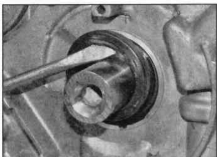
14.3 Take great care not to mark the crankshaft whilst levering out the oil seal
