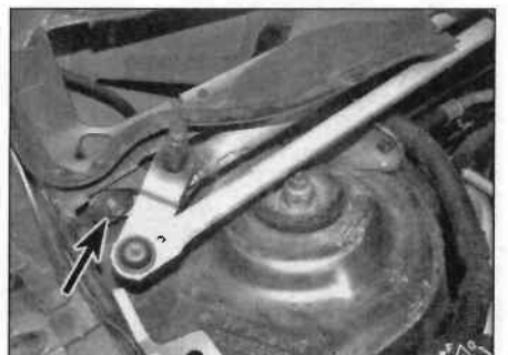
14.6a Wiper linkage right-hand bolt (arrowed) ...
