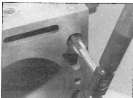
11.8 Use a suitable tap to clean the cylinder block threaded holes
