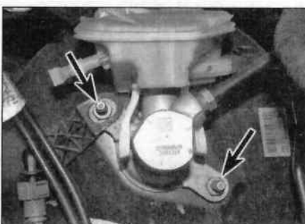
10.7 Master cylinder securing nuts (arrowed)
