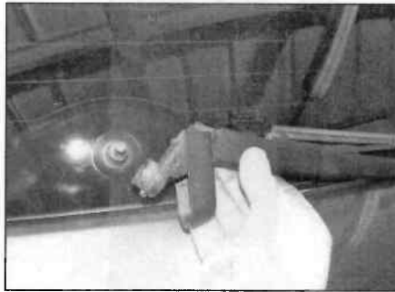
13.8 Remove the wiper arm from the spindle
