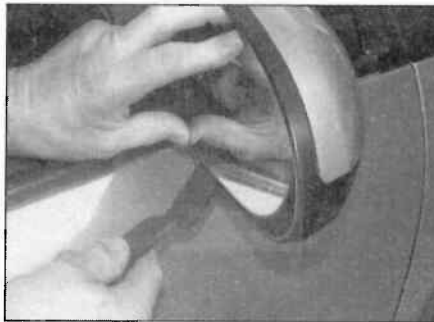
18.6 Carefully lever the lower edge of the mirror glass to remove
