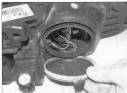
5.9 Unclip the headlight bulb protective cover
