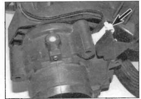
14.10b ... release the locking clip (arrowed) ...
