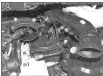
15.4c ... and remove the rear part of the air ducting
