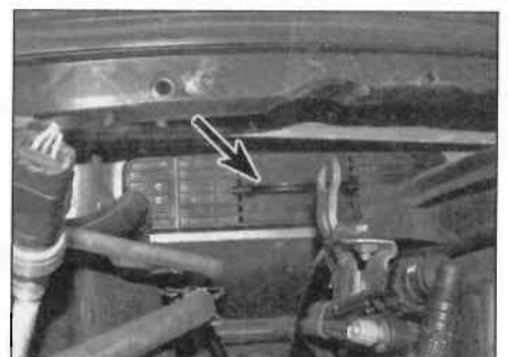
9.3a Pull the filter cover (arrowed) ...
