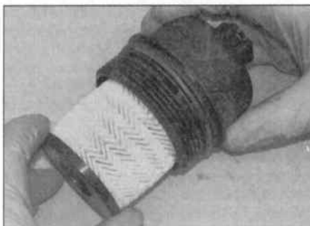
3.14a ... insert the new filter into the cap ...
