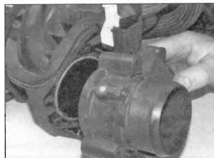
14.10c ... then remove the throttle housing from the manifold
