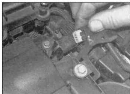
4.11 Disconnect the camshaft sensor wiring
