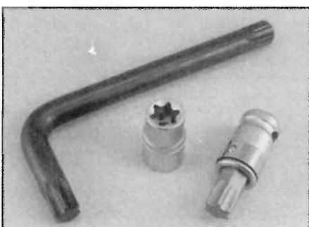
Torx key, socket and bit
