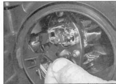
5.10 Disconnect the headlight bulb wiring plug
