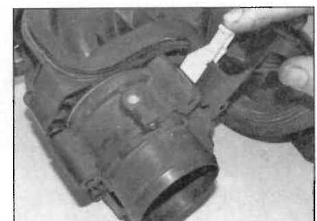
14.11c Push the locking clip back into place – THP models
