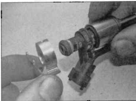
15.19b ... and remove the retaining clip
