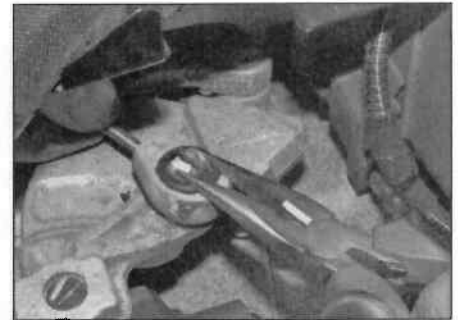
4.3b ... or squeeze the retaining clips to release the cable balljoint
