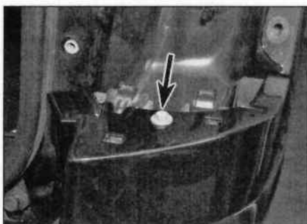
7.11 Bumper upper retaining bolt (arrowed)
