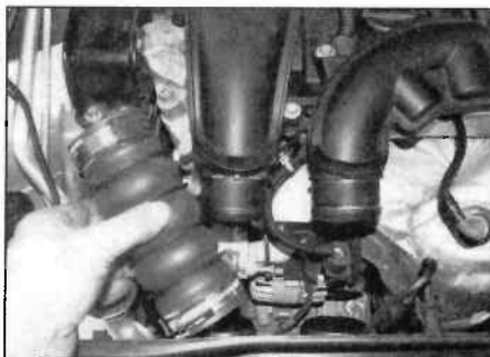
7.3 Remove the air inlet hoses from the intercooler
