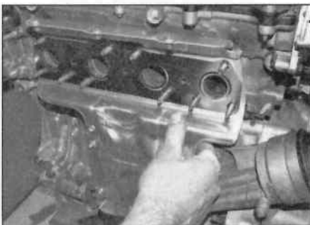
17.16 Manifold gasket has built-in heat shield – VTI engines
