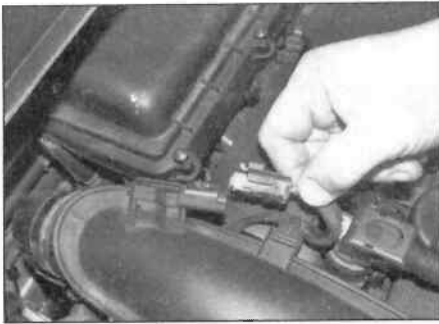
14.6 ... disconnect the sensor wiring connector ...
