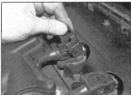
3.4a Release the locking clip ...
