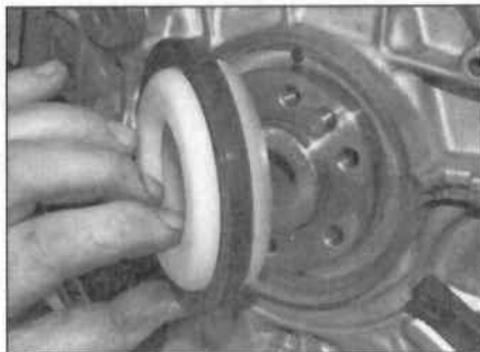
11.12a The new oil seal comes with a protective sleeve ...
