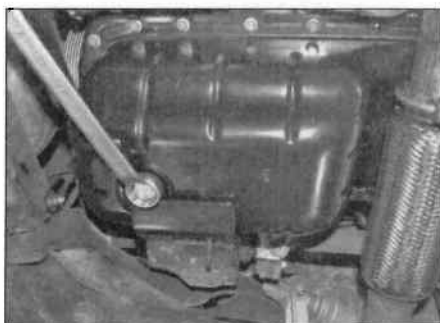
3.4a Using a spanner to slacken the sump drain plug ...
