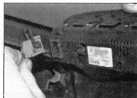
10.3 ... and disconnect the wiring connector
