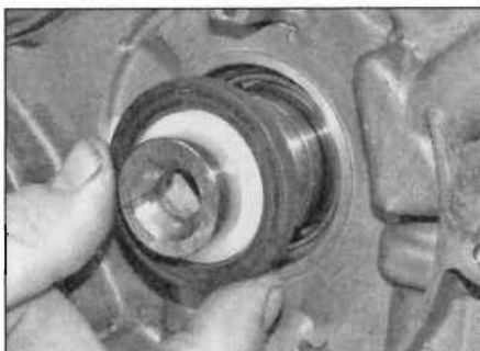
14.5a Slide the seal and protective sleeve over the end of the crankshaft ...
