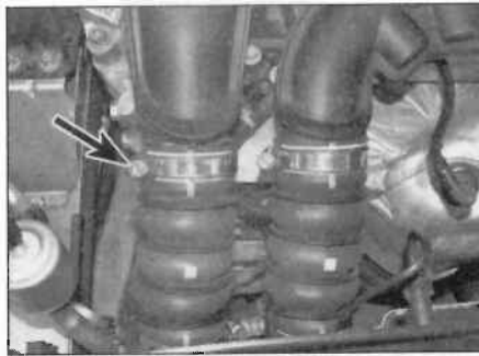
14.7 ... slacken the retaining clip (arrowed) ...
