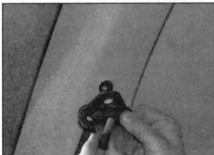
24.16a Prise off the cap and undo the anchor bolt - C-pillar
