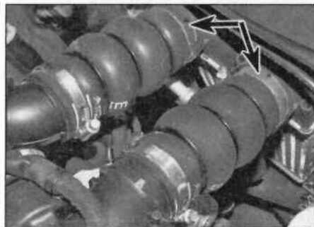
17.3 Remove the upper hoses (arrowed) from the intercooler
