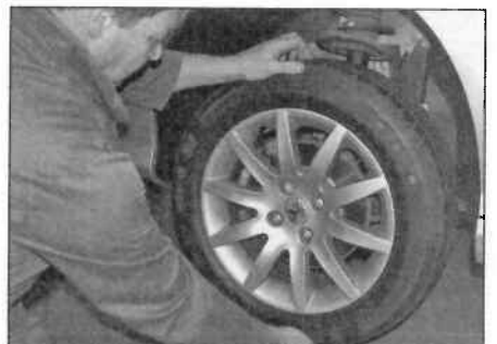
13.3 Check for wear in the hub bearings by grasping the wheel and trying to rock it
