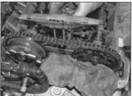
7.8 Remove the guide/anti-knock pad from the cylinder head
