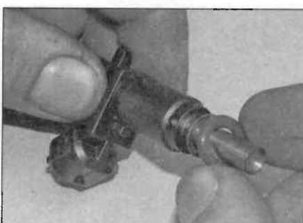
15.8 Remove the seal from the end of each injector
