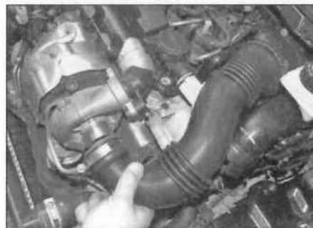
15.2d ... and remove the air intake hose
