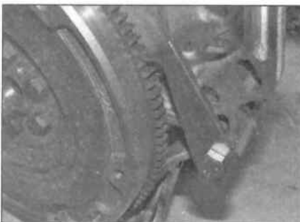
12.2 Use a tool to lock the flywheel ring gear and prevent rotation
