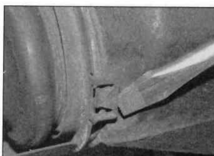
7.2 Release the clips and remove the balljoint protector plate
