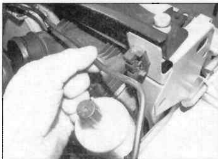
17.4 Unclip the coolant overflow pipe from the retaining clip
