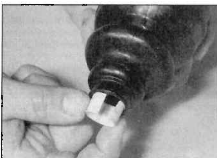
3.6 Where applicable, remove the plastic bush
