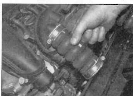
4.2b ... and remove the air inlet hoses
