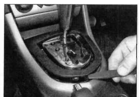
26.2b ... and outer gear selector surround trims
