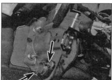
12.9 Undo the two cross-over bar mounting nuts (arrowed)
