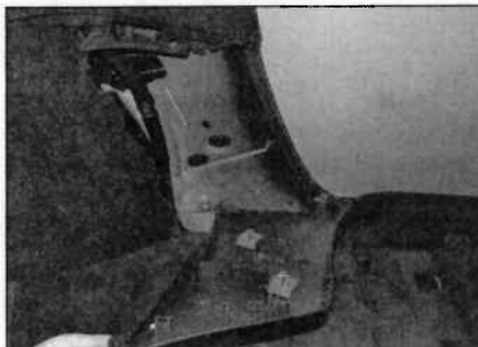
25.36 Unclip the lower trim panel
