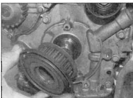
8.11a Slide the sprocket from the crankshaft ...
