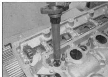
11.15 Fit the injectors into their original locations
