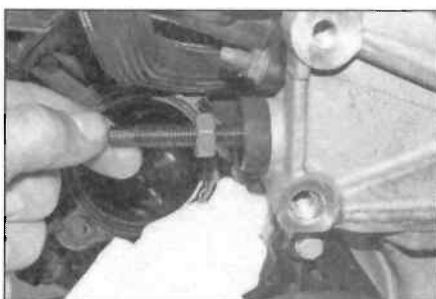
6.4b Screw the threaded centre part of the tool in until it contacts the timing chain guide and hand-tighten
