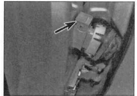
11.2 Lever up the locking catch (arrowed) and disconnect the wiring plug
