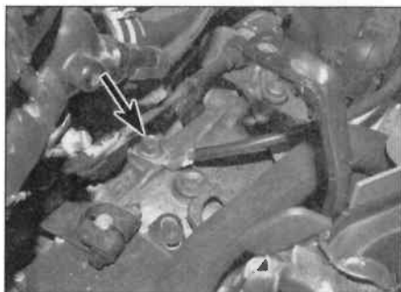
9.3 Engine/transmission earth strap connection (arrowed)
