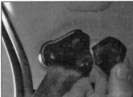
24.16b Prise off the cover and undo the anchor bolt - D-pillar
