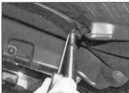
19.4 Prise out the clip and pull the strut from the upper balljoint
