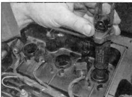
3.3 ... and withdraw the ignition coil
