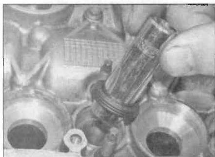
9.32a Fit the new seal around a 20 mm outside diameter socket ...
