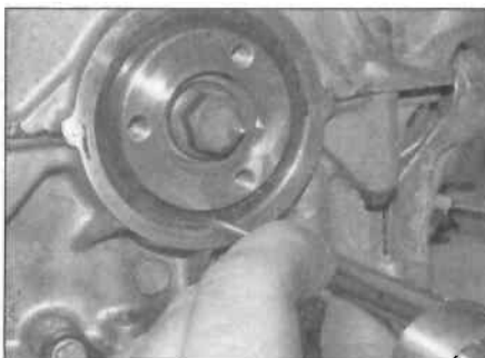
11.6 Tap the seal squarely into position
