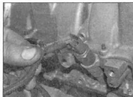
14.2 Disconnect the wiring connector from the oil level sensor
