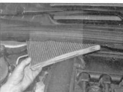
9.4 Slide the pollen filter out from the bulkhead
