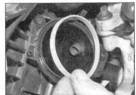
14.11a Fit new sealing ring – VTI models
