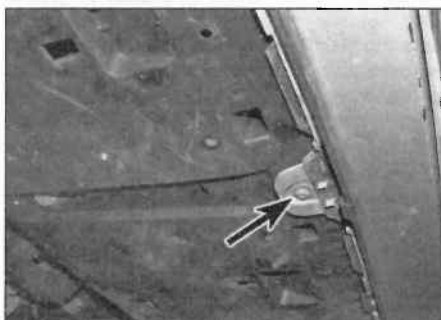
6.4b ... and the screw (arrowed) at the centre
