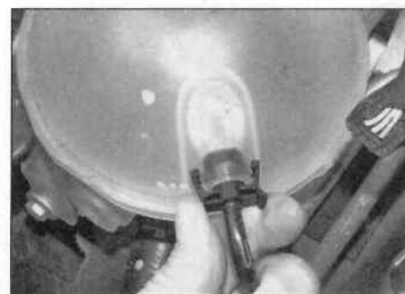
3.2 Squeeze the clips to disconnect the coolant pipe
