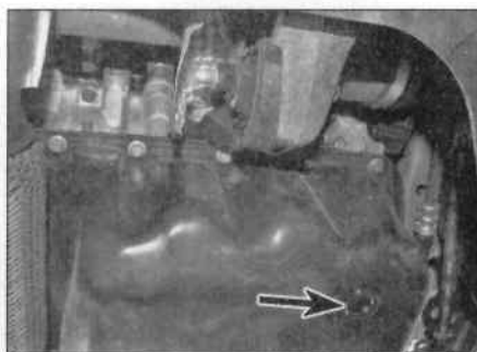
3.4b ... some drain plugs will need a square-section wrench
