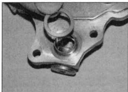
12.12a Fit a new seal ...
