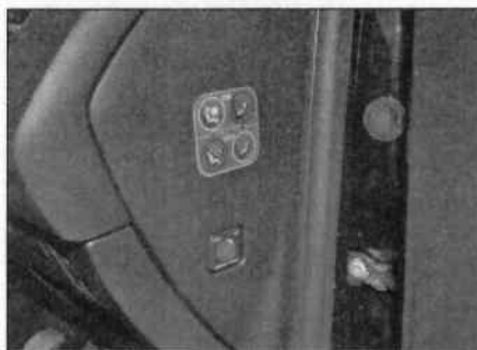
21.6 Passenger airbag disabling switch
