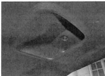
25.70 Undo the retaining screws in the handle recess
