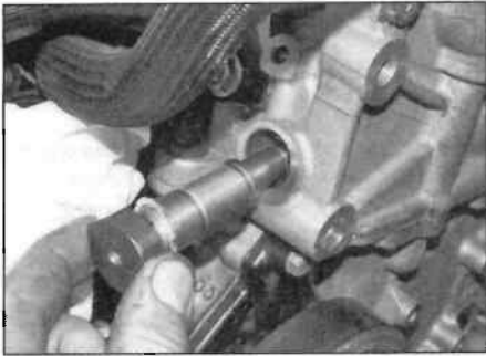
6.11 Remove the timing chain tensioner
