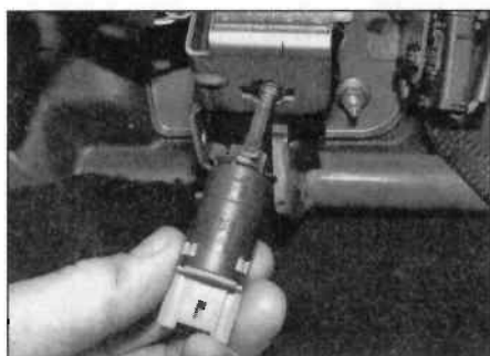
17.3b Rotate the brake light switch 90° anti-clockwise, and pull it from the bracket switch 90° anti-clockwise and remove it from the bracket (see illustrations).
