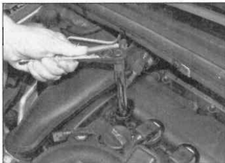
15.3a Unscrew the spark plug ...
