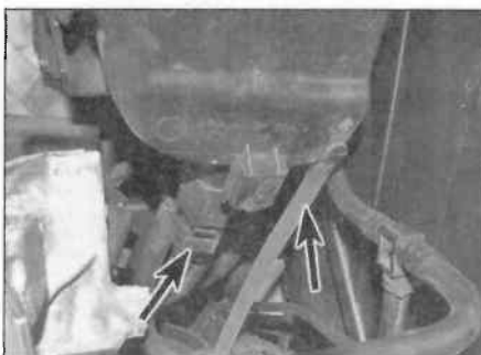
16.8c Disconnect the wiring connector and the drain tube (arrowed)
