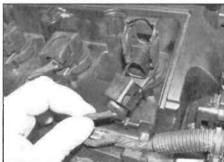
3.2b ... disconnect the wiring connector ...
