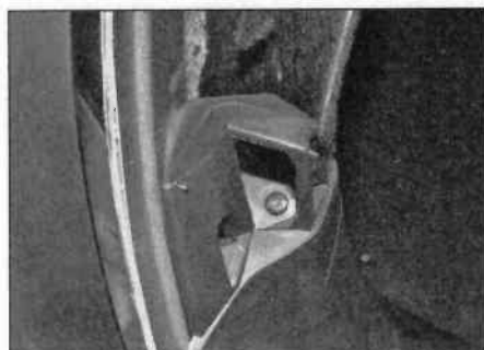
25.42 Undo the rear trim upper retaining screw
