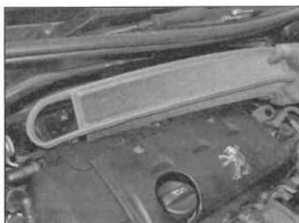
3.3 ... and remove the air filter element
