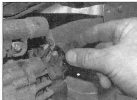
7.7b ... prise out the rubber cover ...
