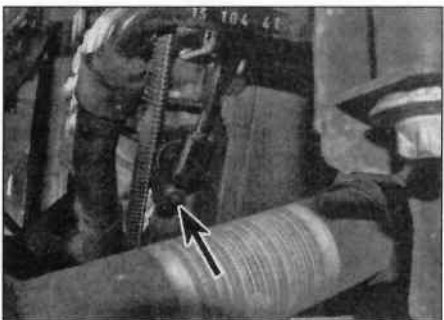
8.49a input shaft speed sensor securing bolt (arrowed)
