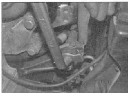
10.7a Turn the tensioner arm clockwise ...
