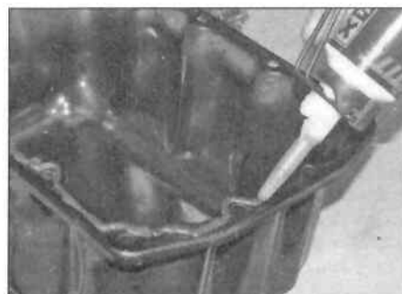
9.10 Apply a thin bead of RTV sealant to the sump mating surface
