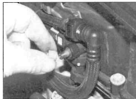
7.2b Pressure relief valve – THP engine
