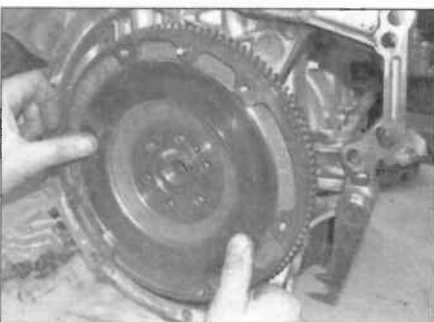
12.3b ... and remove the flywheel
