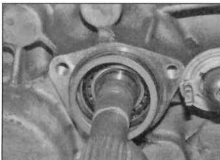
4.7b ... and any shims, where fitted – BE4/5 transmission
