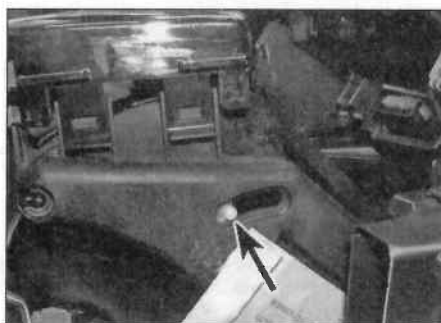
1.6b ... the locking lever (arrowed), to move it out of (P) park position
