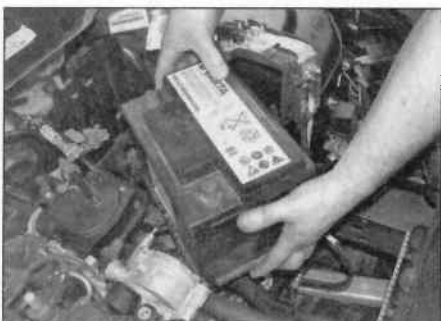
4.10 ... and then lift out the battery
