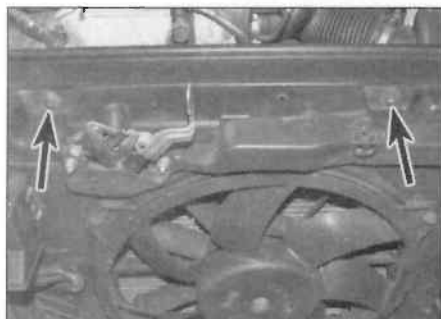
4.6a Undo the radiator upper mounting screws ...
