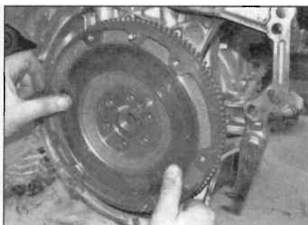
12.3b ... and remove the flywheel
