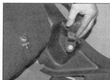
25.22 Undo the seat belt lower anchorage bolt
