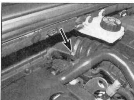
16.2a Slacken the retaining clip (arrowed) ...
