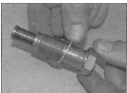
6.27 Fit new washer to tensioner
