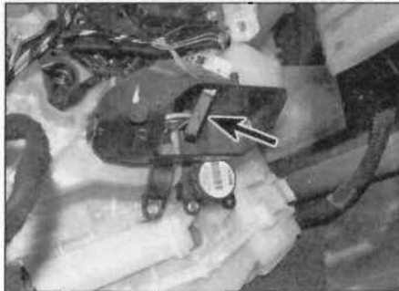
10.59 Interior air temperature sensor (arrowed)
