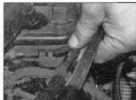
16.18 Disconnect the vacuum pipe from the reservoir
