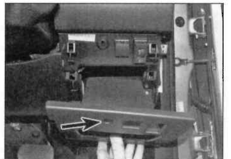
4.21 Turn the securing clip (arrowed) and remove the trim panel
