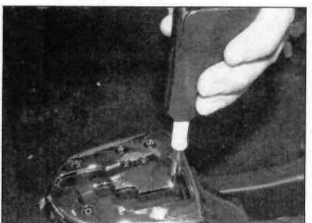
4.11a Pull the gear knob from the lever ...
