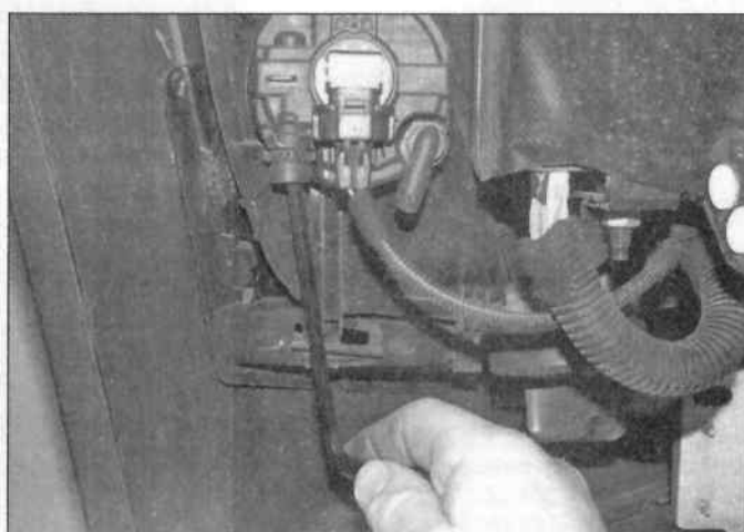
8.4 Using an Allen key to adjust the front foglight alignment
