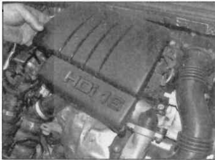
4.2 Pull the plastic cover upwards to release the rubber mountings
