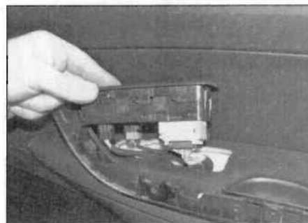
12.6b ... and remove the switch assembly
