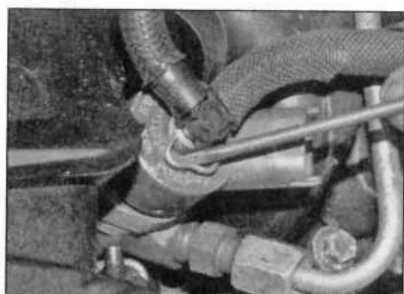
11.7 Prise out the clip and pull the return pipe from each injector
