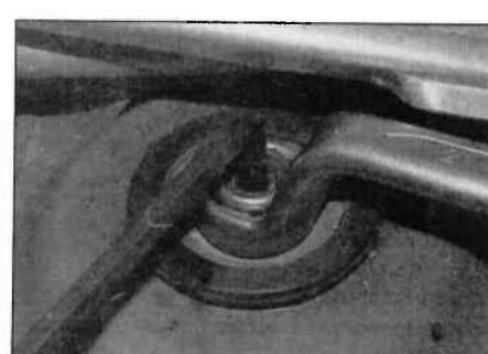
4.6b ... and use an Allen key to counterhold the rod whilst slackening the nut
