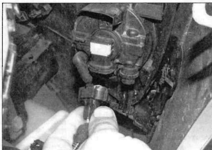
6.6a Disconnect the foglight wiring ...
