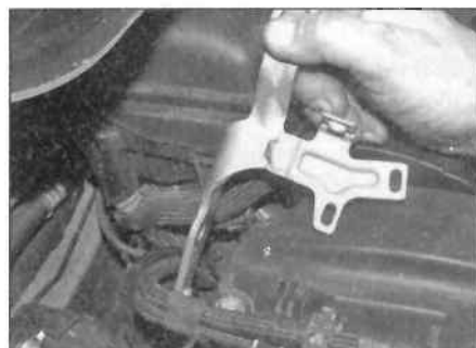
4.9b ... and remove the mounting bracket
