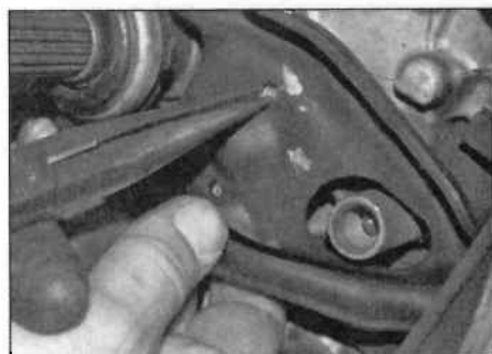
7.2 Squeeze the tabs of the retaining clip together and remove the release fork ...
