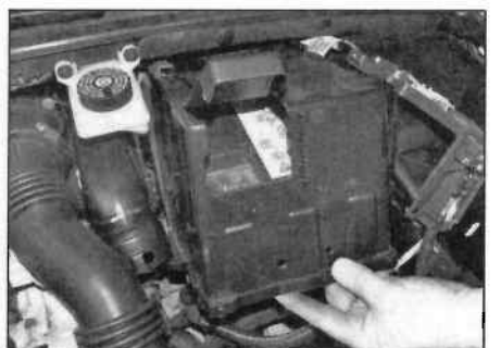
4.7a Remove the cover from the battery ...
