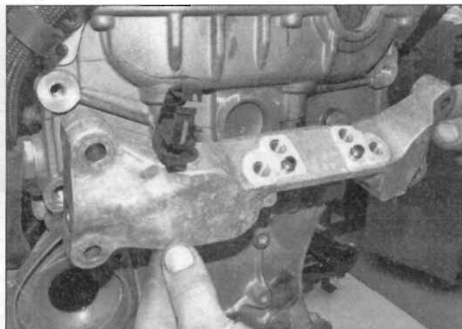
13.7 Remove the engine mounting bracket
