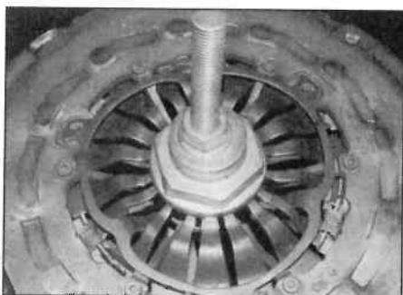
6.16 Using some threaded rod, washers and nuts, compress the spring and the pressure plate together ...
