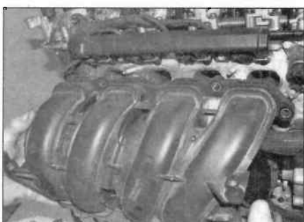
16.10b Withdraw the manifold from the head
