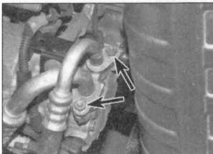
12.4 Undo the nuts (arrowed) securing the refrigerant pipes to the condenser
