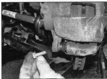
4.13 Pivot the caliper down and over the pads, then fit and tighten the new caliper guide pin bolt
