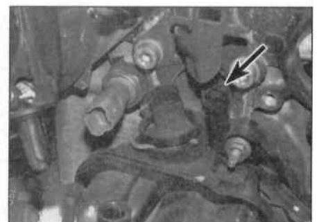
20.5b ... and the bleed screw (arrowed) on the coolant housing
