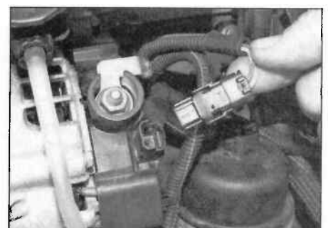
7.4b ... then disconnect the alternator wiring and plug ...
