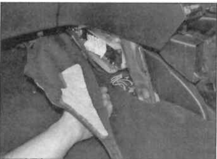
10.16 Undo the retaining screw and remove the trim panel
