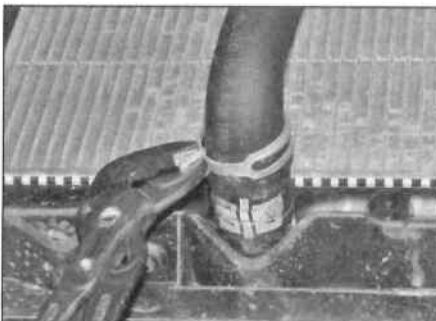
20.4 Squeeze together the tabs to release the hose clamp
