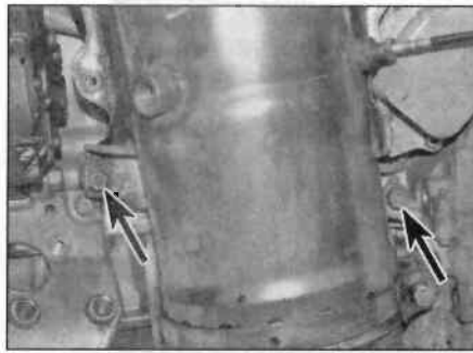
18.11 Catalytic converter/particulate filter retaining nuts (arrowed)
