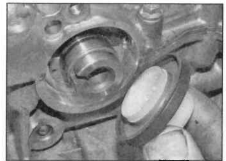
14.18 Fit the protective sleeve and seal over the end of the camshaft
