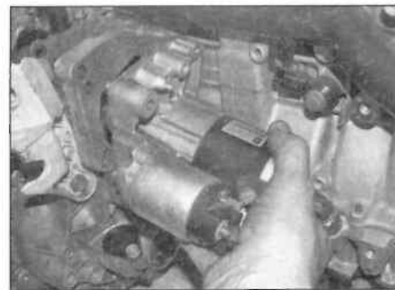
10.9 Remove the starter motor
