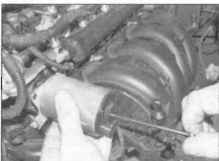
8.11b ... and withdraw the actuator from the cylinder head using an Allen key
