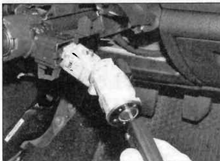
18.7b ... and slide the switch from the steering column
