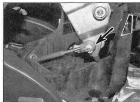
3.3b ... and disconnect the end of the cable (arrowed) – MCM and BVM6 transmissions
