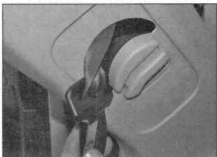
25.10c ... pass the seat belt through the trim on removal
