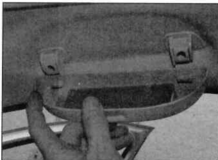
25.87b ... and remove the sunglasses holder
