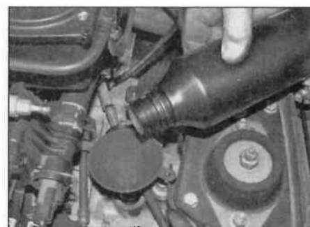
2.13b ... and add the exact amount of fluid specified using a funnel
