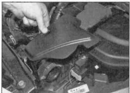
5.2 Unclip the air inlet ducting cover
