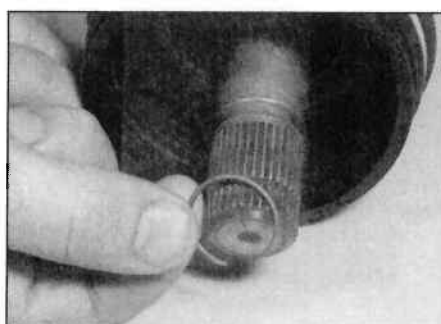
3.11d Fit the new circlip to its groove in the driveshaft splines ...
