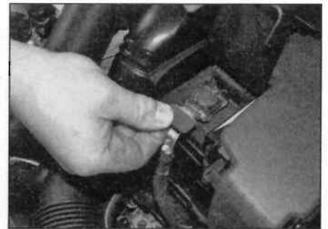
4.4b ... then lift up the quick-release lever and disconnect the positive lead
