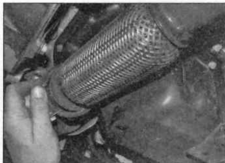
17.7 Undo the clamp from the front pipe
