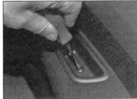
12.11b ... and undo the retaining screw
