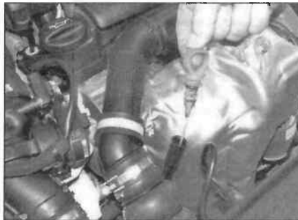
3.16b ... and the oil level dipstick
