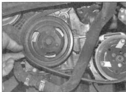
10.9 Remove the belt from the pulleys
