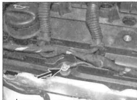
4.8a Undo the earth wire connection (arrowed) ...
