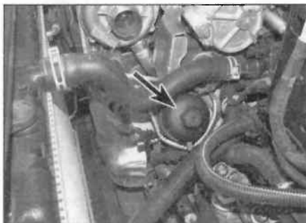
3.9 ... to access the oil filter (arrowed)
