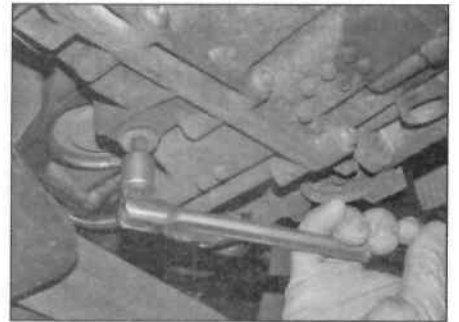
18.5b Remove the square-drive (8 mm) plug to check level – AL4 and AT8 transmissions
