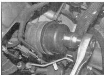
3.8a Slacken the filter cover ...
