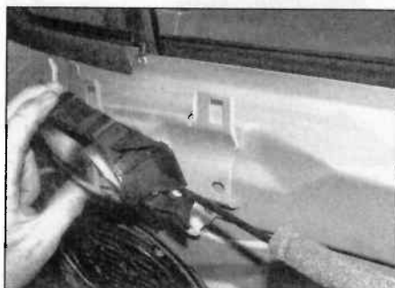
13.2a Release the handle from the door ...
