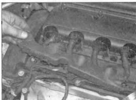
4.7b ... and unclip the plastic trim
