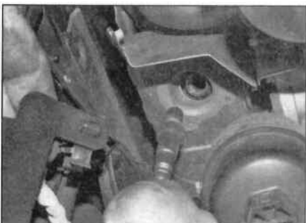
17.5 Remove the oxygen sensor ...
