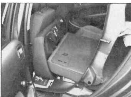
25.24 Remove the trim panel from the C-pillar
