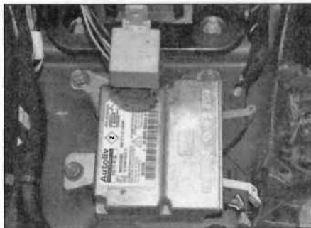
22.16 Undo the airbag ECU retaining nuts
