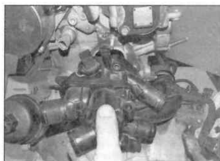
8.10 Withdraw the housing from the cylinder head
