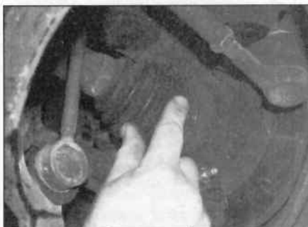
5.1 Check the driveshaft gaiters for signs of damage or deterioration
