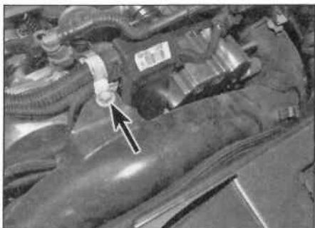
3.14b ... undo the retaining bolt (arrowed) ...
