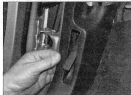
9.7 Unclip the trim panel from around the lever
