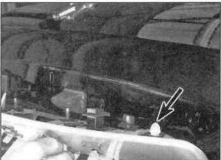
16.15 Release the retaining clips (arrowed) – one at each end
