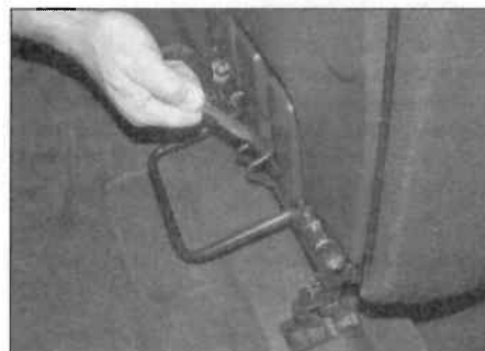
23.13c ... then pull the red strap to release the seat catches from the floor
