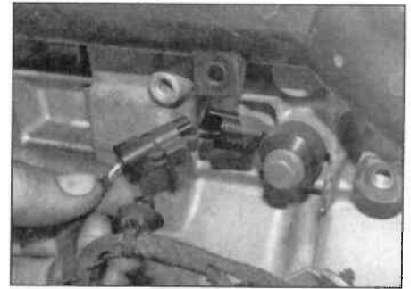
5.3 Disconnect the knock sensor wiring plug
