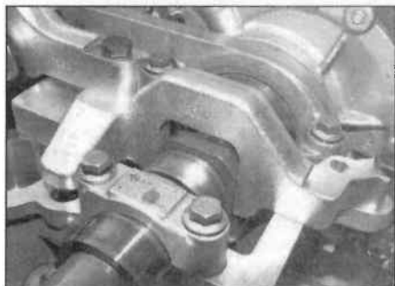
3.6 Bolt the special tool over the camshafts to lock them in position
