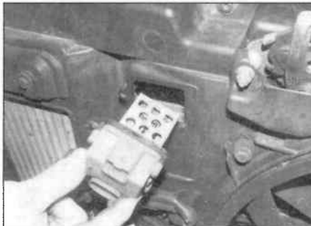
6.8c ... and remove the cooling fan resistor
