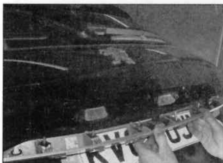
7.32 Remove the switch/handle rear trim panel
