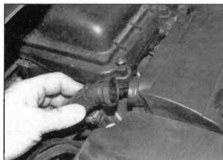
16.16 Disconnect the breather pipe
