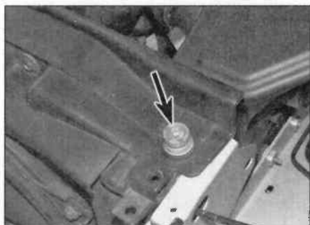
17.6 Undo the front panel outer retaining bolts (one side arrowed)
