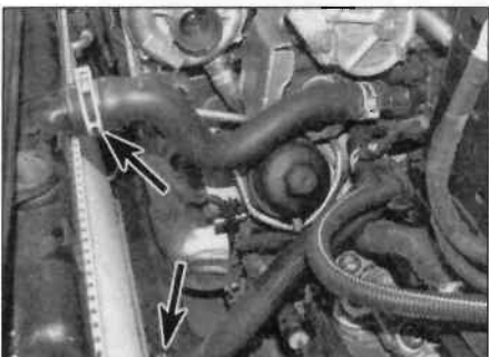
4.4 Disconnect the upper and lower radiator hoses (arrowed)
