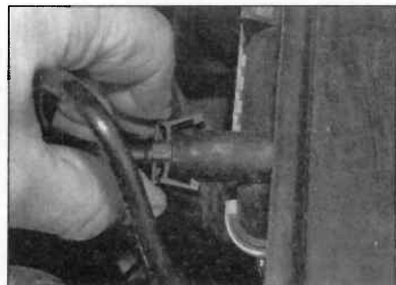
4.5 Squeeze the clips to disconnect the coolant pipe
