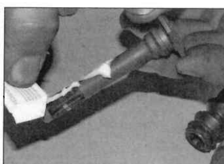
4.8d Use the special grease to lubricate the pins
