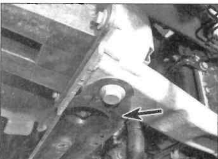
9.9 Remove the strengthener bar (arrowed)
