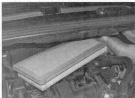
16.4a Remove the air filter element on THP turbo engine ...
