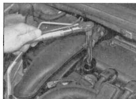
15.11 Use a torque wrench to tighten the spark plugs
