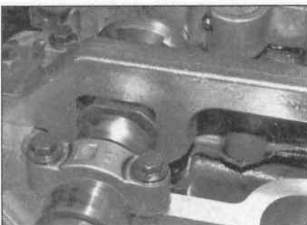
3.6a Bolt the special tool over the camshafts ...
