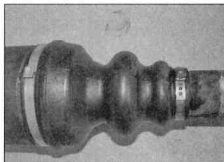
3.42 Fit the new clips and crimp them into place
