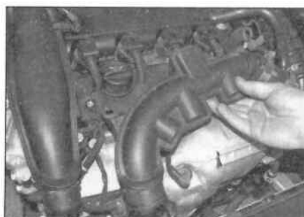
4.3b ... and remove the air inlet ducting
