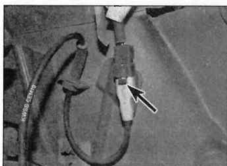
19.16 Disconnect the front sensor wiring connector (arrowed)
