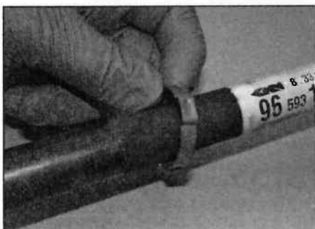
3.24 Make sure the inner retaining clip is put on the shaft
