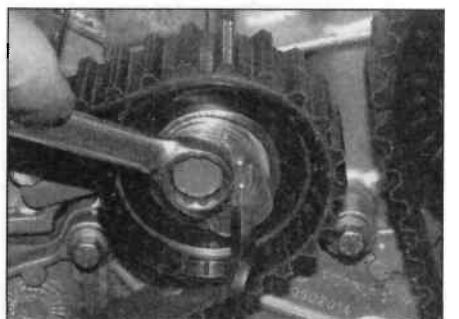
7.13 Slacken the bolt and allow the tensioner to rotate, relieving the tension on the belt
