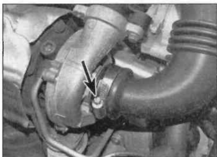
15.2b ... and the retaining clip (arrowed) on the turbo ...
