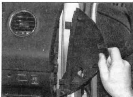
27.23 Unclip the trim from the end of the fascia
