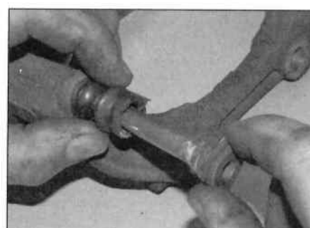
4.8a Check the condition of the guide pins ...
