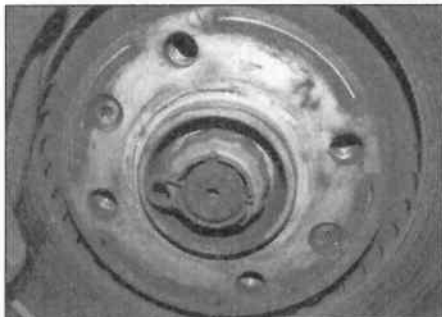
2.5a Use a screwdriver to prise out the R-clip
