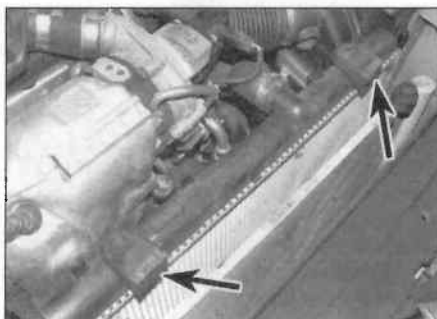
4.6b ... and remove the upper mountings (arrowed) ...
