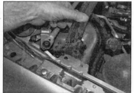
22.7b ... and unclip the scuttle crossmember
