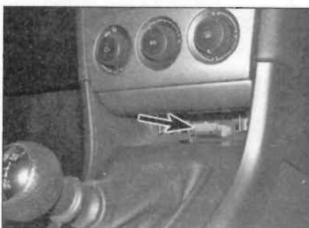
13.2 Diagnostic plug connector (arrowed)
