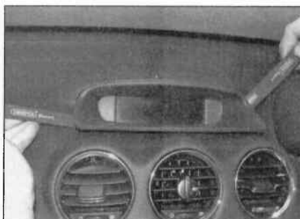
10.2 Unclip the display unit from the fascia ...
