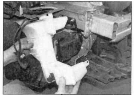
16.8b ... then tilt the reservoir to remove from wing panel
