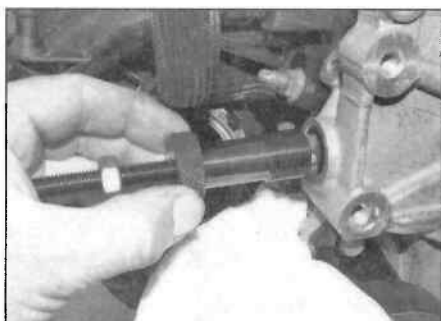
6.4a Insert the tool into the cylinder head where the chain tensioner fits
