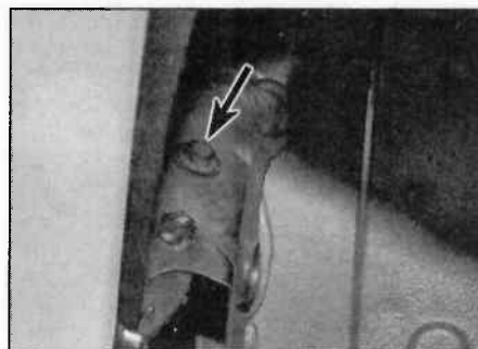
7.7 Undo the bumper-to-wing bolt (arrowed)
