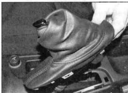
26.8b ... and withdraw it over the handbrake lever to remove
