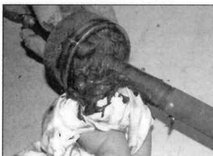
3.3b ... and clean out the old grease
