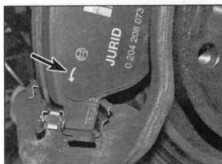
4.12 Refit the pads, with the arrow (arrowed) in the direction of rotation
