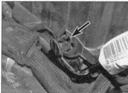
4.7b ... releasing it from the locating peg (arrowed)
