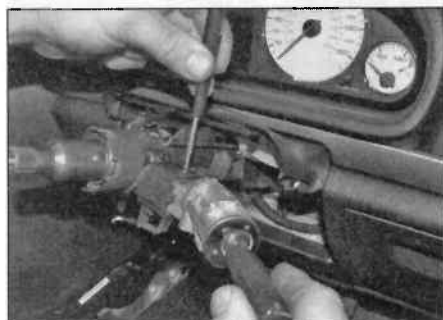
18.7a Depress the locating peg with a thin screwdriver ...
