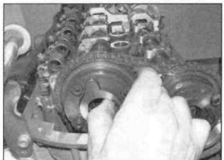
6.26 Refit the camshaft sprockets
