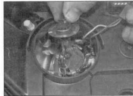
5.6b ... and remove the bulb
