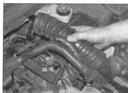
16.2b ... and disconnect the air intake hose
