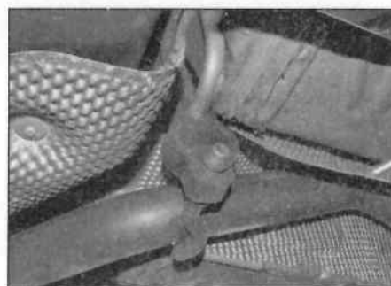
21.21a Exhaust centre rubber mounting ...
