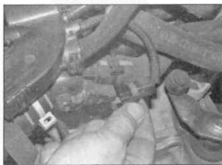
8.5a Disconnect the thermostat wiring connector
