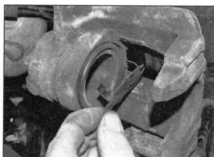
4.5b Check the shim (where fitted) in the caliper piston
