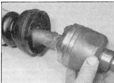
3.37a Release the inner gaiter retaining clips and remove the joint outer member
