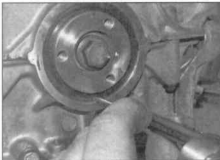
11.6 Tap the seal squarely into position
