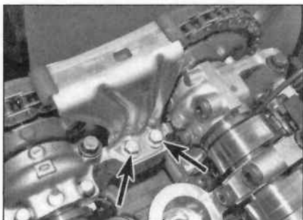
6.27 Refit the guide/anti-knock pad securing bolts – arrowed
