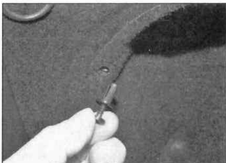
7.12b ... release the securing clips ...
