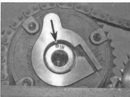
6.20 Check the alignment marks are in position (arrowed)
