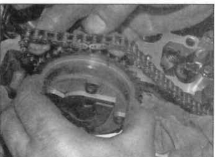
7.11b ... and inlet camshaft dephaser unit
