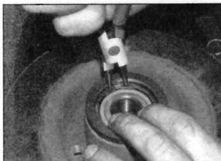
11.11 Fit the new bearing retaining clip
