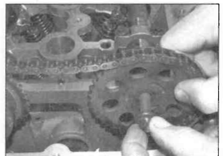
6.16a Undo the sprocket retaining bolt ...
