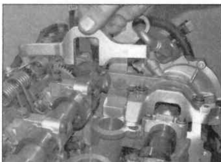
3.1 ... to lock the camshafts in position
