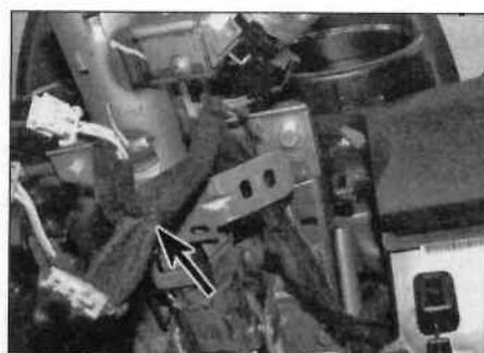
17.7 Unclip the wiring loom (arrowed) from the steering column
