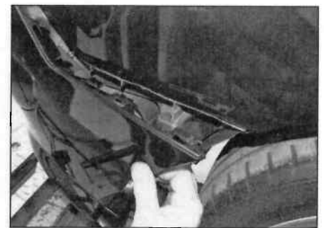
7.15 Release the bumper from the sides at the rear wings
