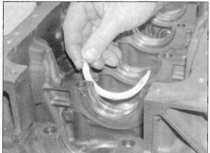
17.21 Place the thrustwashers each side of the No 2 bearing upper location
