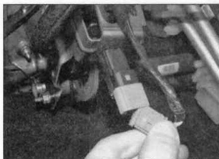
17.3a Disconnect the wiring connector from the switch
