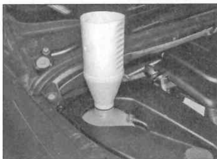
20.19 Using a 1.0 litre plastic bottle as a header tank
