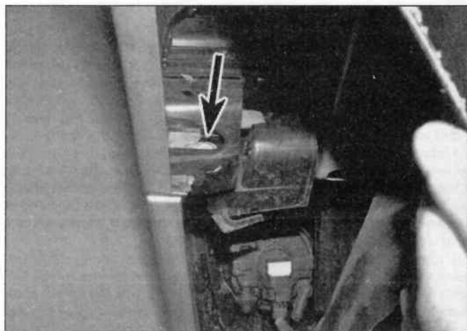
6.3 Undo the bumper-to-wing screws (arrowed)
