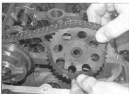
6.25 Refit the camshaft sprockets
