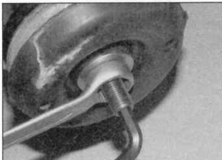
5.2 Slacken the top nut whilst retaining the rod with an Allen key
