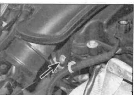
4.5b ... and the front mounting bolt (arrowed) ...
