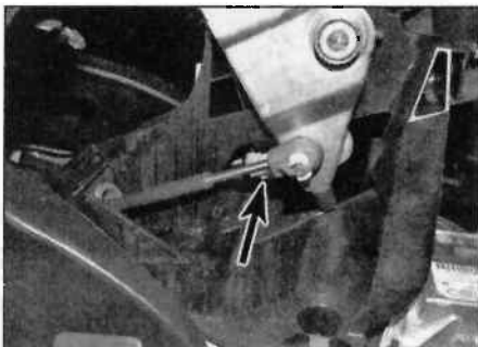
3.20 Release the locking clip (arrowed)
