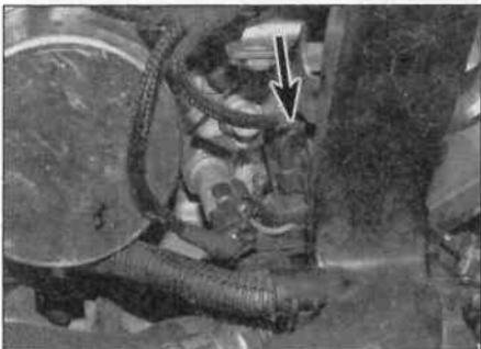
7.5a Temperature sensor wiring connector (arrowed) – petrol engines
