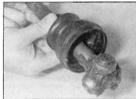
3.37b Slide the gaiter off the end of the driveshaft
