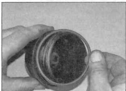
3.11a Renew the O-ring seal to the cover ...
