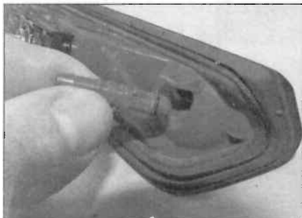
16.19a Pull the washer jet from the light unit – Hatchback
