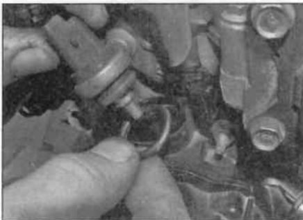
7.6b ... and pull out the sensor and seal from the housing
