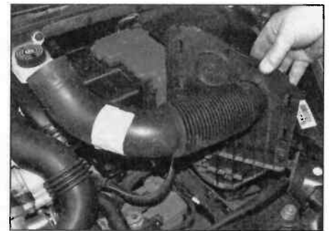
4.3b ... and remove the air ducting
