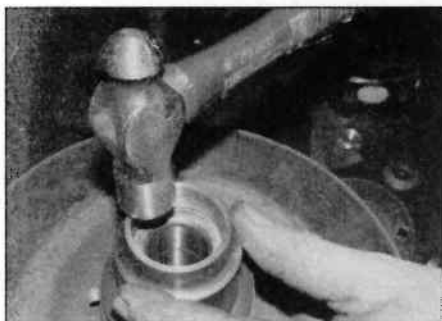
11.9b ... then tap it gently to start it into the hub
