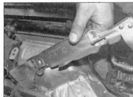
21.10 Unbolt the upper heat shield
