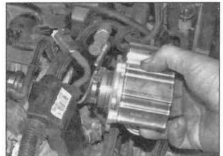
11.6 Remove the fuel pump from the cylinder head
