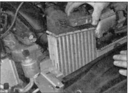
20.7a Withdraw the intercooler out from the front panel ...
