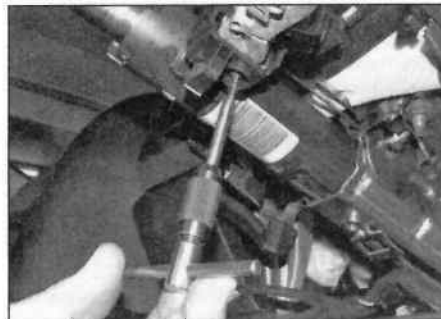
18.6b ... and use an extractor to remove the bolt
