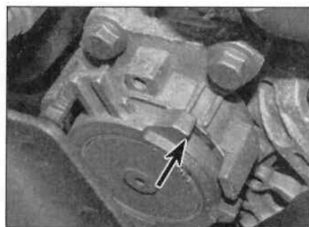
14.5 The alignment lug (arrowed) must be between the two lines on the housing
