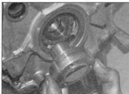
6.14b ... and then withdraw the hub
