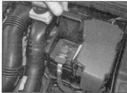
4.4a Open the cover to access the battery terminal ...
