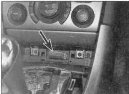
9.9 Vehicle diagnostic plug connector (arrowed)
