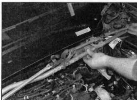
14.7 Remove the wiper linkage from the bulkhead
