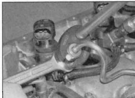
11.19 Tighten the high-pressure pipe union nuts using a crow-foot adapter
