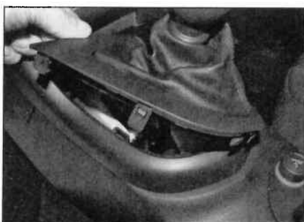
26.1 On manual transmission models, prise up the gear lever gaiter trim
