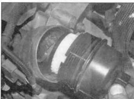
3.11d ... and refit the oil filter and cover
