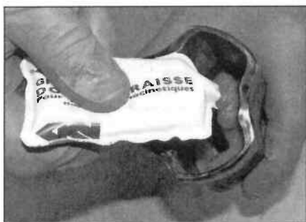
3.27a Pack the outer joint with grease ...
