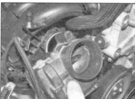
14.4b ... then remove the throttle housing from the manifold and recover the sealing ring
