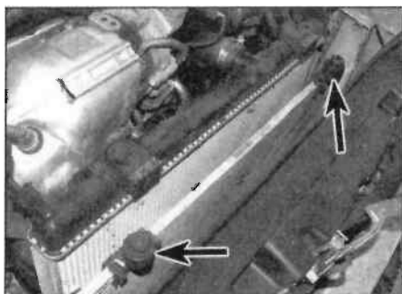
12.16 Make sure the rubber mountings are fitted securely
