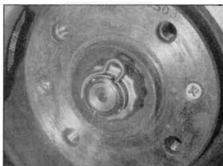
2.23b ... and secure it in position with the R-clip
