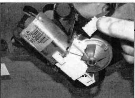
15.4 Disconnect the wiring plug connector ...
