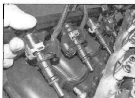
15.6 ... then withdraw the fuel rail and injectors
