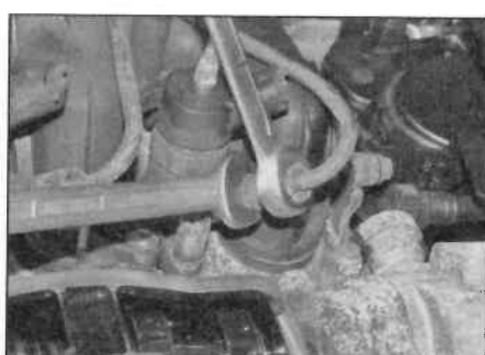
11.8 Use a second spanner to counterhold the high-pressure pipe union nuts
