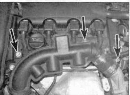
21.8a ... undo the two mounting bolts and slacken the retaining clip (arrowed) ...
