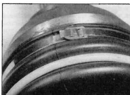
3.11j ... then fold the buckle firmly down onto the clip to secure the clip in position
