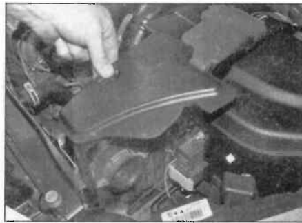
4.3a Release the securing clips ...
