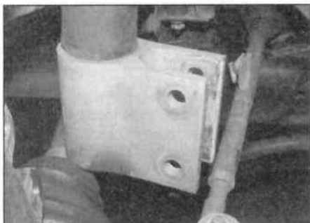
2.8c Rotate the base of the strut 90° towards the rear to minimise any chance of damaging the driveshaft gaiter
