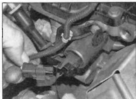
8.15a Disconnect the exhaust electrovalve connector ...
