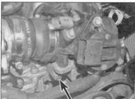
4.7c ... undo the bolt on the end (arrowed) ...
