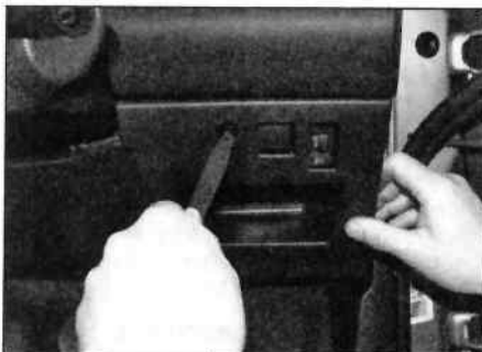
27.4a Turn the securing clip ...
