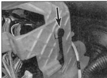
23.6 ... then slide the unit downwards (arrow) ...
