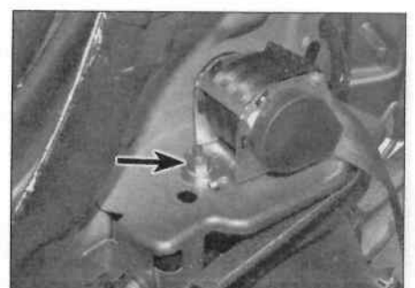
24.9b ... and undo the seat belt reel mounting nut (arrowed) ...
