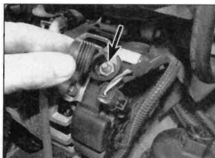
7.4a Remove the rubber cover and undo the securing nut (arrowed) ...
