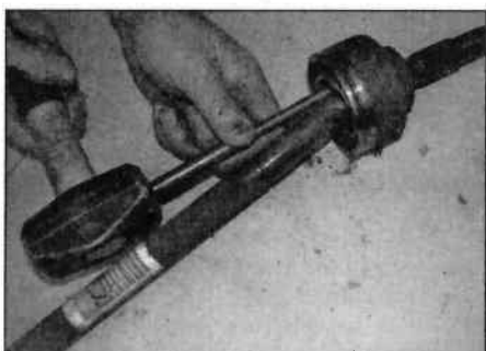
3.4 Using a soft metal drift to release the outer joint
