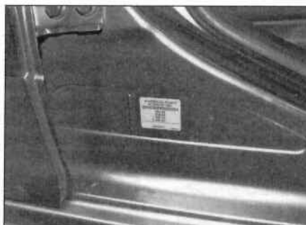
The vehicle identification number (VIN) is also on a label at the bottom of the driver's side B-pillar ...
