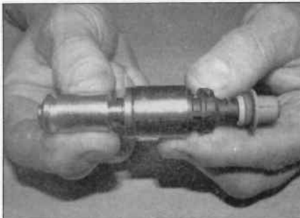
15.21d ... to calibrate the seal, compressing it slightly for fitting
