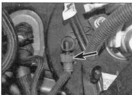
12.6 Release the securing clip (arrowed)
