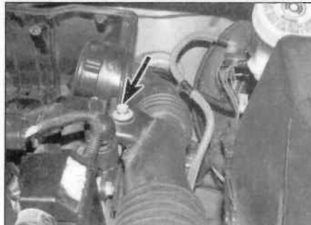
3.5a Undo the retaining bolt (arrowed) ...
