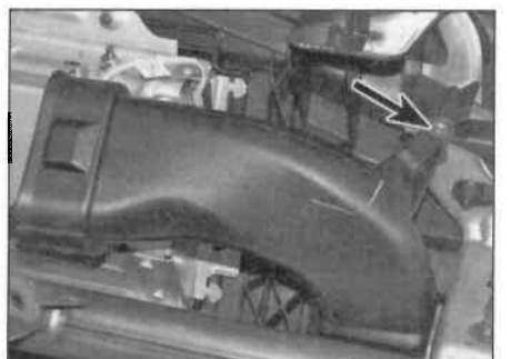
22.9b ... and undo the retaining screw (arrowed) to remove
