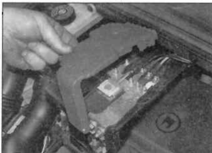
4.5 Unclip the red cover from the top of the battery
