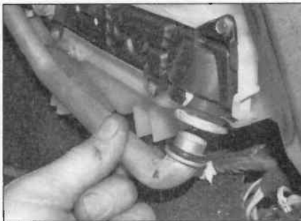
10.20 ... and disconnect the heater pipes from the heater matrix
