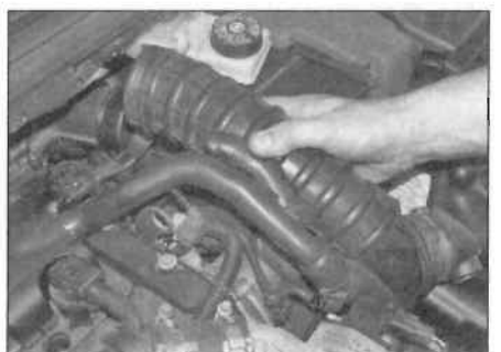
3.11 Remove the air inlet hose
