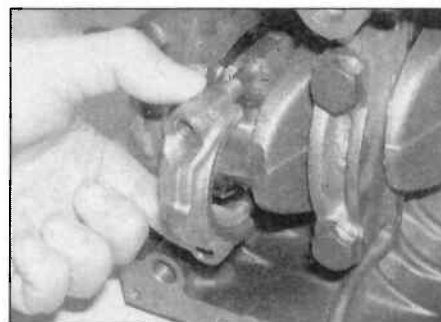
18.8 Fit the big-end bearing cap, ensuring it is fitted the right way around, and screw on the new nuts
