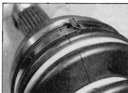
3.11i Fold the clip end underneath the buckle ...
