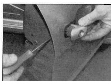
13.6 Slacken the retaining screw and withdraw the lock cylinder/push button
