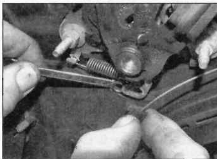
9.4c ... to release the cable retaining clip
