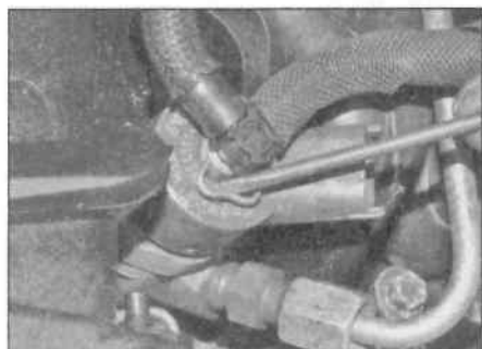
4.9a Prise out the clip and pull the return hose from the top of each injector
