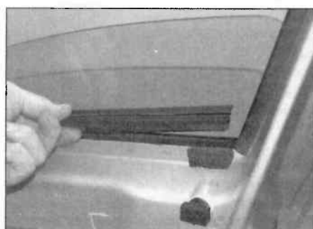
14.1 Carefully prise up the door seal
