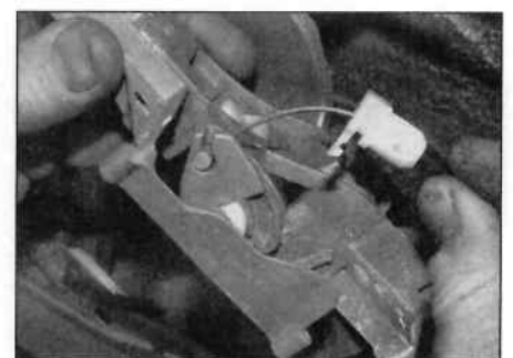
13.15 Release the operating cable from the handle support
