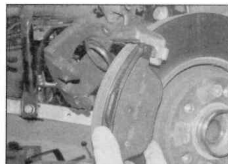
4.23a Fit the new brake pads ...
