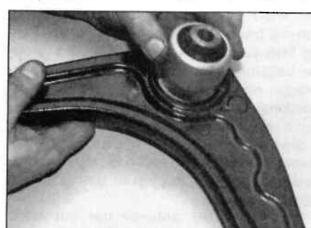
6.7a Press the bushes into the lower arm ...
