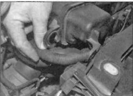
3.7b ... unclip the vent pipe ...
