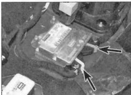
22.15 Lift the locking catches (arrowed) and disconnect the airbag ECU wiring plugs
