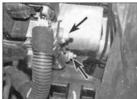
19.11b ... and two lower mounting securing nuts (arrowed)
