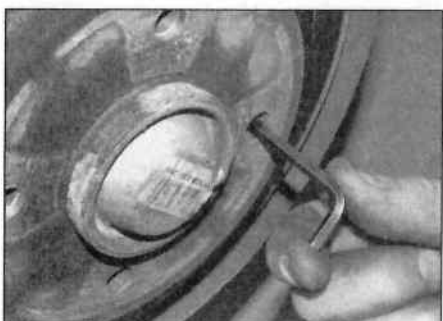
19.26 Insert the tool (arrowed) through one of the roadwheel bolt holes to undo the speed sensor retaining bolt
