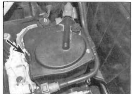
16.8a Release the clip (arrowed) ...
