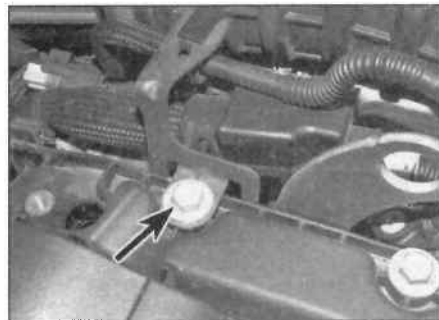
4.13 Undo the wiring bracket retaining nut (arrowed)
