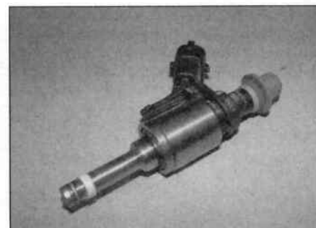
15.21b ... to fit the new combustion seal on the injector ...
