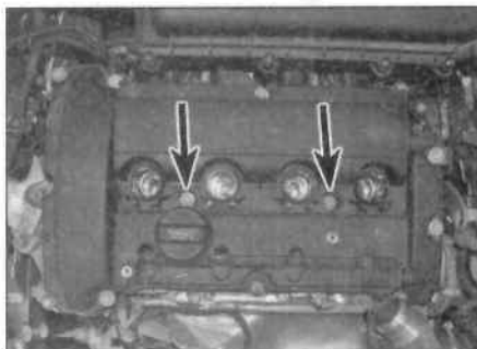
4.12 Two inner cylinder head cover retaining bolts (arrowed)
