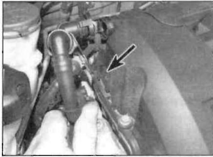
4.9 Release the clip from the camshaft cover
