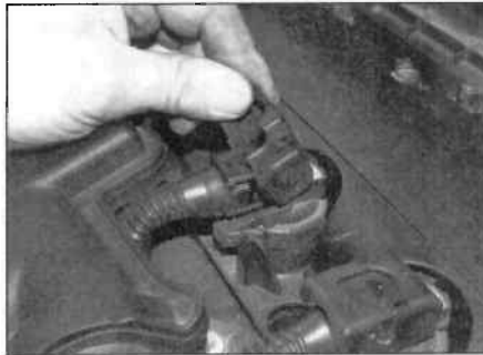
B Check that the ignition system (as applicable) wiring connectors are securely connected (turbo petrol model shown).
