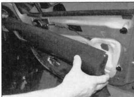
12.9 Lift and remove the door trim panel
