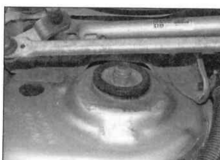
4.6a Undo the strut upper mounting nut ...
