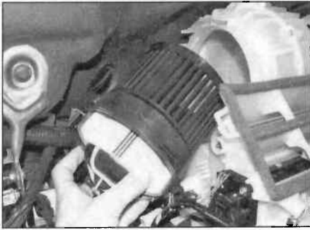
10.33b ... and rotate the motor anti-clockwise to remove
