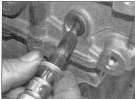
6.13a Remove the upper guide securing bolts ...
