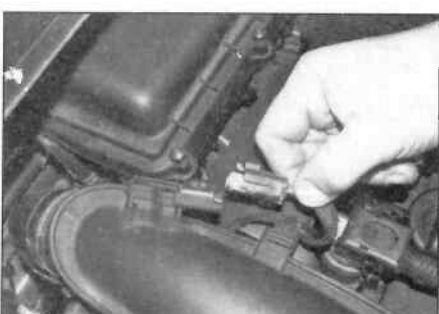
4.4a Disconnect the sensor wiring connector ...
