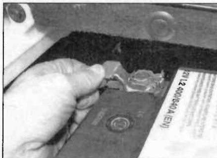
4.8 Lift up the green quick-release lever and disconnect the negative lead
