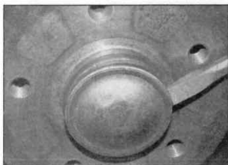
7.5 Remove the cap from the disc/hub ...
