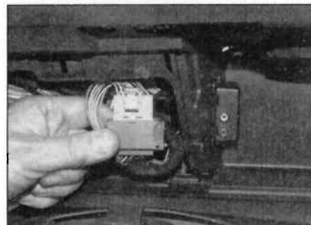
27.12b ... and unclip the wiring connector securing clip
