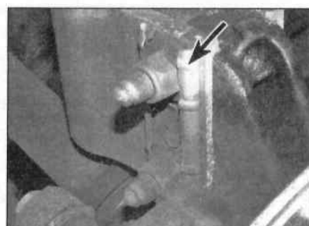
2.8b On later models the bolts go in from the rear and a locking clip (arrowed) is fitted to the securing nuts
