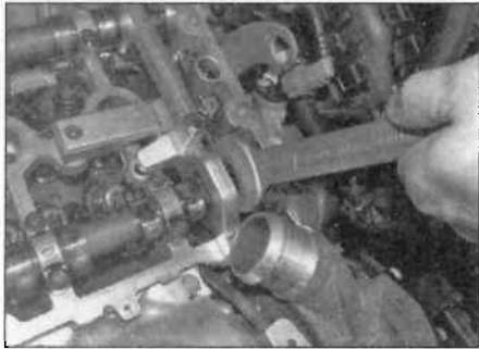
6.8a Hold the camshafts in position ...
