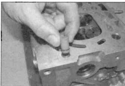
7.9b ... and the camshaft oil supply non-return valve will be ejected from the underside of the cylinder head
