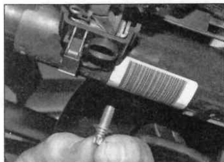
18.8 Fit the new shear bolt – tighten until the head shears off
