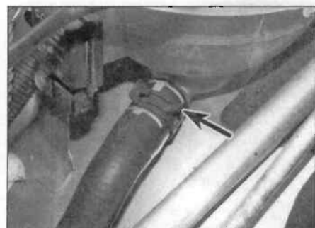
3.5 Release the coolant hose securing clip (arrowed)
