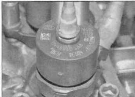
11.11 Note the injector classification number
