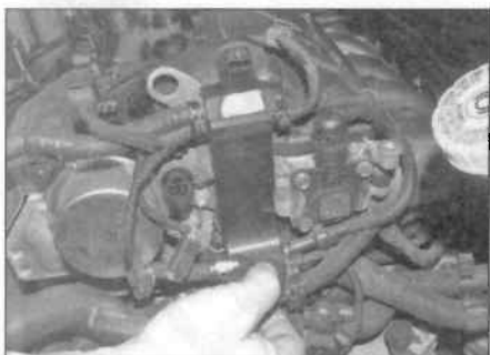
5.4 Unclip the wiring loom mounting bracket
