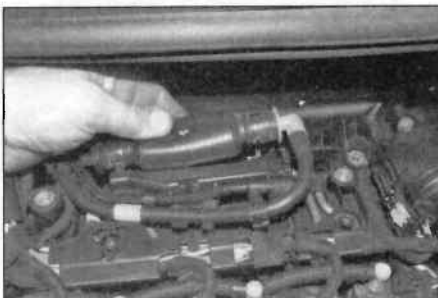
3.1 Operate the hand-priming pump until fuel clear of bubbles appears in the fuel pipe (arrowed)
