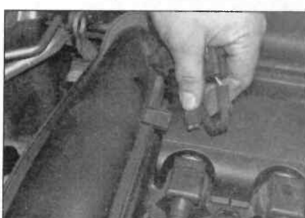
4.4b ... and unclip the wiring loom
