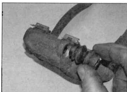
4.8b ... and the guide pin gaiters
