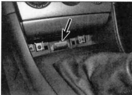
1.3 Vehicle diagnostic plug connector (arrowed)
