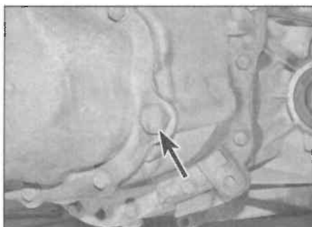
17.4 Fluid level/filler plug (arrowed) – BE4/5 transmission
