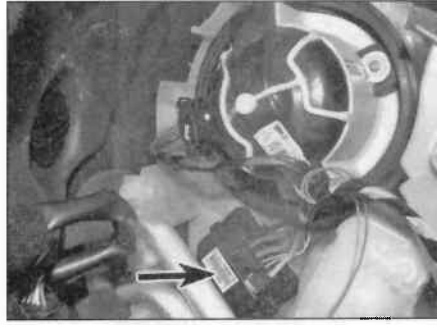
10.35 Location of blower motor resistor (arrowed)
