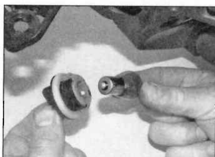
5.26 ... then press in the bulb and rotate it anti-clockwise to remove it
