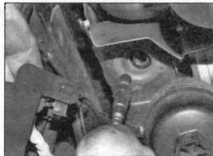
2.12 Removing the upper sensor
