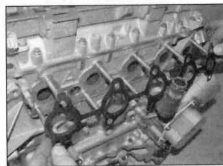
14.2b Recover the manifold gasket
