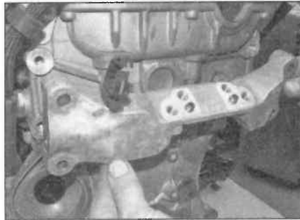
13.7 Remove the engine mounting bracket
