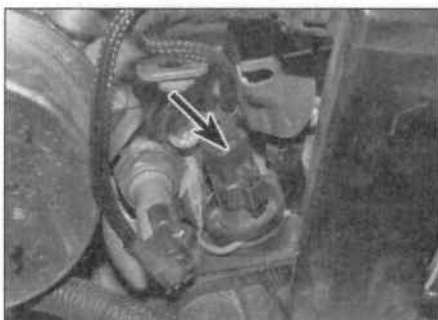
5.5a Disconnect the temperature sensor wiring connector (arrowed) ...
