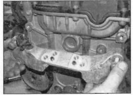
6.13 Remove the engine mounting bracket
