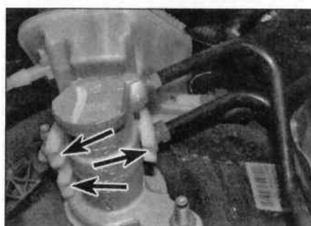
10.8 Release the plastic clips (arrowed) to remove the reservoir
