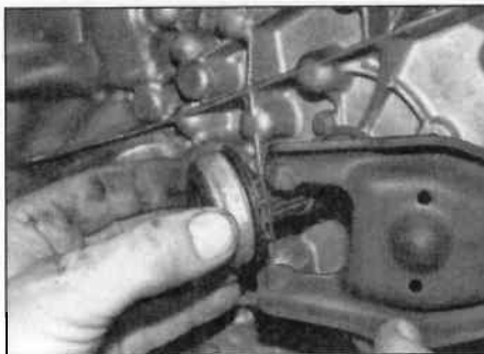
7.3 ... disengage the release bearing as the fork is removed
