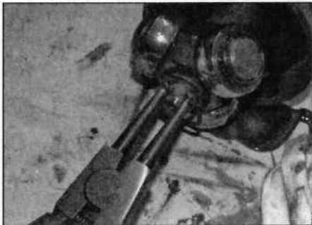
3.19a Release the circlip ...
