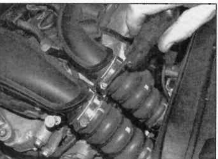
21.7 Slacken the hose retaining clip ...
