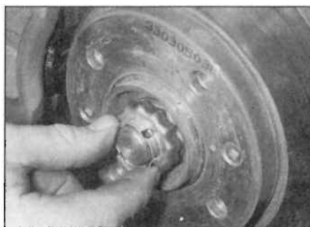
2.23a Tighten the driveshaft nut to the specified torque, then refit the locking cap ...
