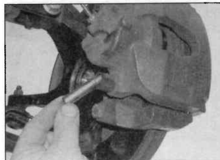
4.18 Unscrew the guide pins
