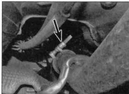
18.14 Flexible pipe-to-middle section retaining clamp (arrowed)
