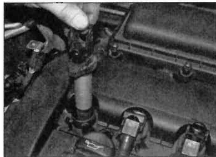
3.5 ... and withdraw the ignition coil
