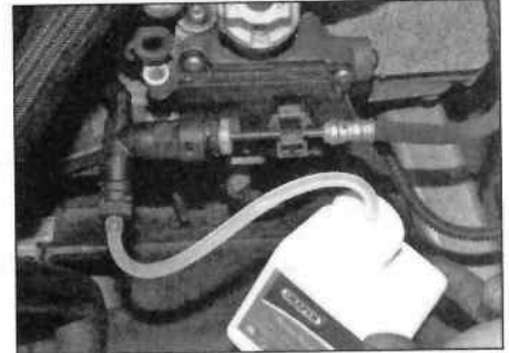
2.6 Air bleed bottle connected to bleed screw
