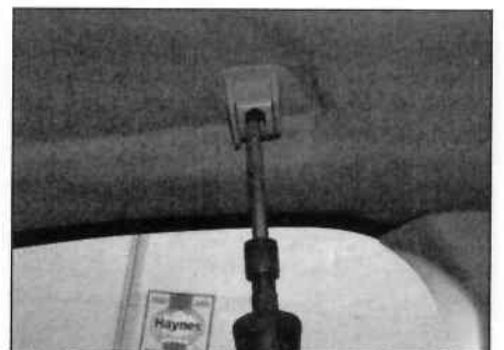
25.88 Undo the retaining screw to remove the hinge clip
