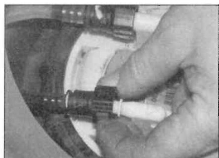
8.4 Depress the release button and disconnect the fuel pipe
