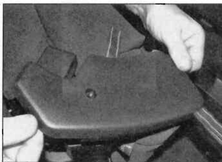
24.22a Remove the seat side trim ...
