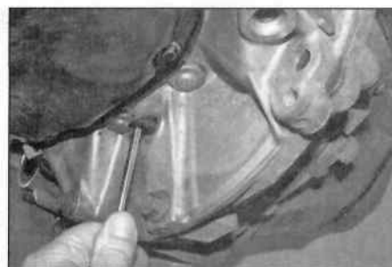
3.2 When the timing hole is aligned with the hole in the flywheel, the pin can be inserted to lock the crankshaft in position
