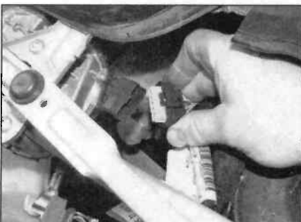
14.5 Disconnect the wiper motor wiring plug
