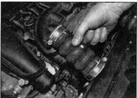
7.5 Remove the intercooler hoses – turbo models
