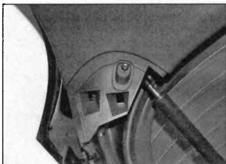
25.69 Undo the lower trim upper retaining screws
