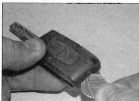
17.6a Twist the coin in the slot provided ...
