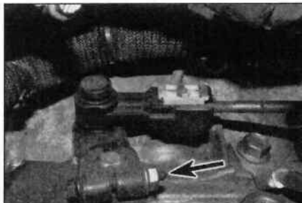
6.12 Unscrew the nut and clamp bolt (arrowed) and free the selector lever from the transmission shaft
