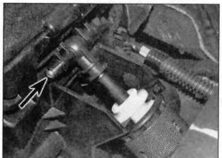
4.8a Release the pivot pin (arrowed) ...
