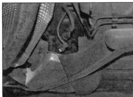
12.10 Additive tank fitted to diesel models
