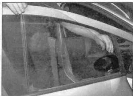
14.3b ... and withdraw the window glass out from the door
