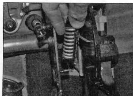
5.5 Withdraw the spring assembly out from the pedal
