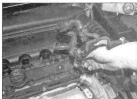
4.8b ... and remove the wiring loom from the cylinder head cover
