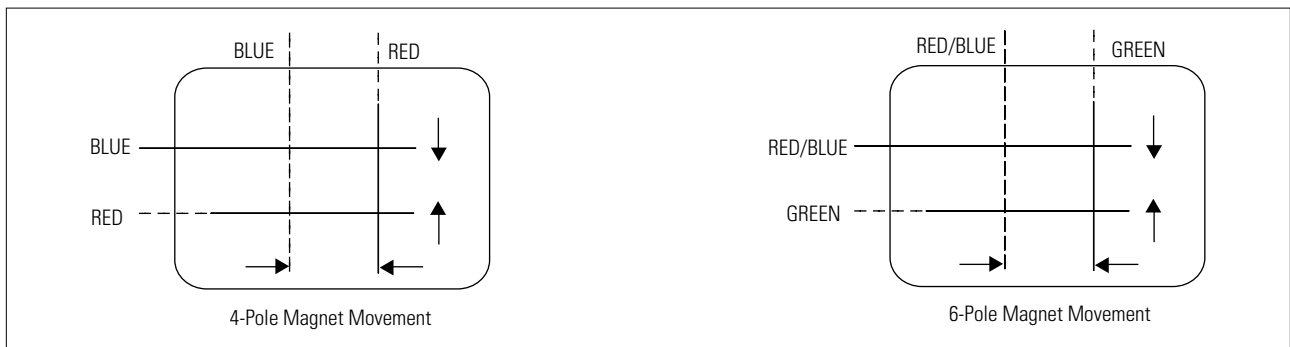
Fig. 4-5 Center Convergence Adjustment
