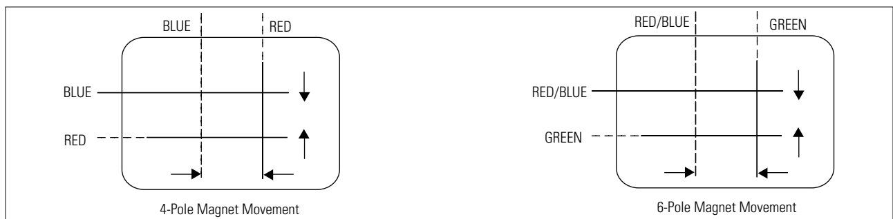
Fig 5-3 Center Convergence Adjustment
