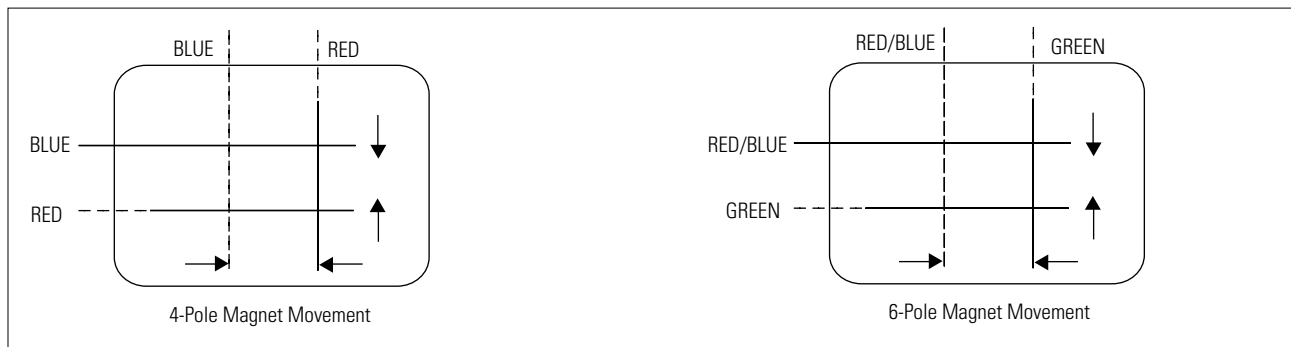
Fig. 4-5 Center Convergence Adjustment
