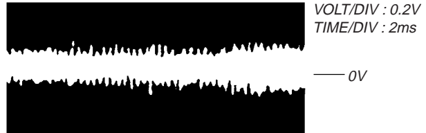
high tracking gain (high fundamental wave than for low gain)
