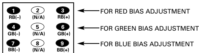
Figure 5. Remote Control Number keys' functions in Service Menu NO. A8 (No Vertical Sweep)
