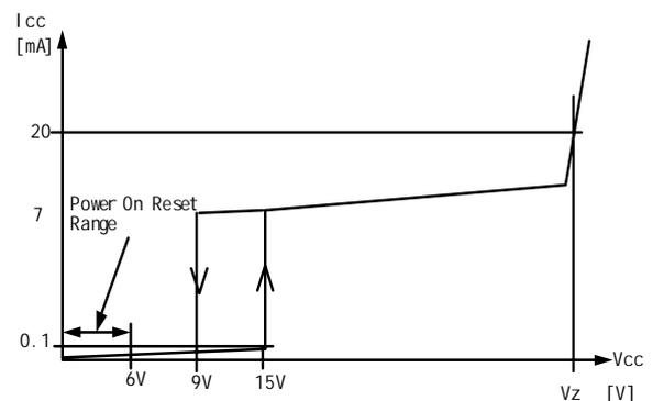
Figure 2. Variation of Icc according to Vcc
