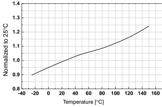
Figure 13. Feedback Sink Current vs. Temp.
