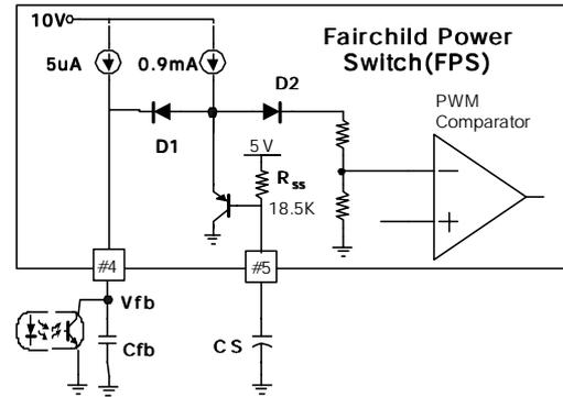
Figure 5. Soft Start Circuit
