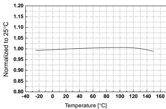
Figure 11. SoftStart Voltage vs. Temp.
