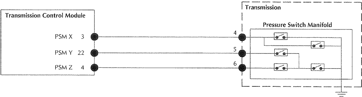
Figure 2. Pressure Switch Circuits
