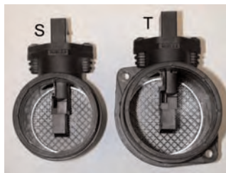
Venturi Mass Air Sensor
