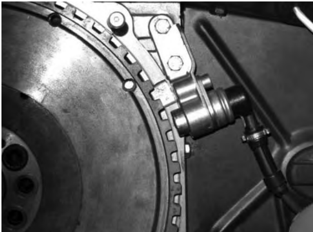
Flywheel With Sensor Ring and Inductive Sensor
