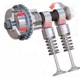
Vane-type VarioCam adjuster on the intake camshaft
