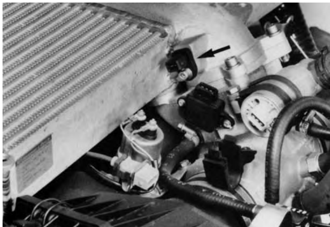
Intake Air temperature Sensor (Black Arrow)
