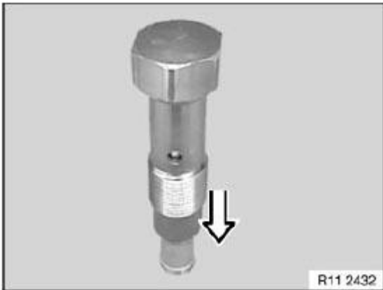
Fig. 209: Identifying Chain Tensioner Piston Courtesy of BMW OF NORTH AMERICA, INC.
