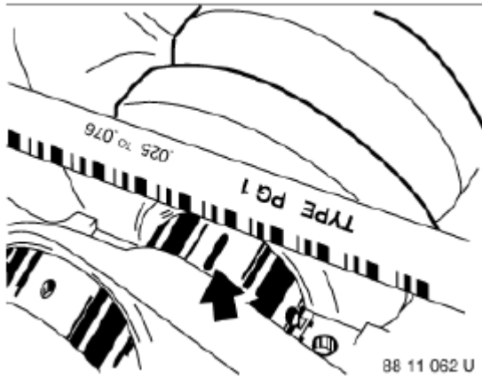
Fig. 124: Checking Radial Clearance At Width Of Flattened Plastic Thread (Plastigage)
