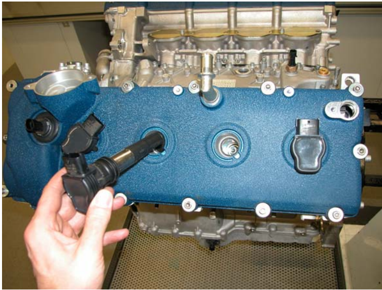
Remove the ignition coils
