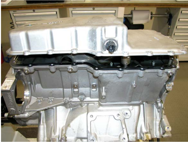
Remove the oil sump
