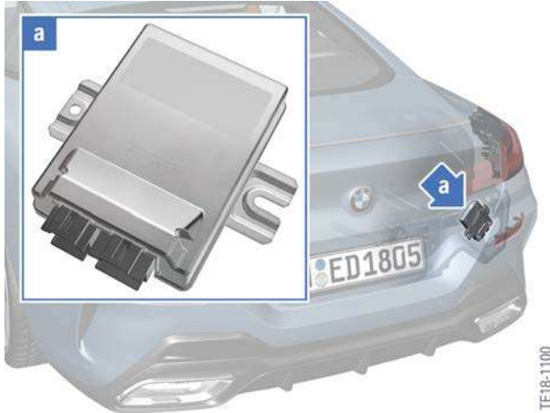
Regulated rear axle differential lock
