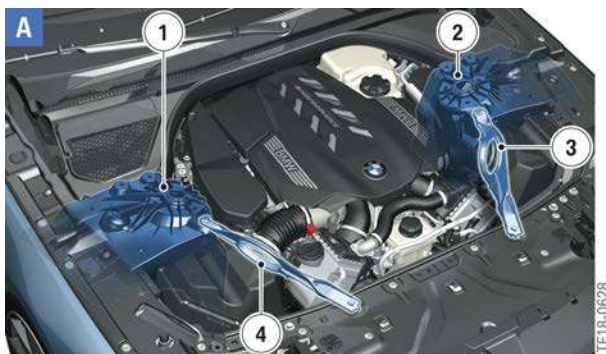
Overview of front-end struts G15
