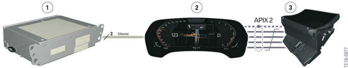
G15 connection of Head-Up Display
