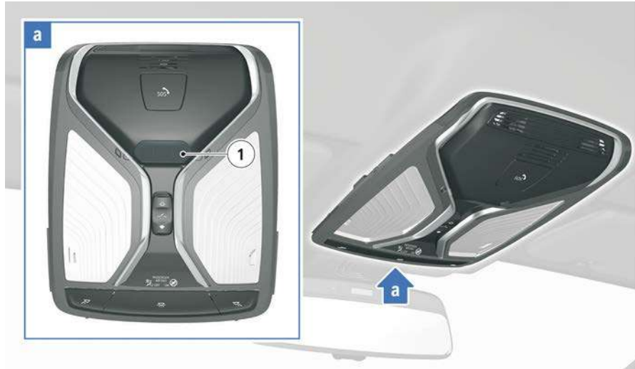
G15 installation location, gesture recognition camera
