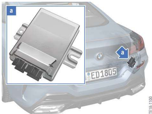
G15 mounting orientation of GHAS
