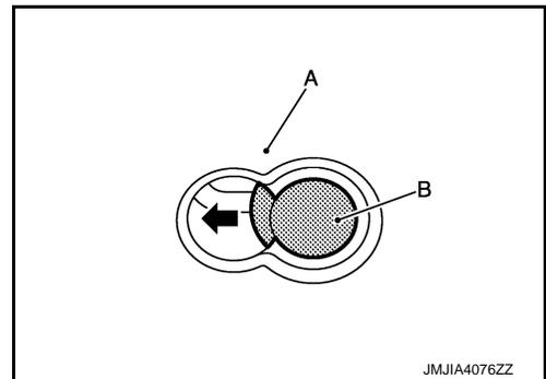
5. Use pincers, etc., to press up pawls as shown by the arrows in the figure, and remove headrest holder from seatback.
