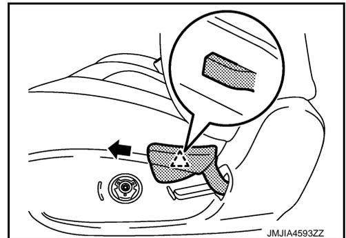
4. Pull seat cushion outer finisher toward seat front. Disengage pawls and metal clips. Slide seat cushion outer finisher toward seat front. Remove seat cushion outer finisher.
