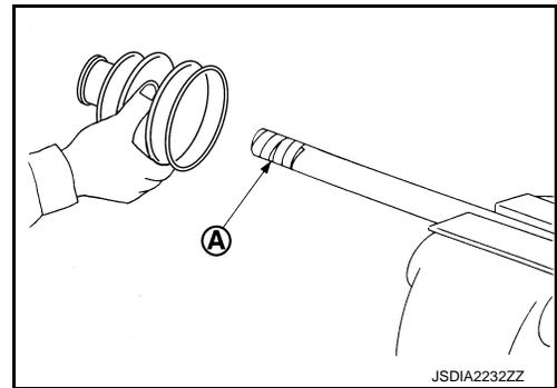
5. Install boot securely into grooves (indicated by "\*" marks) shown in the figure.
