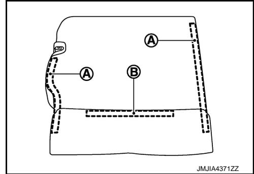
4. Slide and align the clips (B) to the holes on the seatback as shown in the figure, and then remove the seatback board (A).
