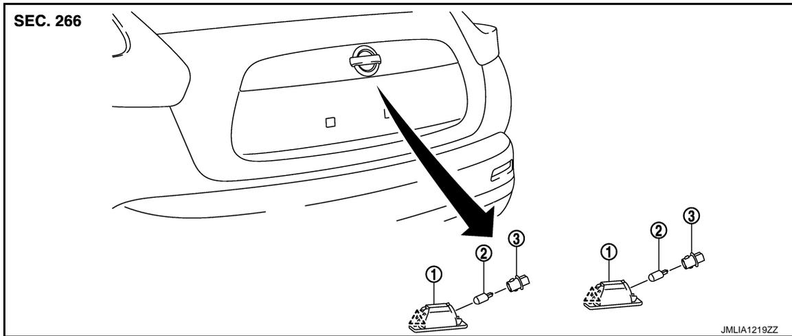
1. License plate lamp housing assembly      2. Bulb      3. License plate lamp bulb socket
