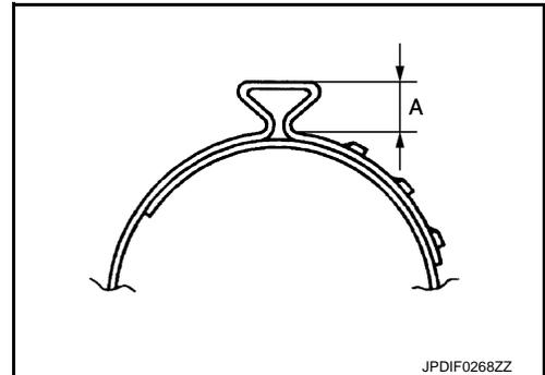
12. Check that displacement does not occur when boot is rotated with the joint sub-assembly and shaft fixed.
