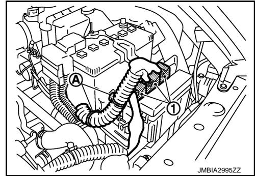
7. Disengage pawl using a flat-bladed screwdriver (A). Remove F/L-fuse holder.
