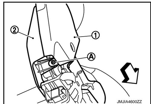
4. Remove fixing screws. Pull seat cushion inner finisher toward seat front. Disengage pawls. Remove seat cushion inner finisher.
