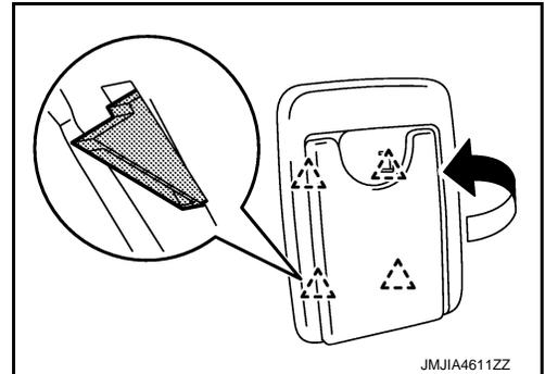
3. Open seatback fastener (A) and remove seatback retainer (B).
