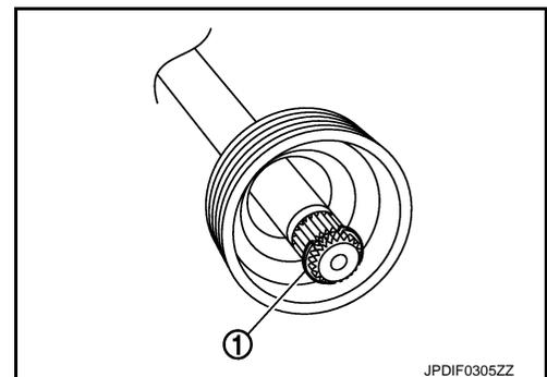
6. Align both center axes of the shaft edge and joint sub-assembly. Then assemble shaft with joint sub-assembly holding circular clip.
