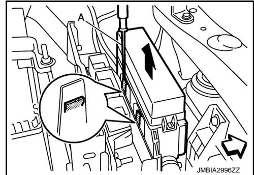
8. Move F/L-fuse holder and harness to a location where they do not inhibit work.
