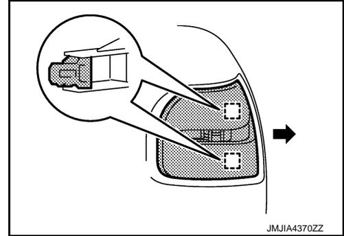
2. Pull tether cover in direction indicated by the arrow as shown in the figure. Remove tether cover.
