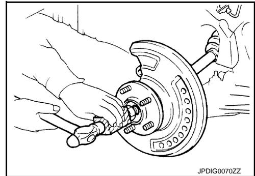
8. Remove wheel hub lock nut.
