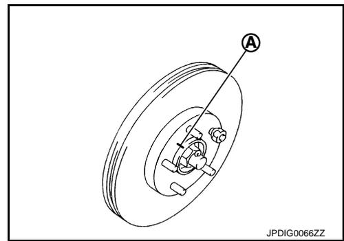
6. Remove cotter pin, and adjusting cap, and then loosen wheel hub lock nut, using a hub lock nut wrench (A) (SST: KV40104000).
