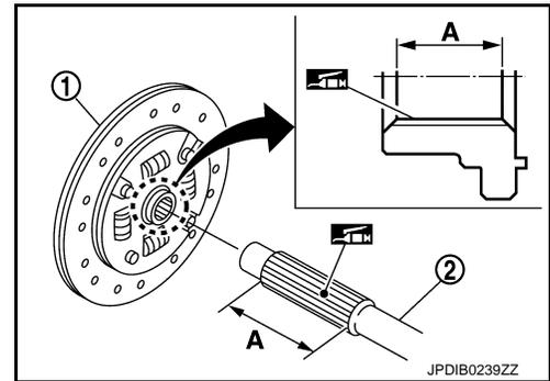
3. Install clutch disc, using a clutch aligner (A) [Commercial service tool].
