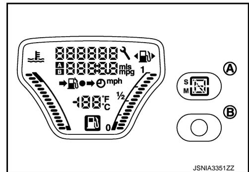
7. Each meter activates by pressing the meter control switch.
