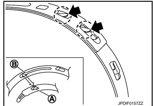
2. Pinch projection on the band with suitable pliers to tighten band.
