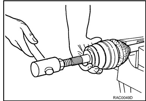
9. Install the boot securely into grooves (indicated by "\*" marks) shown in the figure.
