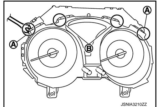
3. Pull the front cover straight to remove it from the meter control unit assembly.
