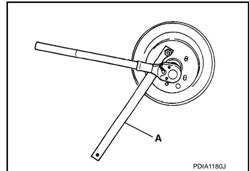
7. Patch wheel hub lock nut with a piece of wood. Hammer the wood to disengage wheel hub assembly from drive shaft.
