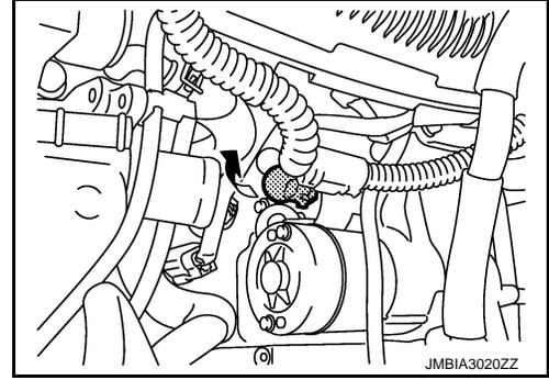
8. Remove "B" terminal nut and "B" terminal harness.
