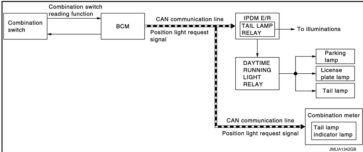
**PARKING, LICENSE PLATE AND TAIL LAMP SYSTEM (WITH DTRL) : System Description**
