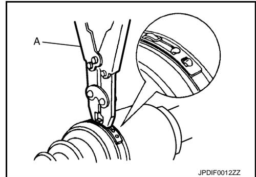
• Secure boot band so that dimension (A) meets the specification as shown in the figure.
