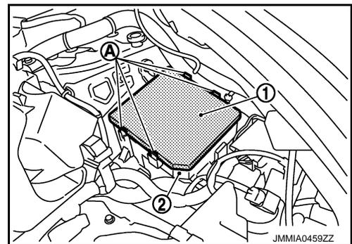
4. Remove IPDM E/R cover B mounting nuts (A).
