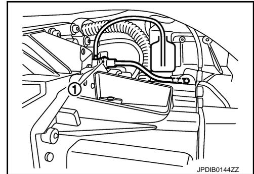
2. Press the lock pin (1) into the bleeding connector (2), and maintain the position.
