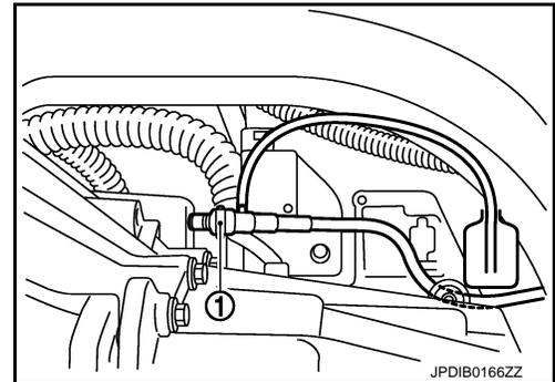
2. Press the lock pin (1) into the bleeding connector (2), and maintain the position.
