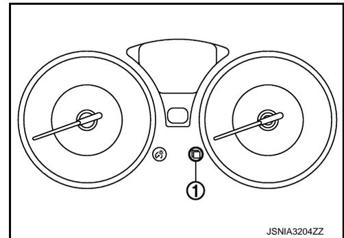
6. The combination meter is turned to self-diagnosis mode. All of the segments of engine coolant temperature gauge, fuel gauge, odo/trip meter, shift position indicator (A) for CVT models and information display illuminate.
