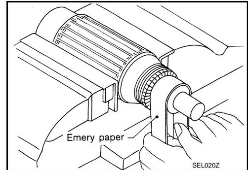
4. Check diameter of commutator.
