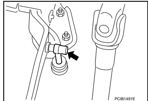
7. Pull up the lock pin (1) from connector of master cylinder (2) and separate clutch tube (3).
