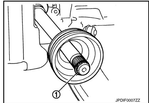
7. Install joint sub-assembly (1) to shaft using plastic hammer.
