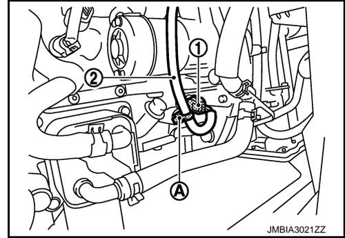
12. Remove starter motor mounting bolts.
