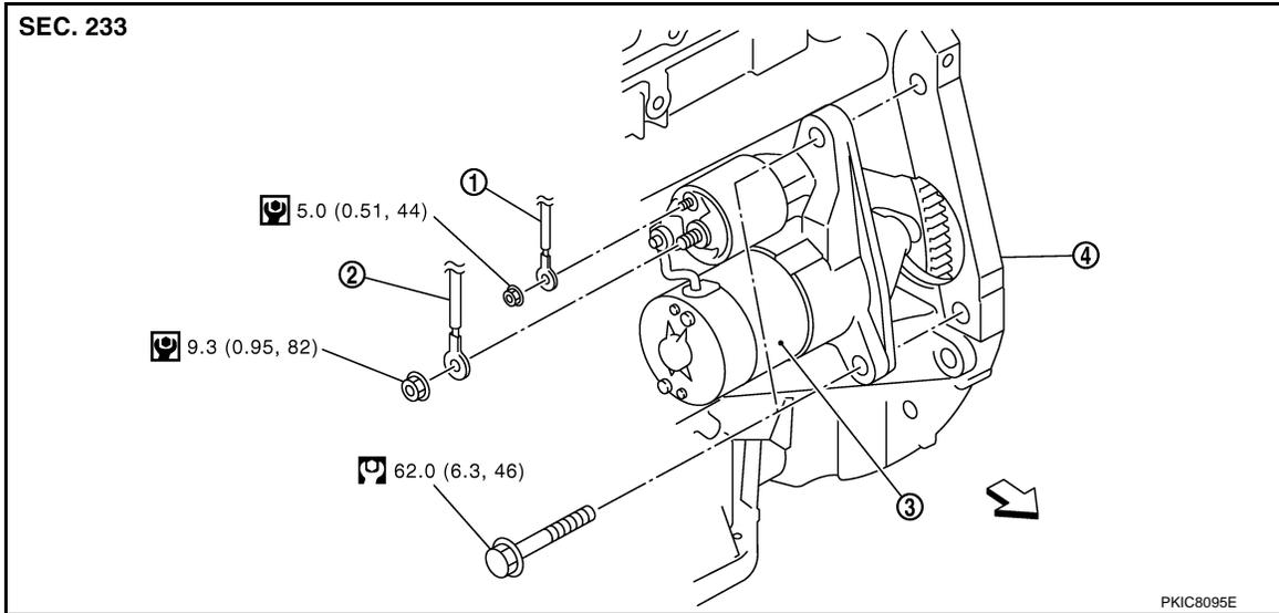
1. "S" terminal harness                      2. "B" terminal harness                      3. Starter motor
