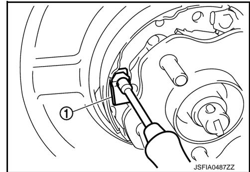
7. Press the rear cable spring (1) against spring tension to remove rear cable (3) from the clamp (A) of toggle lever (2).
