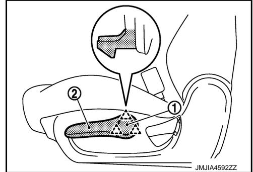
3. Disengage pawl using a screwdriver while pulling reclining lever knob. Slide reclining lever knob toward seat front and remove it.
