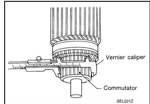
5. Check depth of insulating mold from commutator surface.
