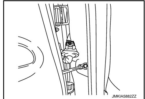
3. Remove mounting bolt of door check link on the vehicle.
