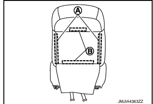
4. Remove side air bag module harness fixing clamps from seat frame & adjuster assembly.
