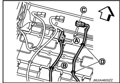
3. Open seatback fastener (A) and remove seatback retainer (B).
