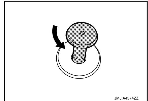
2. Push up seatback lock knob finisher while pressing pawls indicated by arrows as shown in the figure. Remove seatback lock finisher from seatback.
