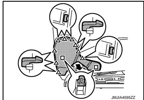
4. Remove seat cushion retainer from seat frame & adjuster assembly. Remove seat cushion trim and seat cushion pad.
