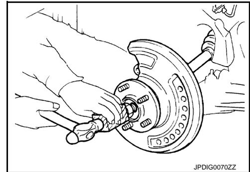
8. Remove wheel hub lock nut.
