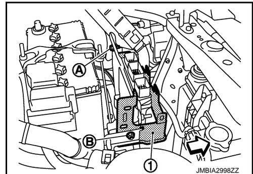
11. Remove mounting bolt (A), and then move water hose (1) and heater thermostat (2) to a location where they do not inhibit work (CVT models).
