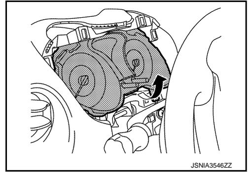
5. Remove connector to remove the combination meter.
