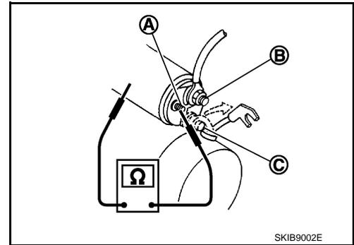
2. Continuity test [between "S" terminal (A) and "M" terminal (C)]
