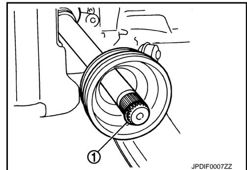
7. Install joint sub-assembly (1) to shaft using plastic hammer.
