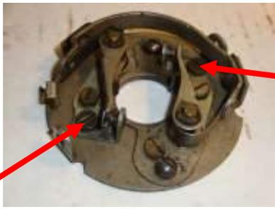
Base plate. Remove points by undoing marked screws (red arrows). The upper and lower screws on the right hold the base plate and should not be touched
