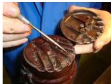
Exterior of Delco cap showing impaling spikes. Seal cable exits with silicone to prevent water ingress
