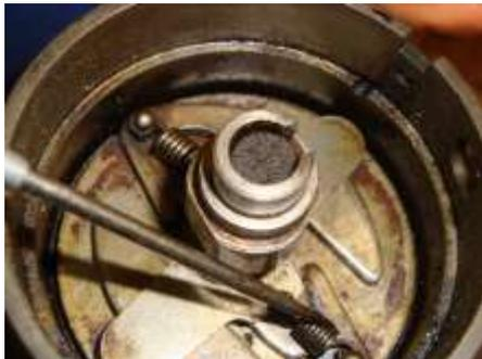
Automatic advance and retard weights and springs. Check for breakage or seizure
