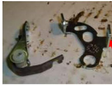
A new set of points. It is necessary to saw off the square lug on the fixed contact
