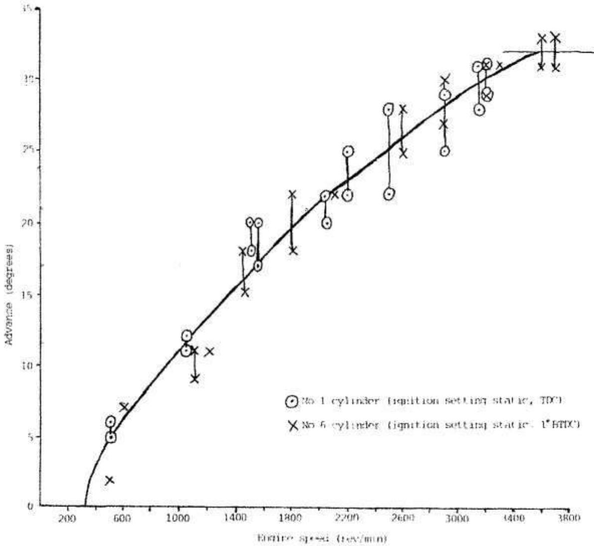
Timing measurements with Delco-Remy unit (650 KB). Vertical lines represent ignition scatter. Governor range 33° approximately (at crankshaft). Cut-off speed 1800 rev/min (3600 rev/min at crankshaft). Static ignition settings measured using small lamp across points.
