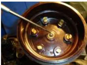
Interior of Delco cap. Check carbon button and brass contacts
