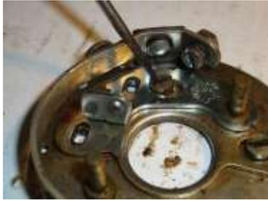
New fixed contact in place. Note adjustment screw
