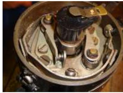
Cap removed showing rotor arm, cam and twin points
