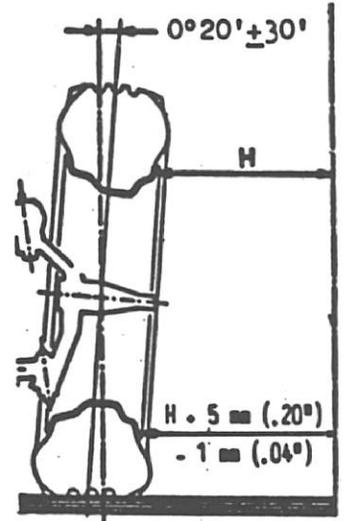
Note - Not adjustable. Check the chassis and suspension arms if necessary.
