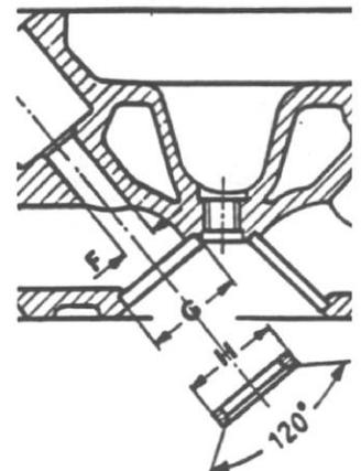
Interference between valve seat insert and recess in cylinder head . . . H-G .100 to .040 mm (.0039 to .0010")
