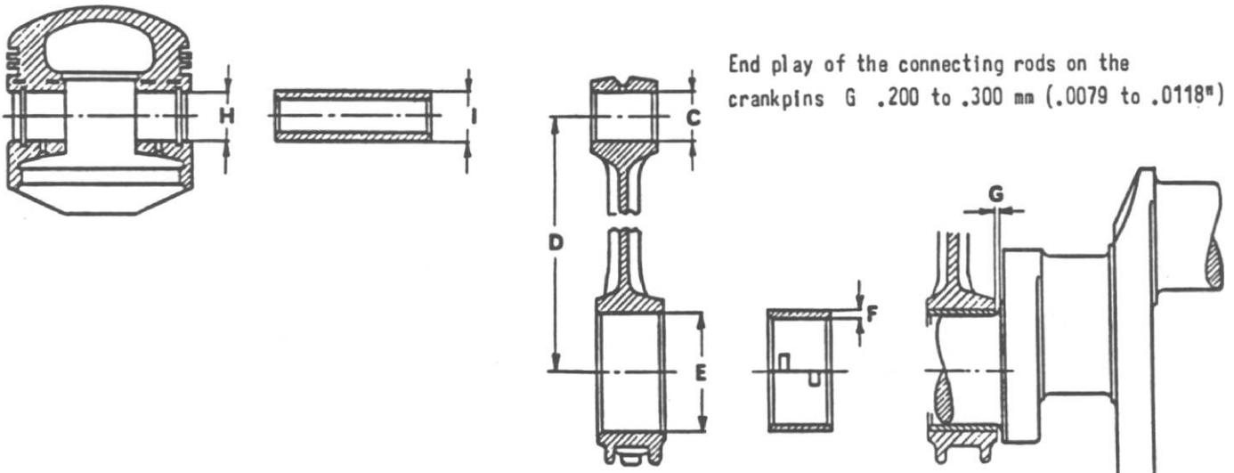
End play of the connecting rods on the crankpins G .200 to .300 mm (.0079 to .0118")
