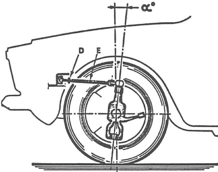
The difference in caster angle between R.H. and L.H. wheel must not exceed  $0^\circ 20'$ .
