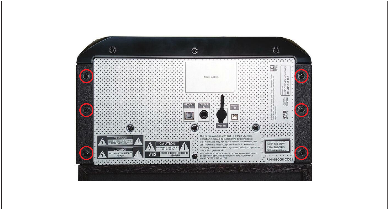
Figure 1. Panel Side L/R disassembly - 1
