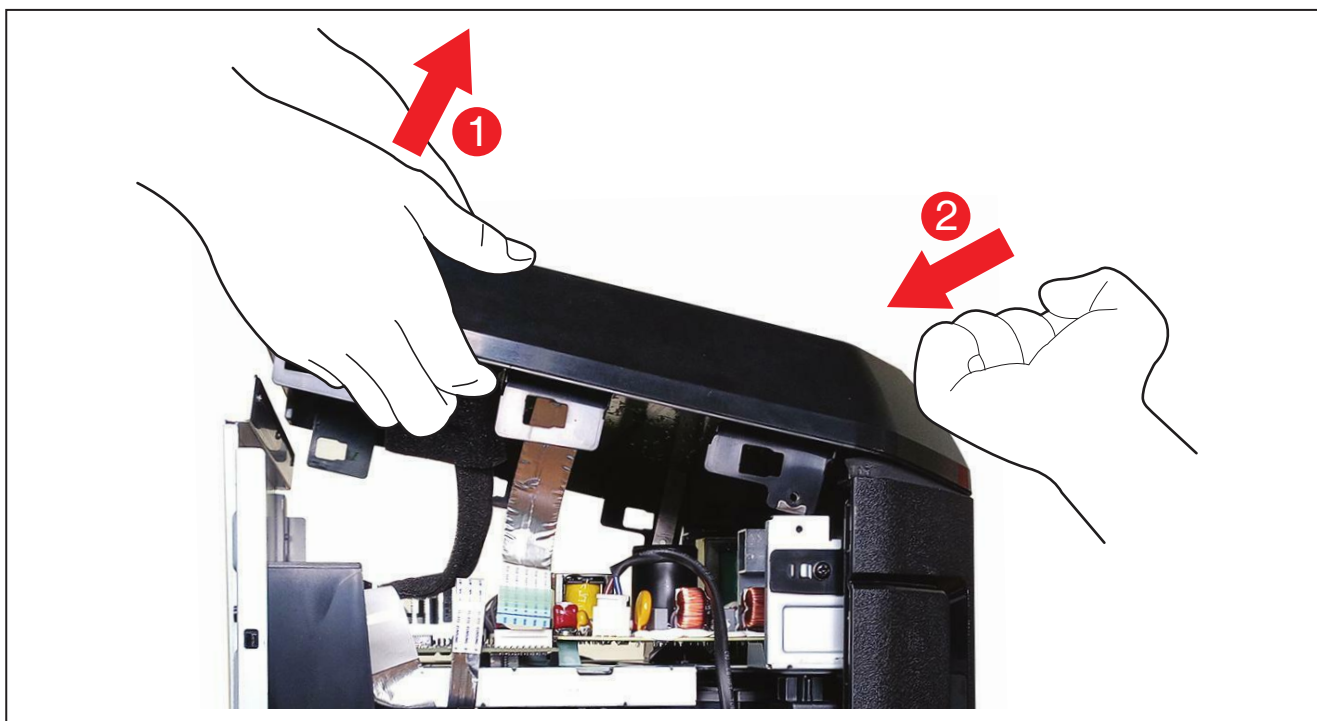
Figure 6. Panel Top disassembly - 3
