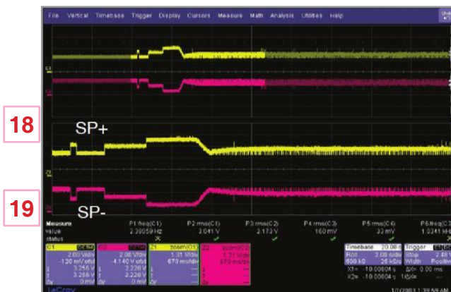
Fig 4-3. SP- & SP+ for Driving SPINDLE Motor (IC400 Pin17, 18)
